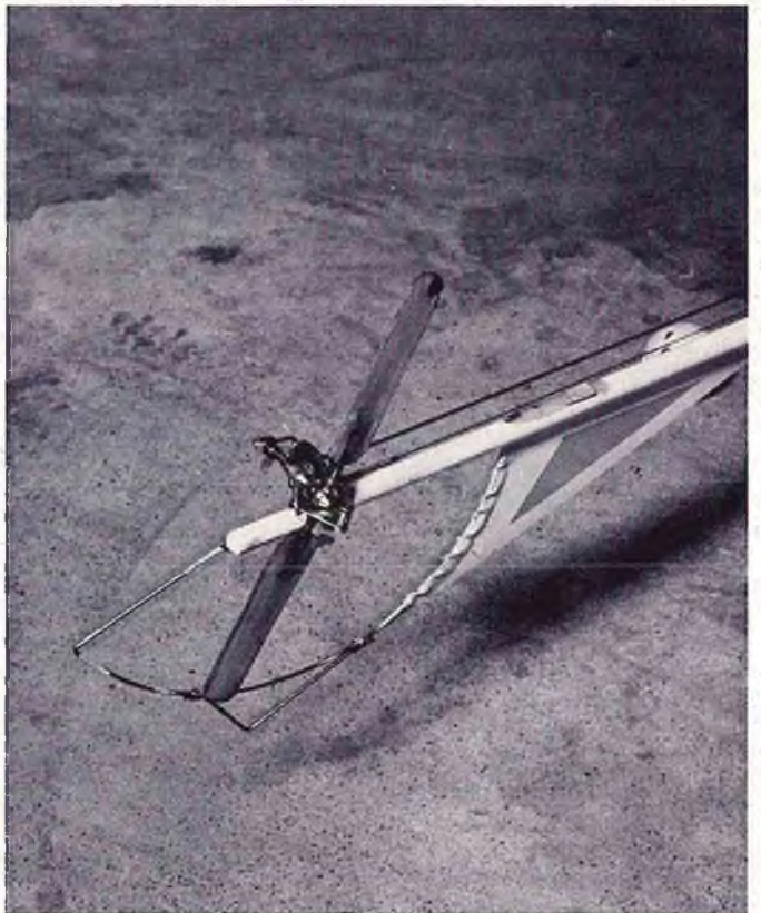
FIGURE 5: Remove horizontal tail, add tail guard, change pitch mechanism.
