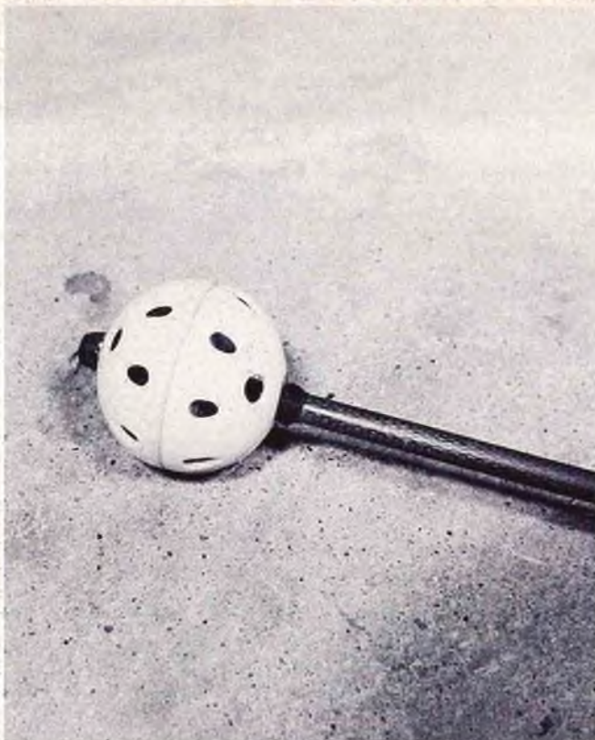
FIGURE 2B: Training golf ball is held on by thread, wrapped and glued to fiberglass arrowshafts. Leave ball face to rotate.
