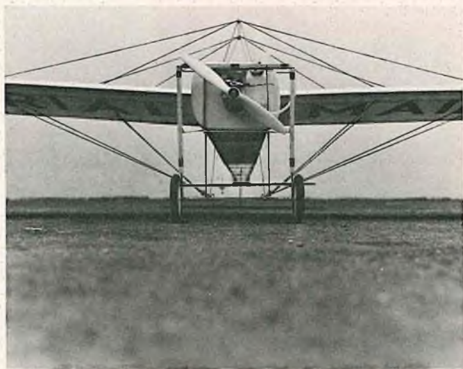
A head-on shot of the Puffin shows a view of the landing gear and rigging arrangement. A little extra effort adds a lot to the overall appearance.
