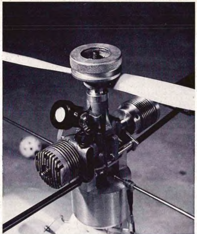
FIGURE 3: Flywheel (6 ounce) attached above prop for mass balance and additional gyroscopic inertia.
