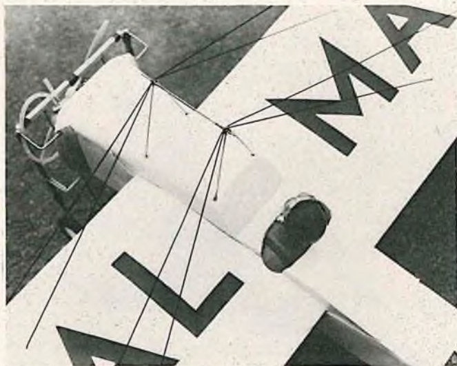
The rigging looks complicated, but takes only a few minutes to install, a few seconds to connect at the field, and adds immensely to the overall appearance.
