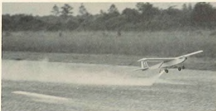
An easily controlled, spectacular boost into the air. JATO is fired at approximately 75% of normal take-off roll.
