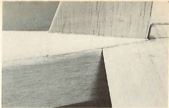
Add 3/4" soft blocks to each side of the fin and carve and sand to blend into the fuselage.
