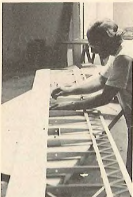
LEFT: The horizontal stabilizer for the Sunrise is being constructed. In the photo above, you can see the vertical stabilizer structure which weighs only four ounces! RIGHT: The photo shows mating wing tips. BELOW: Attaching the landing gear bulkheads.
