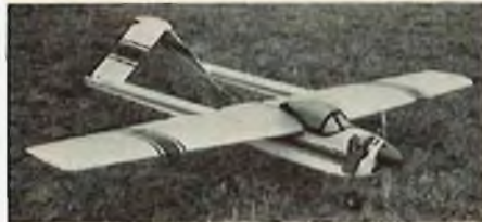
Dean Copeland made this twin-boomed design by sawing off a stock Komander just behind the wing and using the remaining wood for the unusual tail. It flew fine.
