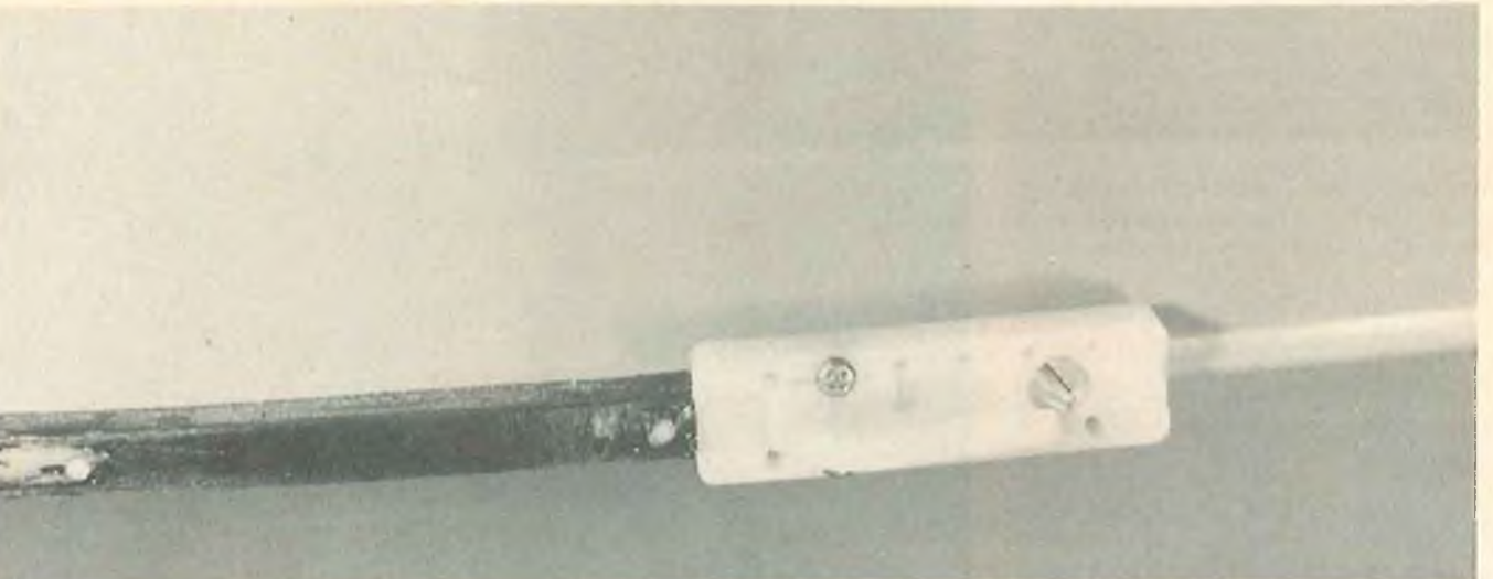
Tow hook and skid detail. The EK-logictrol tow hook is mounted with wood screws rather than using the nut plate that is provided with the tow hook hardware package.
