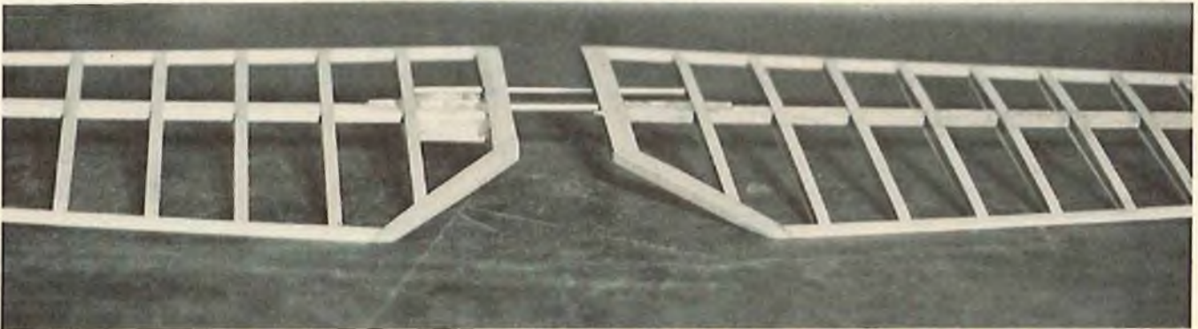
Proper alignment of the connections used in the stabilizer is important. Use 1/16" piano wire for the connector rod and 7/32" diameter brass tubing for the connector tube.
