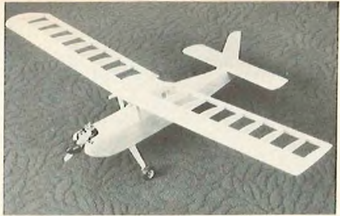
Small Wonder completely framed up ready for covering.
