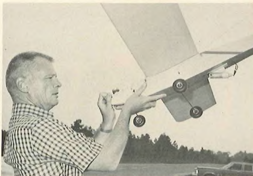
Rocket exhaust temperatures and scant ground clearance restrict this JATO configuration to paved runways.
