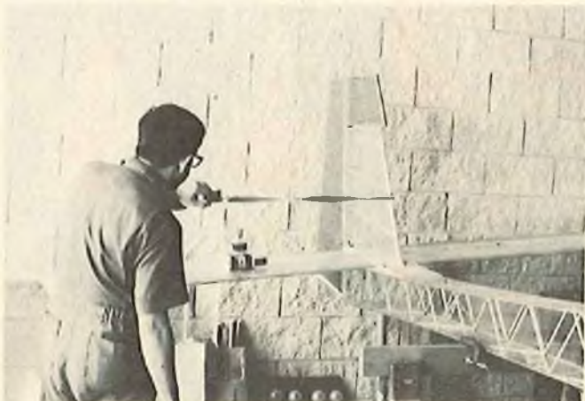
Asymmetrical tail load test.
