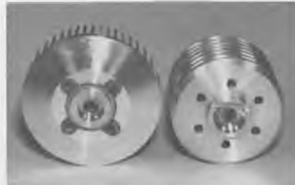
HGK head, on the left, is Heml shaped with squish band. The HB head has a little less compression and is slotted for the piston baffle.
