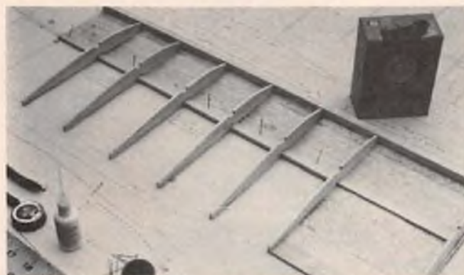
Wing construction is conventional, no tricks. Cyanoacrylate and baking soda good for gluing ribs to bottom sheeting.
