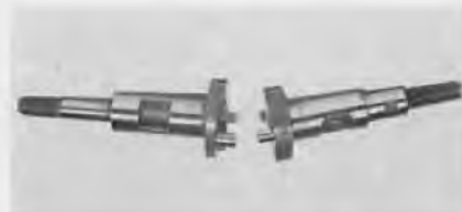
The HB crankshaft, LEFT, is almost identical to the Veco-McCoy cranks. The HGK crank has a smaller bore with a threaded end that screws into the crank.
