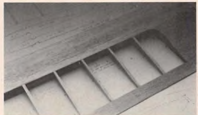
Wing is sheeted with 1/16" C-Grain balsa back to the spars. Cap strips on top only.
