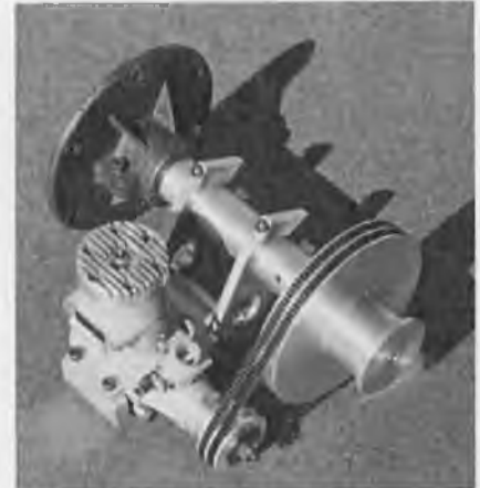
Byron Original's prop unit, equipped with an O.S. .60 FSR. In the Pitts it turns a 20/8 prop.
