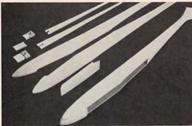
The fuselage is assembled from sheet and blocks. Not shown in photo is the noseblock and bottom block. Shaping is easy with a razor plane.
