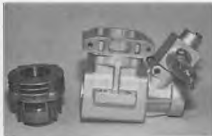
The upper part of the engine, shown on the left, is all one piece aluminum. The Schnuerle intake ports are cast in, as well as the cylinder bore, which is chrome plated.
