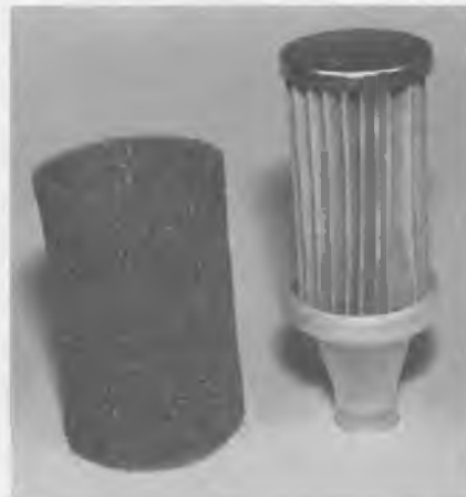
This is probably the ultimate air filter for R/C cars. The HB unit features a paper air filter which is covered with a foam sleeve. Plastic adaptor attaches to carb.
