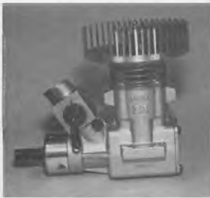
The new HGK engine has been winning a lot of races in Japan. It is Schnuerle ported with a chromed aluminum cylinder.
