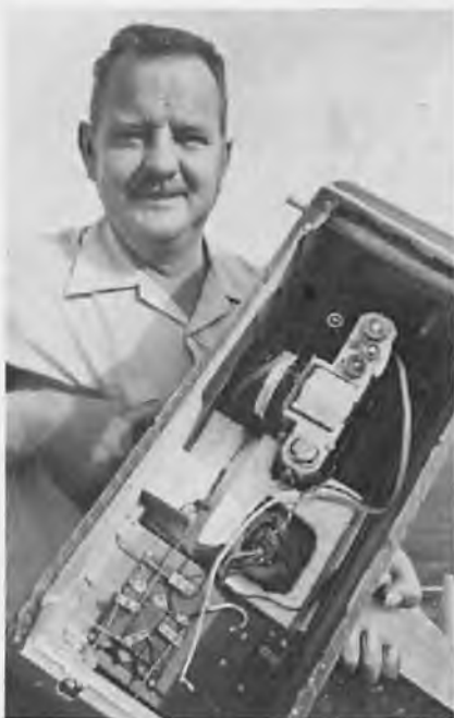
Don Rice from Borger, Texas, with motorized Nikon installation in .61 powered 16 lb. RC model which he used to take aerial photos.
