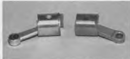
The HB aluminum piston, on the left, uses a Dykes ring, and forged rod that is double bushed. The HGK aluminum piston has a fully machined rod that is bushed on the big end only.
