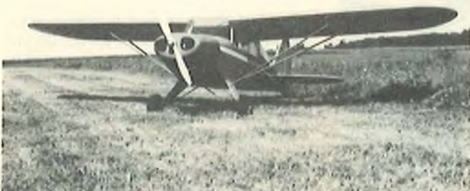
Piper Super Cub by Bill Rose of Dawson Creek, Canada. Model is built almost entirely of foam, mylar covered and flies extremely well. Quadra powered and very aerobatic.
