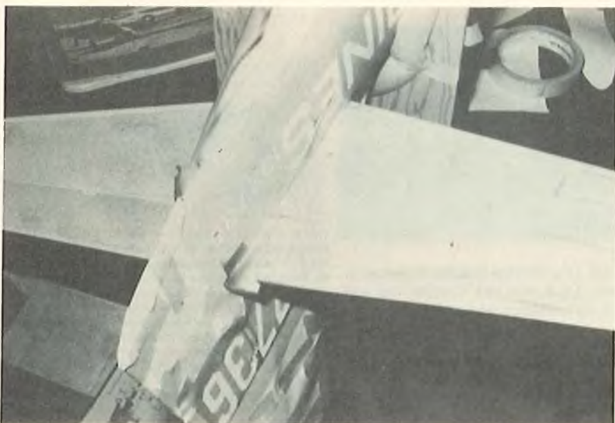
Left side of Stab/elevator sprayed. Right side of Stab/elevator brushed.
