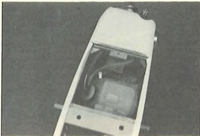
Fuel tank and nose steering installation.
