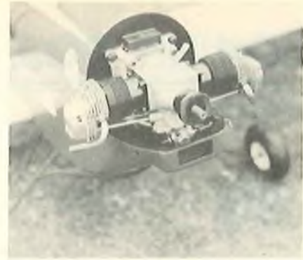
O.S. 1.2 four cycle twin in the nose of modified Lazy Ace — from Holland.
