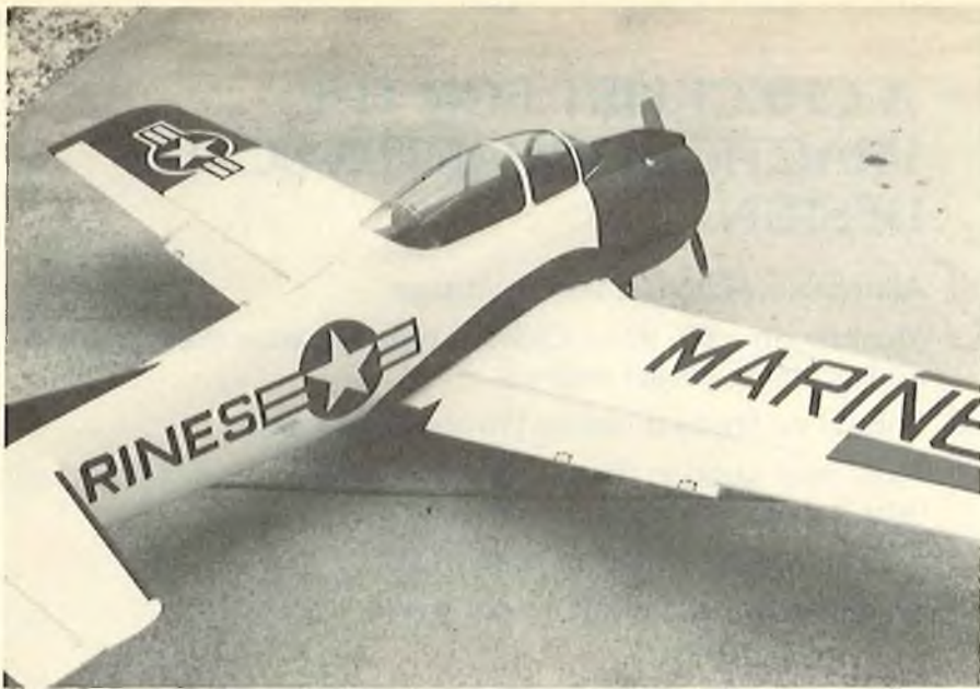
3/4 view of T-28 95% complete. Cowl numbers to be painted, wing walks to install and away we go.
