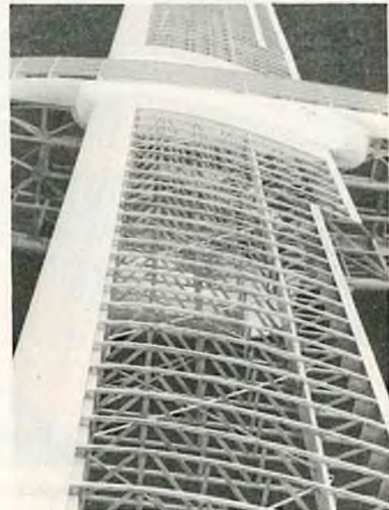
Forty square feet of wing area required the construction of 64 wing ribs at about 30 minutes each rib. Spacing is scale and workmanship obviously of very high caliber.
