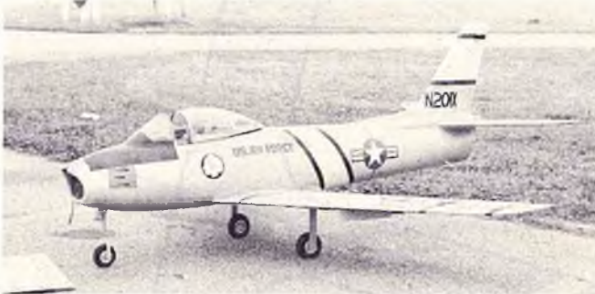
F. J. Gonzalez' big F-86F — only 9.6 pounds with retracts, flaps, and flying on OPS .65 with Byro drive. Power to get off from any field. Realistic in the air. Original design.
