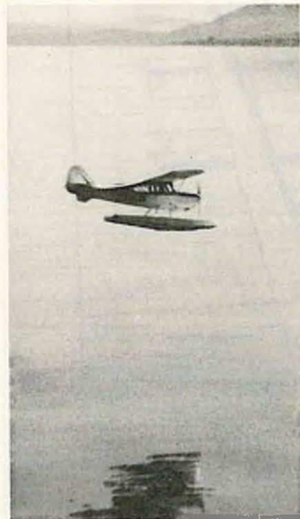
That's the way the lake was most of the time. In fact, some of the full scale jobs had to rock from one float to the other in order to break loose from the surface tension on take-off.
