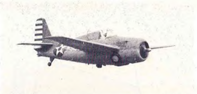
Bob Karlson's FM2 Wildcat flies well on a geared Webra 60. Sportscale at 13 pounds, radio glitches gave Bob problems at East Coast meet. Second high static score.
