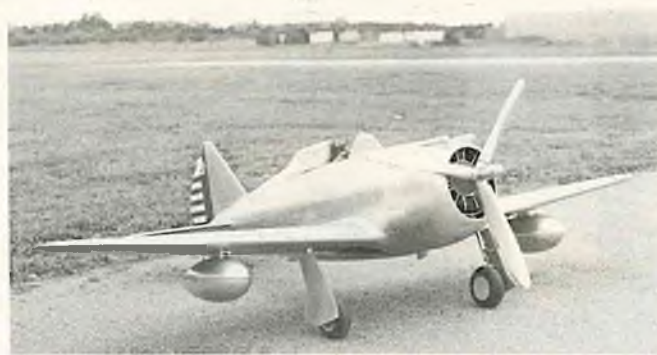
Giant Scale P-43 has home-built retracts to handle 20 pound weight. Quadra behind dummy Pratt & Whitney.
