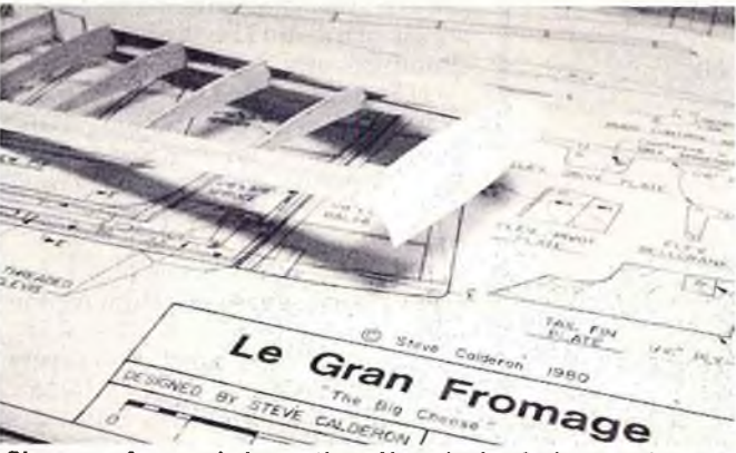
Closeup of carved droop tips. Note lack of shear webs or capstrips in outboard wing panel.
