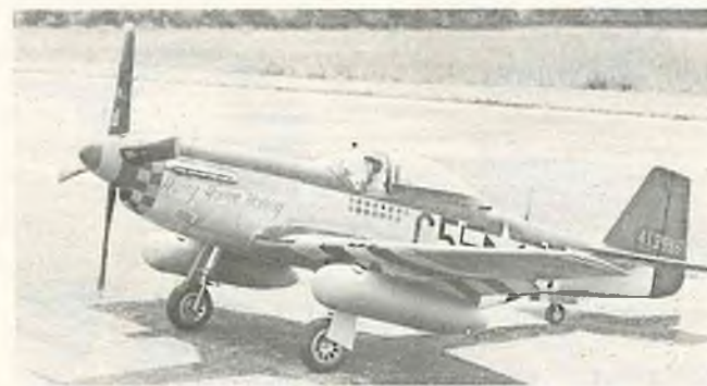
P-51D — Dave Platt's latest — Giant Scale model at 17 pounds, flies with piped Ross 90 using 13/7 prop. Top static points at King Orange.
