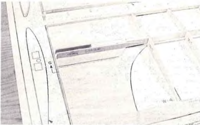
Plywood shear webs in place with stepped balsa shear webs. Ballast box floor with 1/16" balsa spacer underneath can also be seen.
