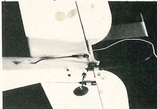
Notice the thin strip of plastic that "captures" the tail wheel wire to yield positive ground steering.
