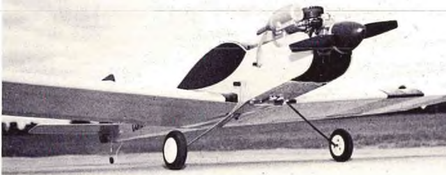
Super Tigre X-25 turns the 8/4 Master Airscrew well over 16,000 rpm's. Corkscrew has been flown with an Enya .19 and was quite docile, but well powered.
