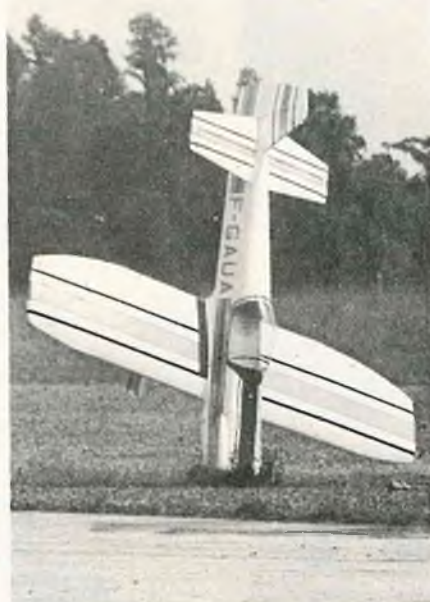
Bill Hunt's Superstar Giant Scale with geared Webra that suffered from overheating. Model tripped up as it dead stuck short of runway.
