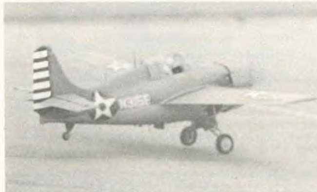
FM2 Wildcat looks real on take-off. Bob Karlson's original has scale working retracts.
