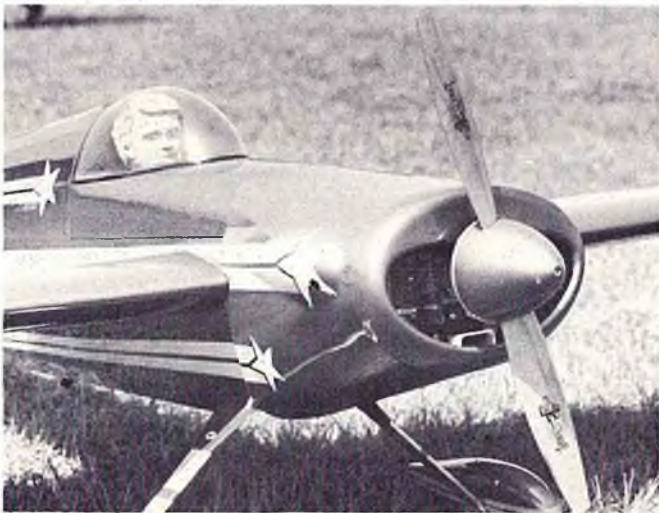
Tartan Twin is well-hidden in cowl of Bob Godfrey's Laser 200. Engine performed magnificently with 20/8 prop. Placed 3rd in Giant at King Orange.
