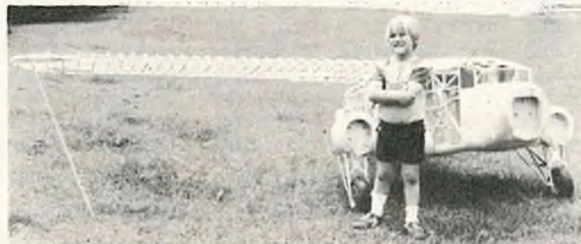
Al Feeley's grandson, Gary, poses with partially assembled Airliner. Power will be two Quadras outboard and a Kloritz in the fuselage. Note the nicely detailed undercarriage. Model will likely try for a long distance record flight.
