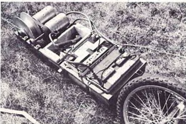
San Fernando Valley Silent Flyers' "Gorilla Winch," two motors, two batteries, one drum. Pegged a 600 ampere meter. Chan photo.
