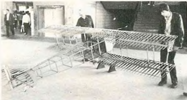
Spad VII at Paris Model Show. Construction conforms exactly to that of the original, and model is powered by a motorcycle engine. (Photos courtesy Georges CHAULET.)
