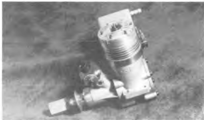
K & B 40 with a Slim-Line muffler. A good "meat and potatoes" scale engine. This particular example was installed in Jack Cole's Jemco AT-6 pylon racer. Engine's reliability is a big plus for scale applications.
