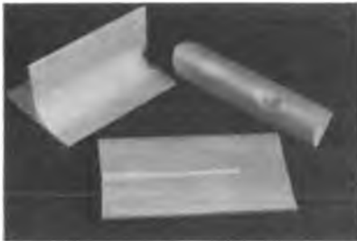
Fillets Gap filling Ding repair
