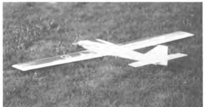
JM Glascraft Electri-X aerobatic ship designed for 05 systems. Uses glass and foam construction.
