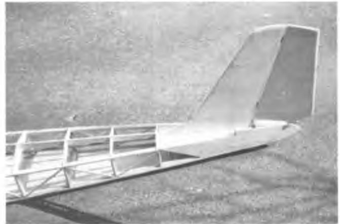
Fin and rudder installed with linkage attached.
