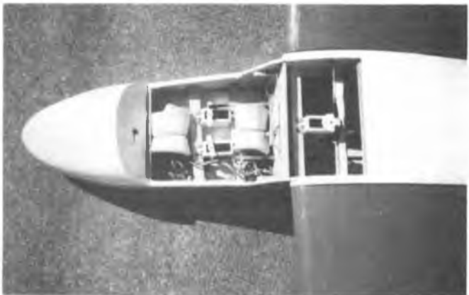
Canopy removed showing the ample room for radio installation.
