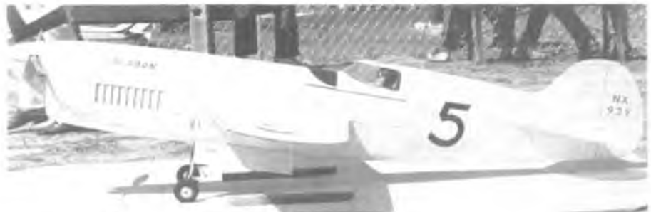
Art Chester's "Goon" in Quarter Scale. Designed by George Fischer, who also designed a scale retract system for the model. Model was built "backwards" — the fiberglass fuselage exterior was completed first and then the structure to connect engine, wing, gear and tail feathers was built to fit inside! A 90 for power and a foam wing.
