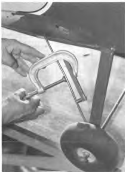
Landing gear wire being straightened with "C" clamp and home brew jig. Over-bending the wire allows it to spring back to original shape. Fixture could be longer for larger models. (#2 is 4 inches longer.)
