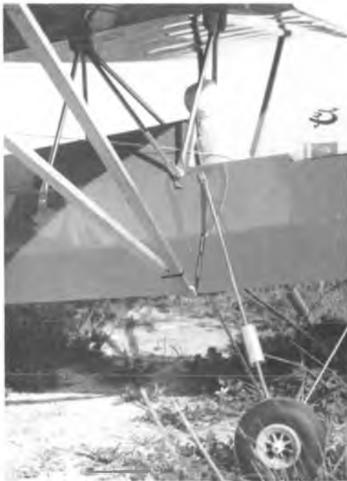
Close-up of cabane struts and landing gear side brace.
