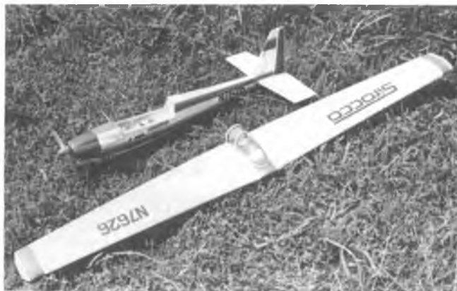
Sirocco broken down for transportation. The pretty model is reminiscent of the Cox Sportavia, but mid-wing allows easy hand launch not attained with low wing sailplanes.
