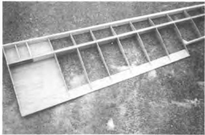
Spar box assembled with brass tubing inside for wing rod.
