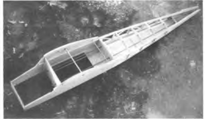
Fuselage nearing completion — note pushrods installed.
