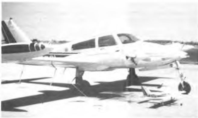
Larry Henderson of Bokeelia, Florida, has taken a Royal kit of the 310 Q and modified it to the K model. Powered by two Fox 45 BB R/C engines and retract system by Rhom-Air. Over five months of work with a little to go. Yet to be flown.
