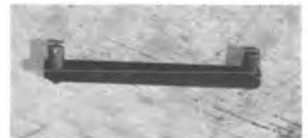
Bar stock wire straightener. Simple and easily made tool is used to straighten non-removable landing gear wires on the model. Saves damaging structure trying to straighten hard wire landing gear struts. More in text.
