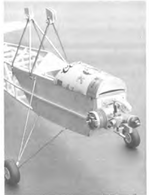
Cabane struts have wing anchors attached. Will be secured into wing.
