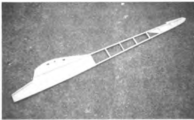
Basic right fuselage side from 1/8" ply and 1/4" sq. balsa.
