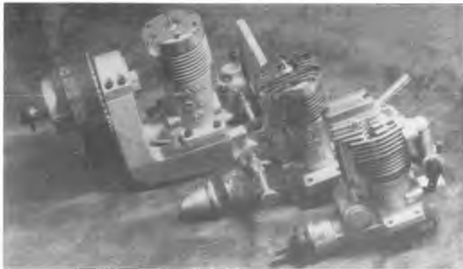
Line-up of suitable-for-scale engines. O.S. Goldhead in "Maximizer" belt drive — works well but drive shaft "wanders" because it's used to tension belts. Old "work horse" Enya 60 in the middle has seen service in three scale models — good engine. New O.S. 40 four-cycle on right has yet to be run — but is expected to perform well in a scale ship.
