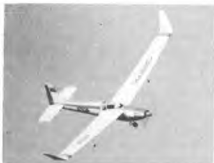
Winglets on Sirocco. This is the first kit the author has seen with winglets.
