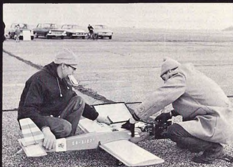
Right: Geoff Pike gives his latest model a quizzical look before starting up. Taurus wing, original fibreglass fuselage and neat "Plane Jane" insignia on the fin. Note silencer on the Super Tigre. F and M proportional gear.
