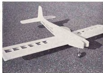
Ready for covering
