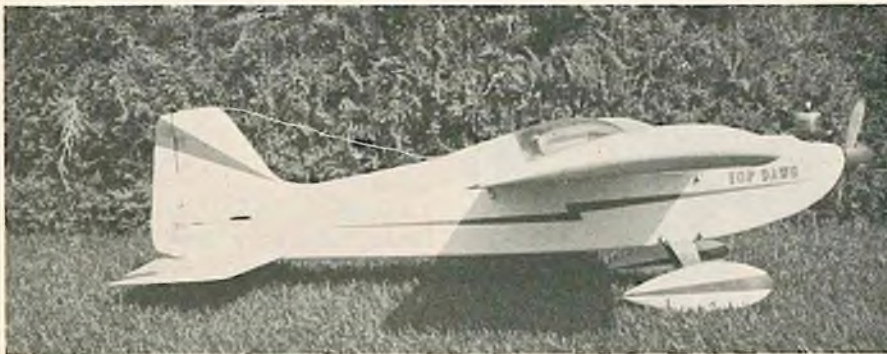
Top Dawg in sidview. 38" span, Orbit 3+1 proportional on R. E. M.
