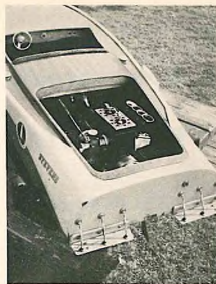
Twin .60 uses steel con rods, ball bearing mounted, original design diaphragm carb. 15,000 R.P.M. alternate firing.
