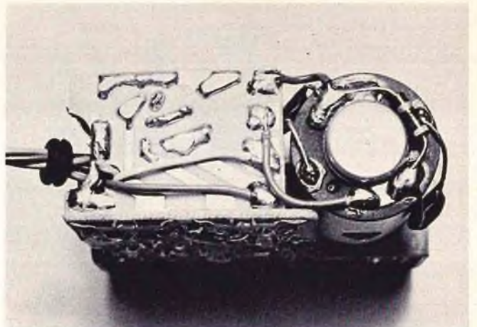
View of base of auxiliary board illustrating motor components and servo wire routing.
