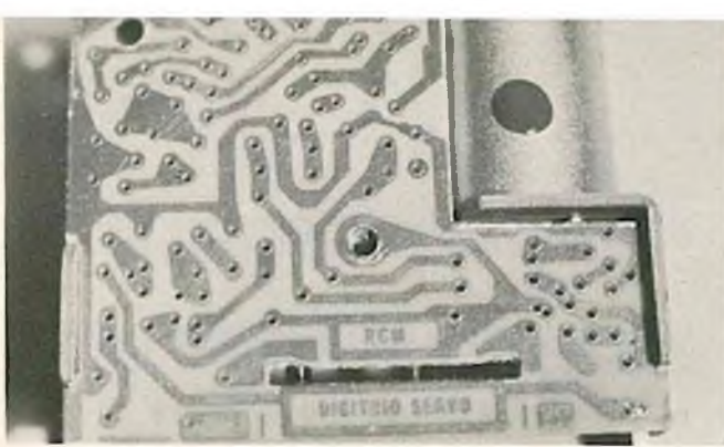
Main PC board fitted to "C" frame.
