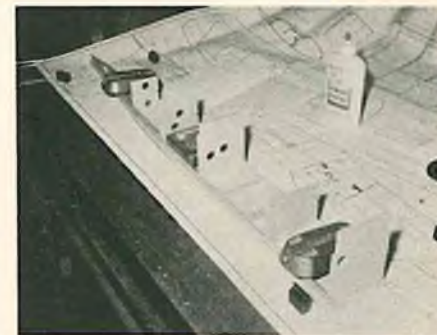
Longerons and bulkheads glued to top sheet.
