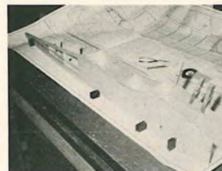
Doublers and portion of rear stringers added.
