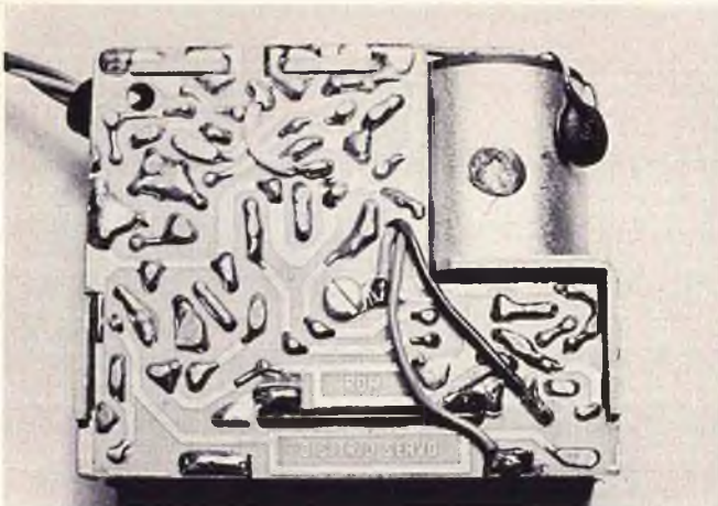
View of base of main board showing routing of wires between lands.
