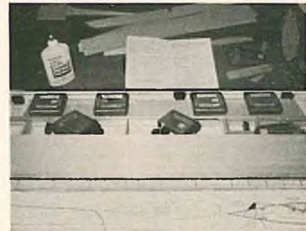
L.E. sheeting secured. T.E. in place.
