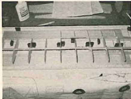
Assembling wing ribs, spars, and T.E.
