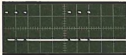
Input: 2 volts/cm vert. 1 mill sec./cm.
