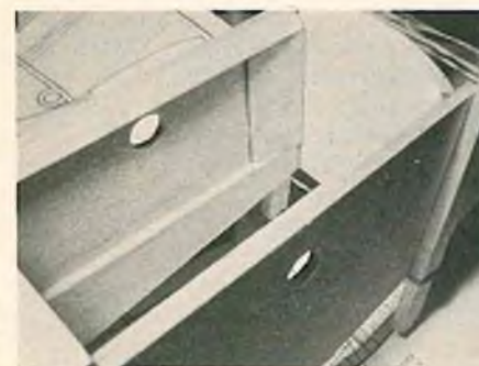
Epoxying fire wall in place.
