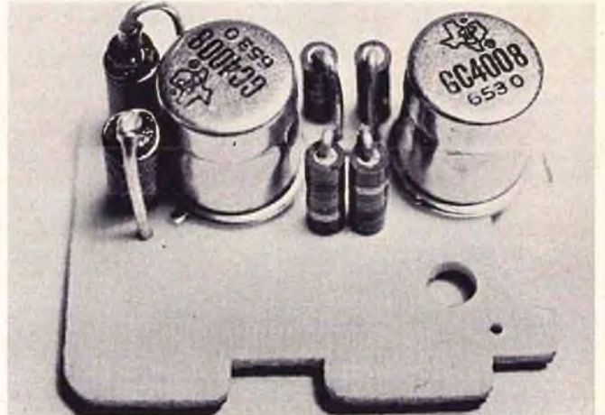
Auxiliary board with transistors, resistors and chokes installed.
