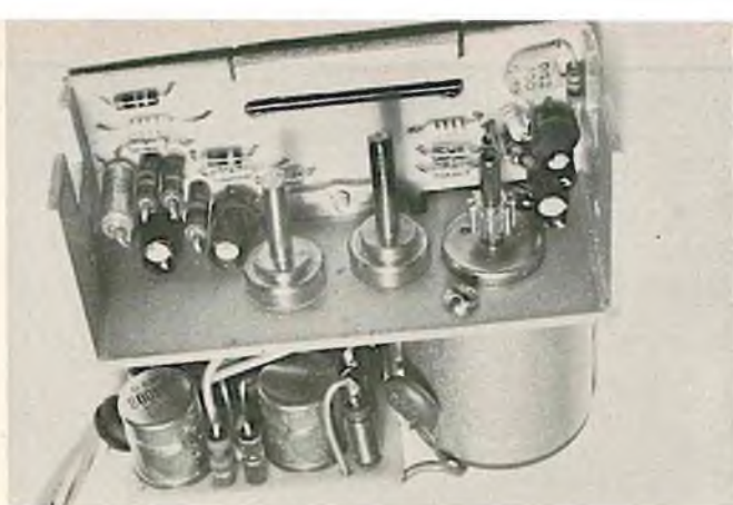
Amplifier installed on "C" frame. Gears and output arm removed in this photo.
