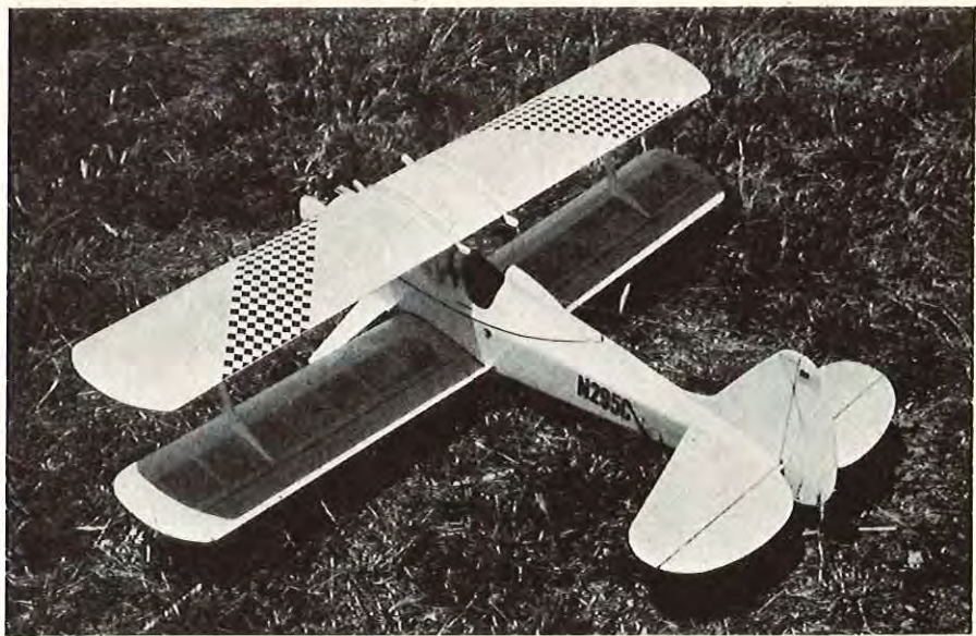
Three quarters view shows ailerons in lower wing. May be coupled with rudder for sport flying.
