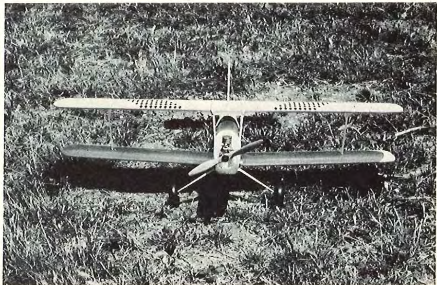
Front view shows straight top wing, dihedral in lower wing only.
