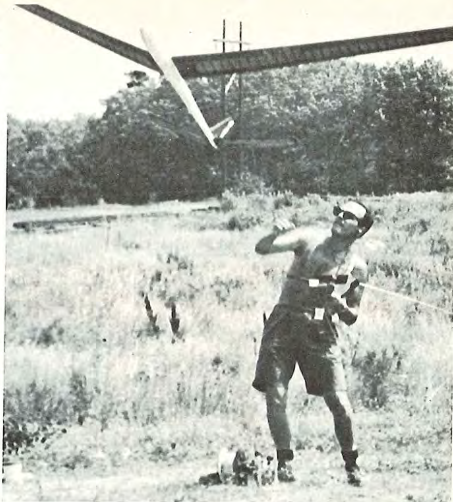
Author launches his Kurwi. Equipment shown includes small, lightweight gas-powered winch with foot controls; transmitter with extra sun shield and stop watch mounted on front; and thermal sensor monitor receiver mounted on a shoulder holster.
