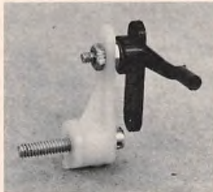
WILLIAMS BROS. SERVO TRAVEL REDUCING LINKAGE WITH COUPLED AILERON AND RUDDER FORK
