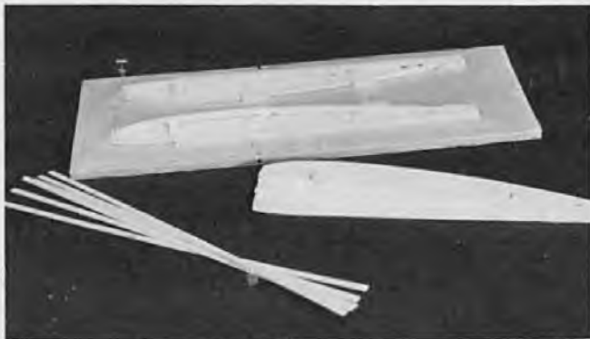
Ribs being capstripped on jig.
