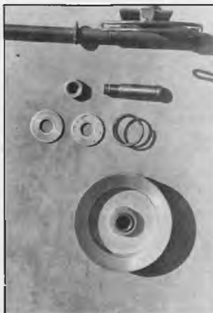
Exploded pulley showing spring which applies light drag on pulley wheel.
