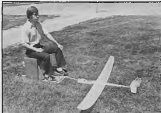
Scott sitting in normal position with heel on pedal. Launching can be a one man operation using a turn-around pulley.
