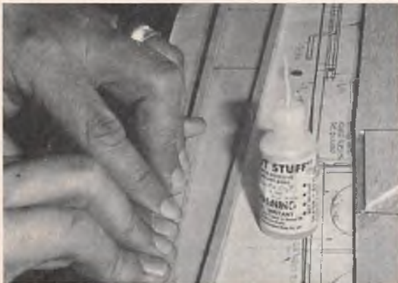
Adding longerons to fuselage sides.
