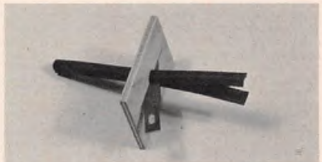
Proper method of retaining blade with fingers. Just pull tubing through blade to cut it in half. Slick and easy.
