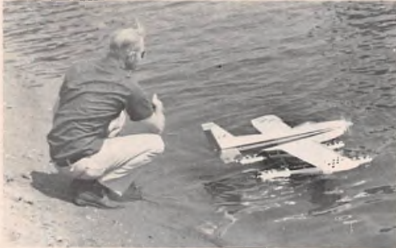
Above and below: Hank Pohlmann gets his feet wet launching the Kiwi, which takes to water like a duck on a pair of 33" Gee Bee floats. Lower right: Jim Duda's Kiwi has a sharp red, white and blue color scheme. Cables from the nose gear steering bracket operate a water rudder on one float.
