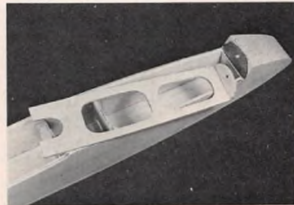
Canopy tray should be completed before shaping nose block.
