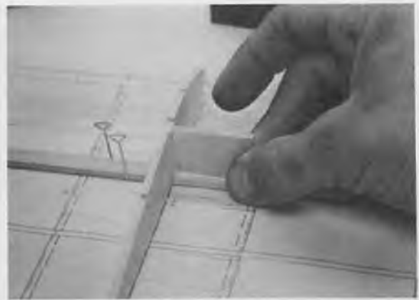
Start with center rib, add web, then next rib. This insures proper contact.
