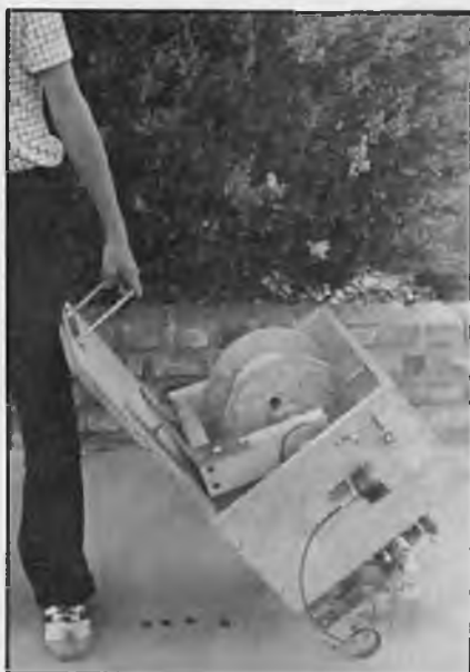
Pulling launcher by line guide on rear wheels. Hole in reel was drilled for balancing.
