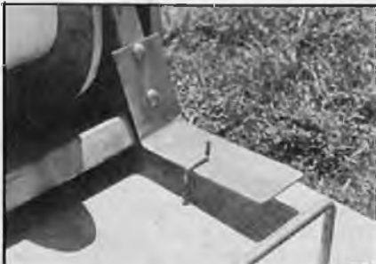
Foot pedal for tightening the belt to drive the reel. Hold-down on pedal is used to hold reel off of the brake to unwind easily. It can be turned out of the way if not wanted.
