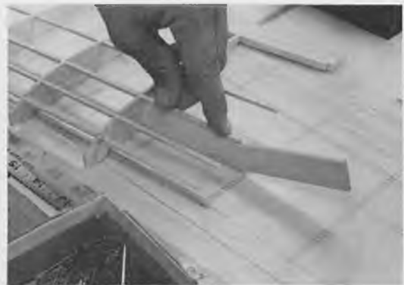
Fitting the wing joiner to the tip panel.
