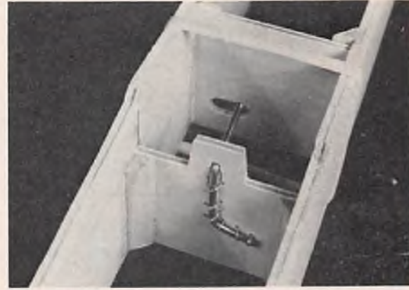
Both fuselage sides together and glued.
