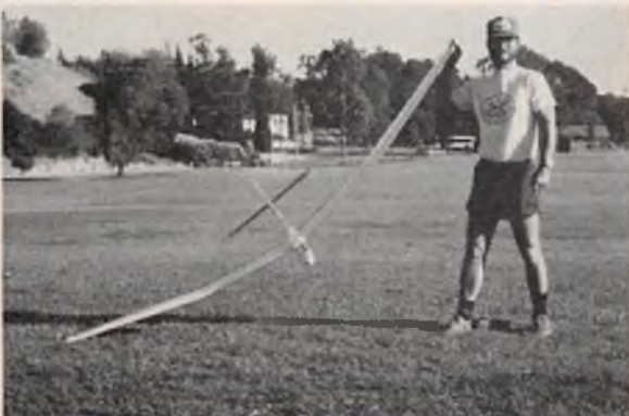
This picture illustrates the best way to test a glider wing prior to winch launch. No bending concentration should appear.
