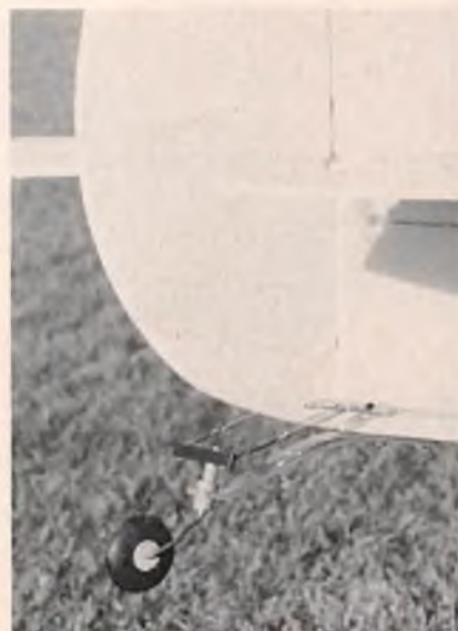
Built up tail wheel assembly.
