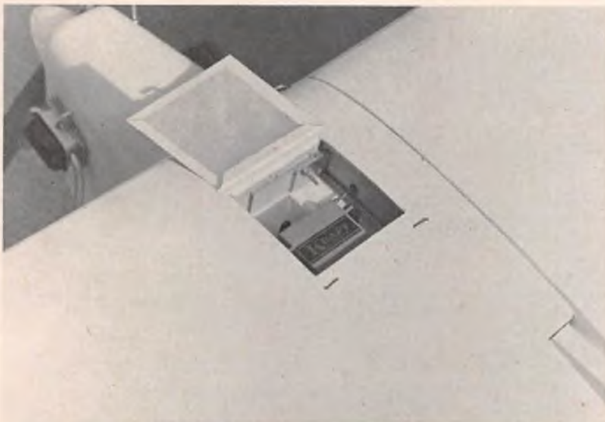
Access hatch for aileron servo.
