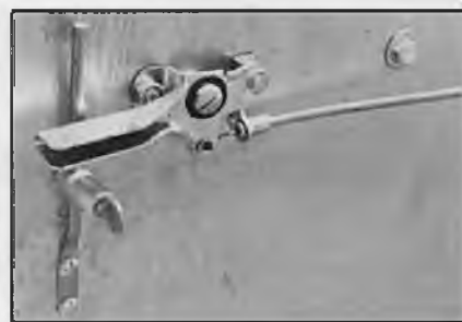
Close-up of throttle, showing adjustable stop.
