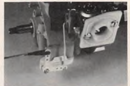
Carb linkage (throttle) for Quadra engine.
