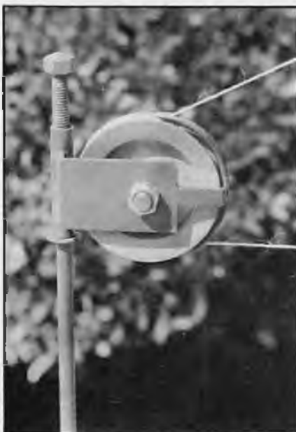
Turn-around pulley showing line guide.
