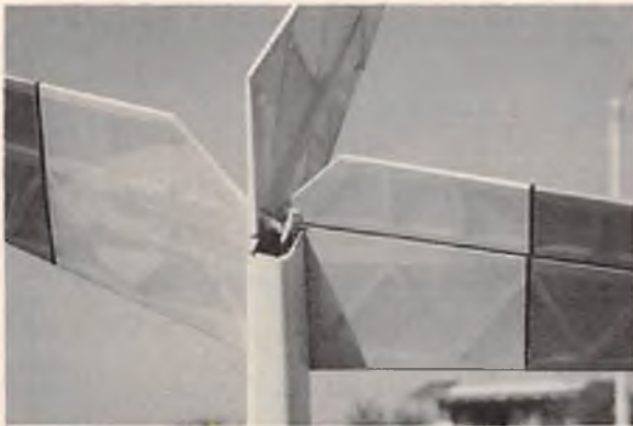
Off-set fin shows neat arrangement for concealing pushrods.
