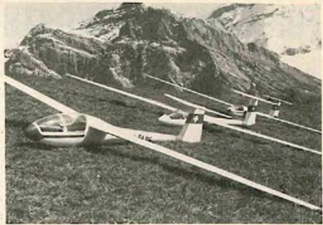
A lineup of the all-fiberglass biggies, (L to R) the LS-1C at 200", Jantar at 178", and the PIK-20D which spans 140".
