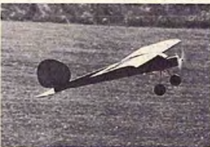
Arthur Garzan's Sweet Stick Astro 25 10/4 nylon prop weighs 5 lb. 2 oz. Won 1st place in "most aerobatic."
