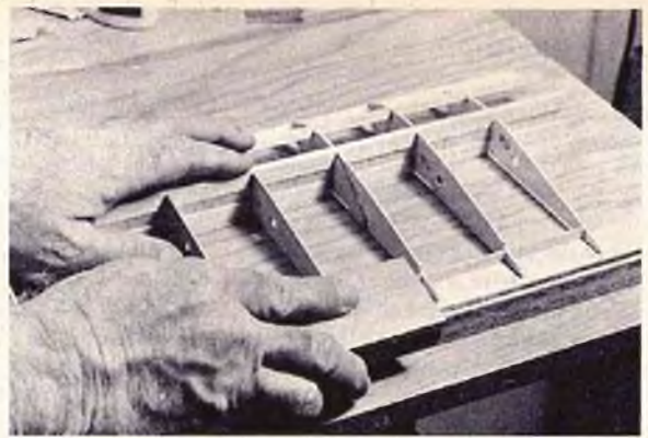
Use fine sandpaper and a block to sand bevel in trailing edge to prepare it for top trailing edge sheet.
