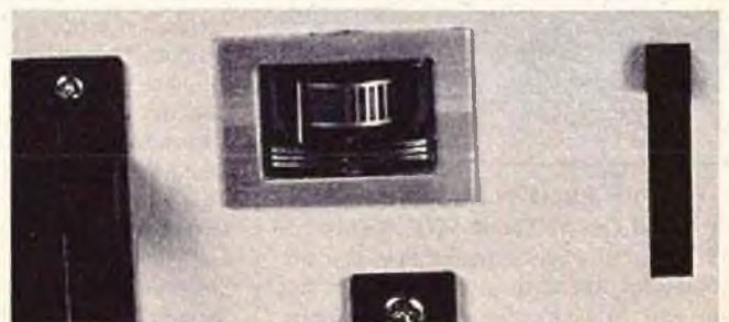
Meter with bezel installed, a nice feature if the hole is inadvertently made over-size or with a jagged appearance.
