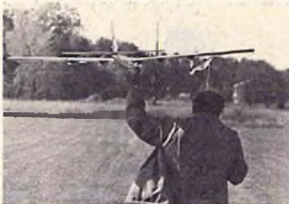
Heinz Koerner with Quad Astro 020 original. Two Inboards winding up. Heinz will switch two outboards on, then let go.
