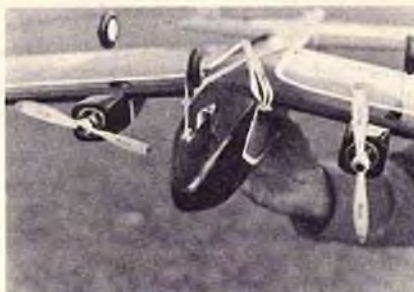
Bottom of Skylark showing air cooling vent.
