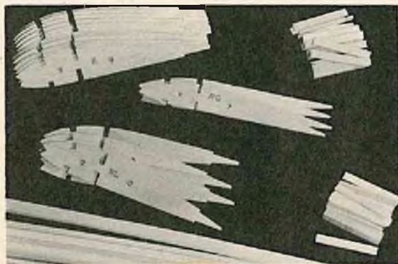
Wing kit, spars, ribs and webs. RL's and RC's are all made from regular ribs.
