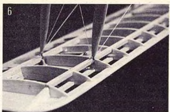
(1) Rear view of uncovered Avro. (2) Another view from the front. Skid keeps the nose-overs to a minimum. (3) Aileron detail viewed from the top. (4) Tip skid shown along with aileron set-up. This gives slight but not noticeable differential action. (5) Bolt-on center section arrangement on top wing. (6) Struts are retained on hooks by elastic thread which wraps around hook. (7) Rear skid struts engage on angled prongs projecting from lower wing center section.
