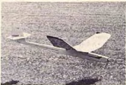
John Henderson's magnificent original 6' Astro 05 powered glider. E385 airfoil, 575 sq. in., 36 oz. First Place in "Best Looking" and First Place in "Longest Flight Time." Unplugs, folds, and otherwise collapses and packs into attache case along with transmitter, field gear. Super job!
