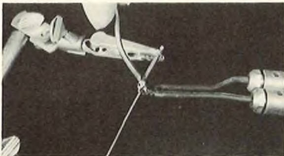
LEFT: Solder the wire to the screw. The use of a "third hand" is quite helpful. Use rosen-core solder and clean the screw and wire well before soldering. Use plenty of heat and get a good shiny joint. RIGHT: The completed link. Make a "Z" bend in the wire to attach it to the output arm of the servo and the screw end will match either NyRod or clevis.
