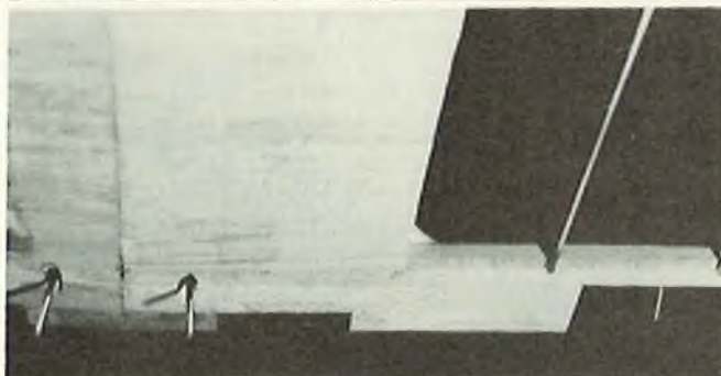
Bottom of wing center section showing aileron horn wires installed.
