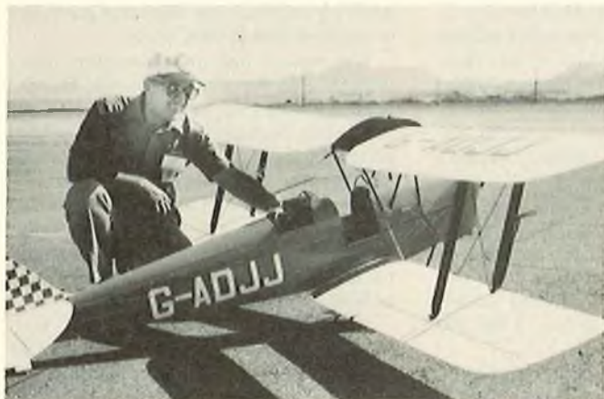
John Pahlow's immaculate Tiger Moth was built from a Toni Clarke Practical Scale kit. Quadra power, 27 lbs., Permagloss covering.
