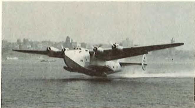
Boeing 314 flying boat with sponsons for lateral stability on water.
