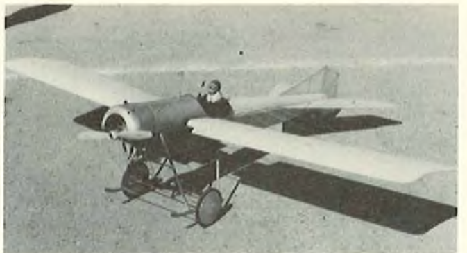
John Greenfield, London, England, brought his 1912 Blackburn. Span is 94", weighs 14 lbs., and is powered by a 2.2 Kawasaki.
