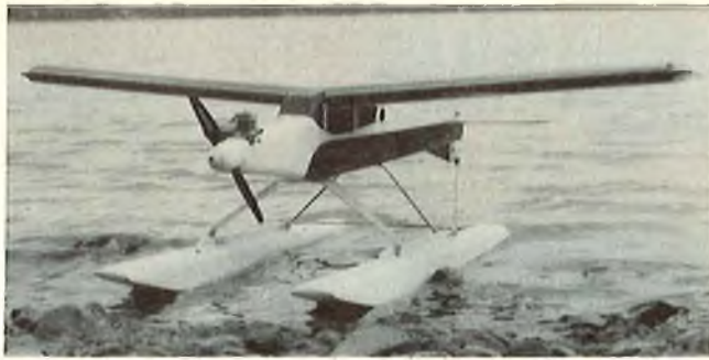
3/4 view front shows "spread" on floats for good lateral stability on water.
