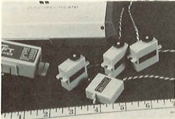
LEFT: Not very big but plenty of power for .15 and down size airplanes. The single grommet mounting at each end of the servo tends to allow them to rock when a one-sided load is applied to the output arm. RIGHT: The solution. Servo tape (double stick) and a block of foam make a very solid tray mount. Three servos can be mounted side by side using just tape between them, or a combination of tape and foam to change their spacing.
