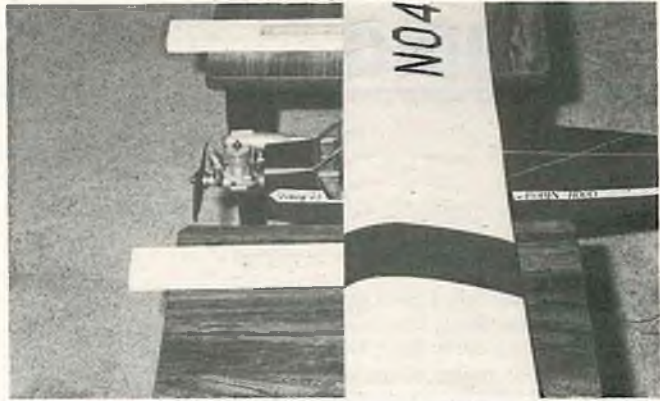
Place the aircraft on the balancing tools as shown, making sure they are in line. Balance aircraft by sighting in a level position. Low wing airplanes can be turned upside down.
