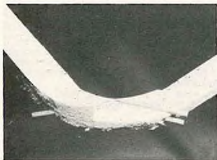
Three part wing tip corner is tied together after gluing by drilling into joint with a slightly undersized drill and driving glue coated cocktail toothpicks through joint. Penetration is indicated by half toothpick lying on top of material.
