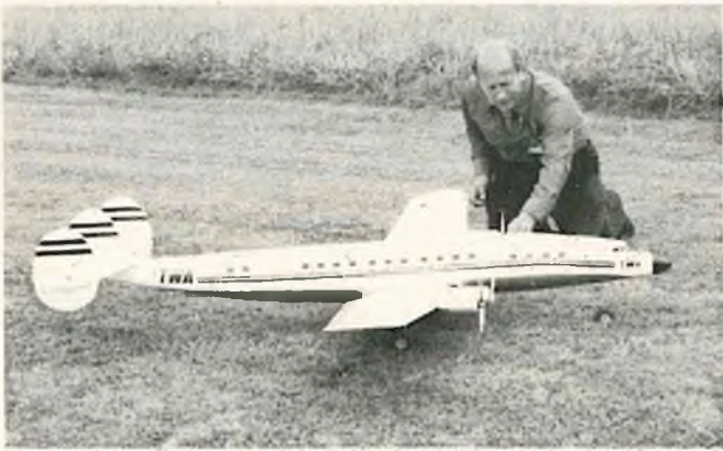
KRC's Heinz Koerner with scratch-built Lockheed Constellation. Powered by four Mabuchi 550's, 98" one piece wing with 76" fuselage. It was not completed for fun fly. Weight — approximately 10 lbs.
