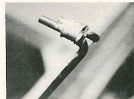
Joint after soldering with solder with melting temperature of 275-300°C. Joint is much stronger than copper wire and ordinary solder joint and heat required will not affect temper of the wire.
