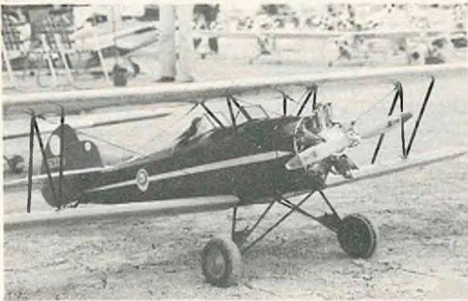
Forest Edwards' Fleet Trainer is powered by his famous 5 cyl. 4 stroke engine.
