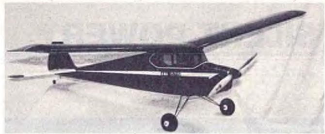
Mel has over 300 flights on this bird, 600 sq. in., 54 oz., geared Astro 075 with 12 550 mA cells, Futaba 3 channel, 11/8 Rev-Up prop. It will do consecutive loops from level flight. Many thermal flights of over 30 minutes.
