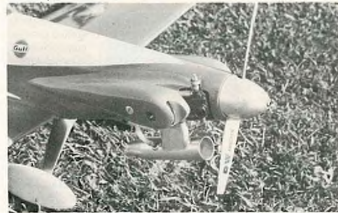
"Business End" of "Denight Special." Mac flow-thru muffler, D & W 8 1/2" D. — 6 1/2" P. prop.
