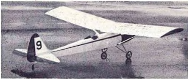
This Thomas original design is a 450 sq. in. Astro 05 Cobalt powered ship covered with Mica film. It uses 7 cells and an 8/4 prop — it climbs like the devil!
