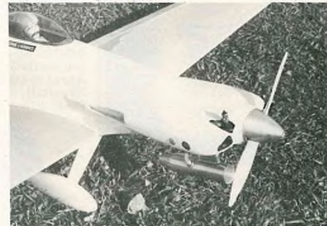
Prather "Lil Toni" owned and flown by Ernie LaChance — built for Formula One-40 racing. Weight 4 lb. 4 oz. with 500 mA battery pack.
