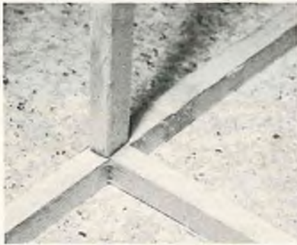
Bare bones fuselage framing butt joint. Glued area is minimal and joint is quite weak.
