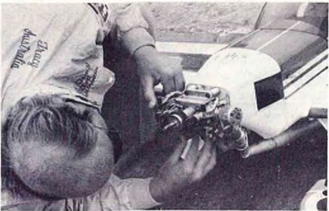
Jeff Tracy used a Webra Twin installation in his Cap 21.
