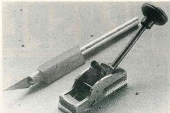
Brookstone's brass thumb plane, with a No. 1 X-Acto knife to show scale. Tiny plane is perfect for rounding leading edges. Plastic pencil holder on X-Acto, found in a stationery store, is great to keep it from rolling off the workbench!
