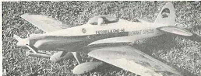
"Denight Special" built expressly for Formula One-40 event by Bob Wallace — weight 4 lbs. 4 oz. Original molded fiberglass fuselage, foam/balsa wing, EconoKote on wing and tail surfaces.
