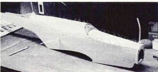
Top sheeting being added to fuselage — note nylon ties along with pins used to secure balsa to basic frame.
