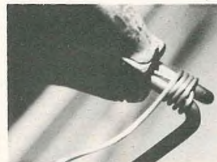
Vice grips hold wires in place while being wrapped with steel wire (not piano wire). Note that end of wire is wrapped under turns of wire holding parts together.
