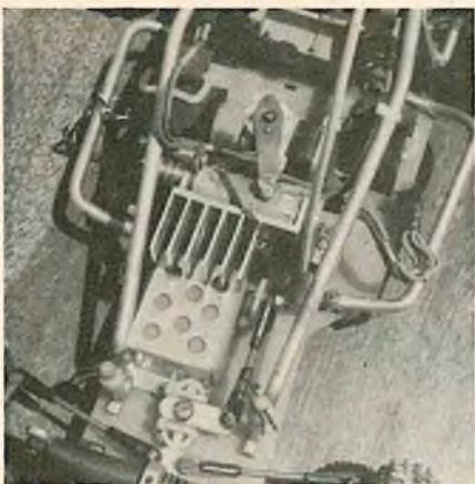
Resistors also get hot so large heat sinks are also used for cooling. Notice the nerf bars which are a necessity.
