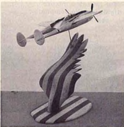
The wing and the base are laminated. The music wire is epoxied to the wing.
