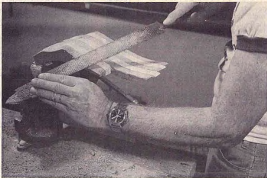
A coarse tooth rasp will be the best way to form and shape the wing.
