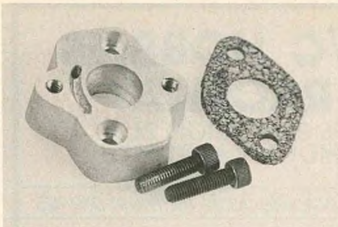
Don Harris carburetor adapter rotates carb for ease in control installation.
