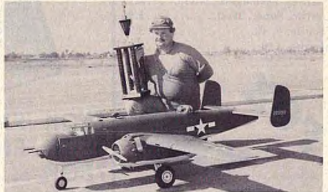
John Lockwood was third (1/4 point behind 2nd) with B-25G-10. Wingspan of 1015", weighs 22 lbs. Scratch-built retracts. Working bombay doors and bomb drop. HB engines.
