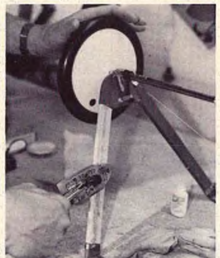
A heat sealing iron will then pull the material very tight on the wood fairing strips. Glass or epoxy resin is then painted on the cloth and the resulting dacron and resin sheath secures the fairing solidly to the wire gear leg.
