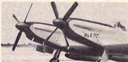
Scale props add character to Art's F-82E model. Twin O.S. .60 FSR powered, the F-82E was first in Sportscale at the King Orange.
