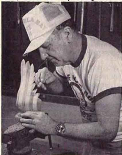
After the wing is shaped, the feathers are cut with a coping saw. The hobby knife helps to trim the feathers.
