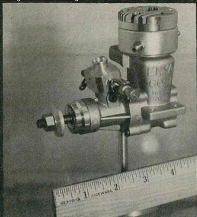
Enya 60 IIIB TV marine engine — note the water jacket and hose fittings for water cooling.
