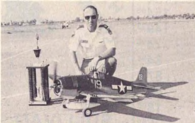
Fourth place was taken by Garland Hamilton with his 1/8 scale Grumman F6F-3 Hellcat. Immaculately detailed, weighs 11 lbs., and powered by HP .61 engine.
