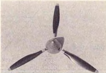
Balsa blades ready for installation in balsa spinner. Pitch angle is set when you glue blades in place.
