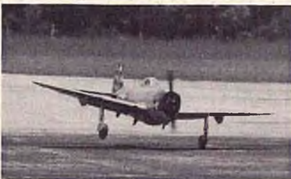
Vito Tomeo's 1/6 scale P-47 landing at the King Orange. The 20 pound model powered by an O.S. .90 with belt drive flew in Giant Scale.
