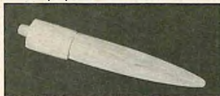
Balsa blade roughed out with sharp knife ready for sanding block. This one is a reject, shape not right. If at first you don't succeed, try . . . try . . .
