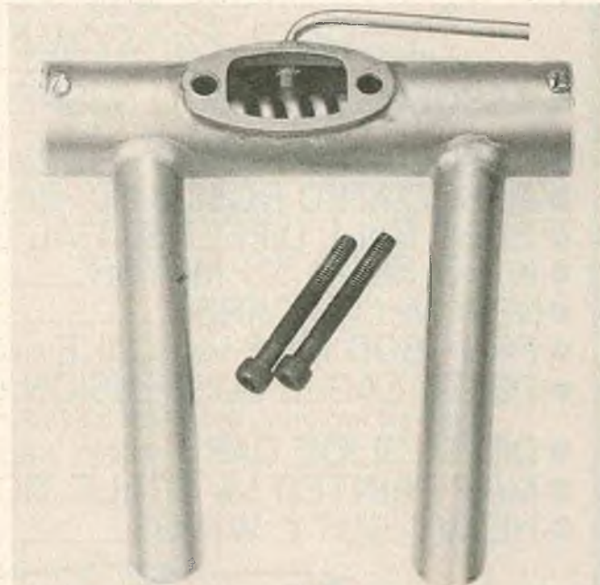
The muffler/exhaust manifold shows the pre-heating coil for the smoke generating system. A Don Harris accessory.
