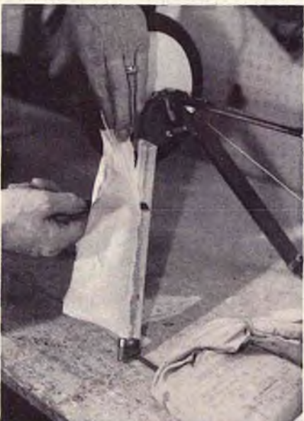
A sharp knife is then used to remove the excess dacron.
