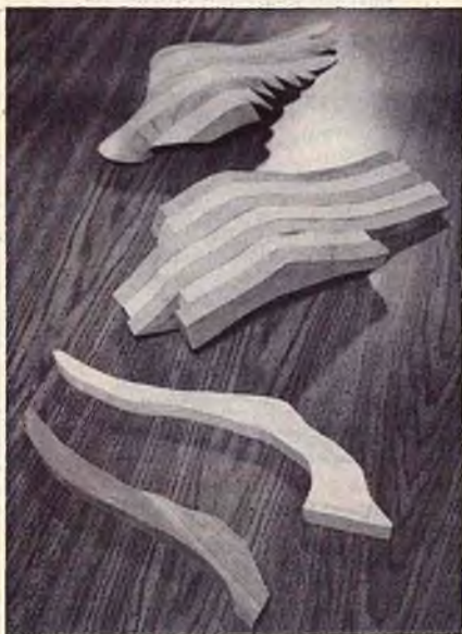
The pieces are cut out with a jigsaw or a coping saw, glued with a shop glue. Clamped and left to dry overnight.
