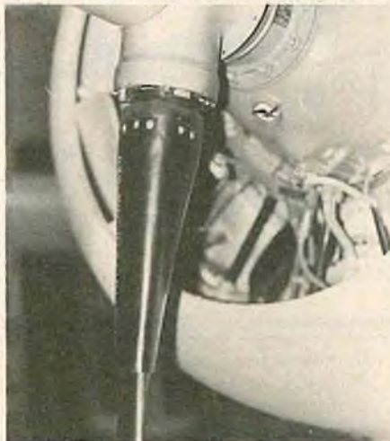
This shows how to taper the cuffed end of blade towards the round hub. Curtis Electric prop on WW II Wildcat.
