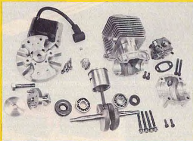
Parts break-down of the G-38 Quartz (shown without the Don Harris accessories).
