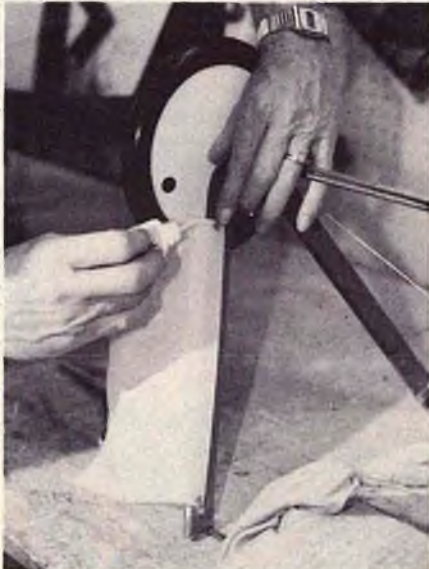
Appropriate length of dacron is tack glued to back side of wooden strut. Dacron should be pulled tight between two dots of glue.
