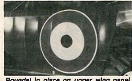
Roundel in place on upper wing panel. Chord is 22 inches. Spraying with flat clear eliminates shine in Olive Drab base color and conceals brush marks in roundel.
