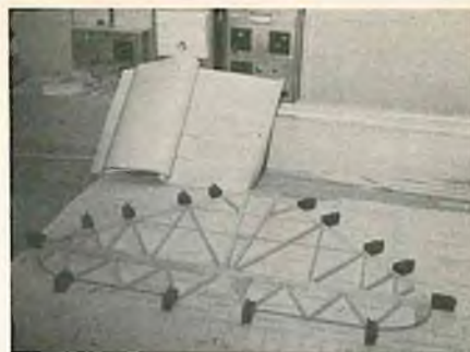
Stabilizer and elevator framework.
