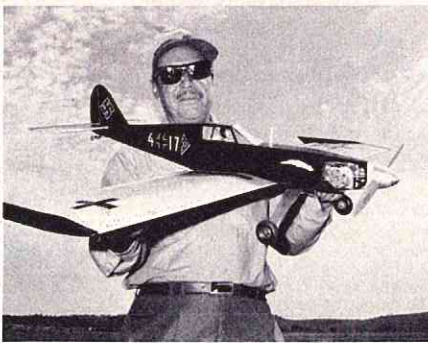
Another diamond airfoil entry in unlimited was 42" span original by Emilio Lozano. ST .40 ABC engine, Kraft radio. Flew well at 3½ lbs. in mile-high Puebla altitude.
