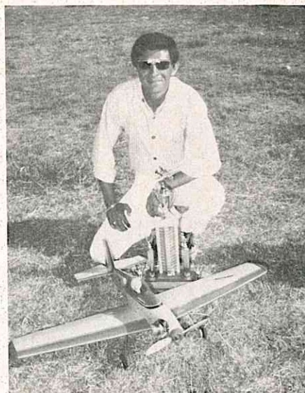
RIGHT: Luis Castaneda Jr., fastest RC'er in Mexico, with original midget Midget Mustang. Ship, an amazing 2½ lbs. with K & B .40, 3 Orbit servos, 10 oz. fuel tank. Span 39", 300 sq. in. Despite size, stable and easy to fly. (Future RCM feature).
