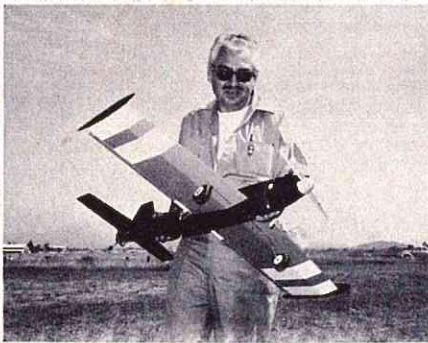
Lightest Puebla Ciclon racer, 2½ lb. ship by Gaston Mathelin placed 2nd. Diamond airfoil shows George Killeen design influence. K & B .40, Logictrol radio.
