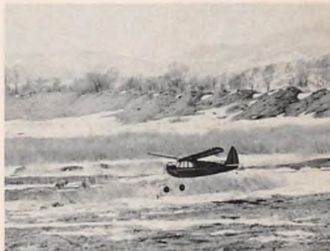
First flight take-off. Buffalo grass and snow patches, plus a rich engine run, held the Super back; but with 1600" of wing lifting, the model was airborne in 60'. And – it flew SLOWLY!
