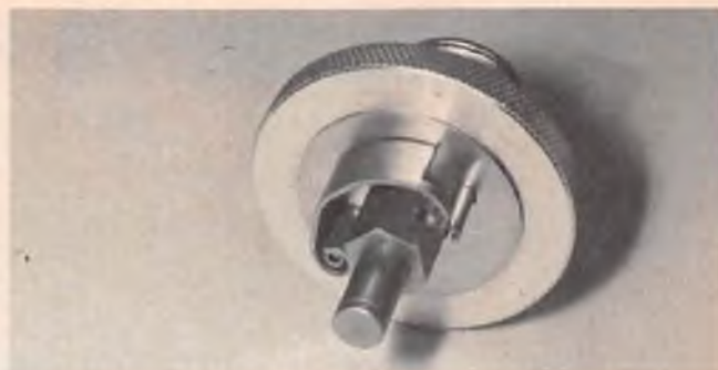
# 4: This shoe has been lightened on the swing end which allows the clutch to slip more, making it easier to drive on most tracks.
