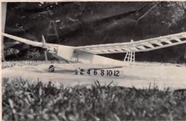
Butterfly II complete with the exception of the cabin structure. This is left to the end so as to locate wing properly with respect to the C.G.
