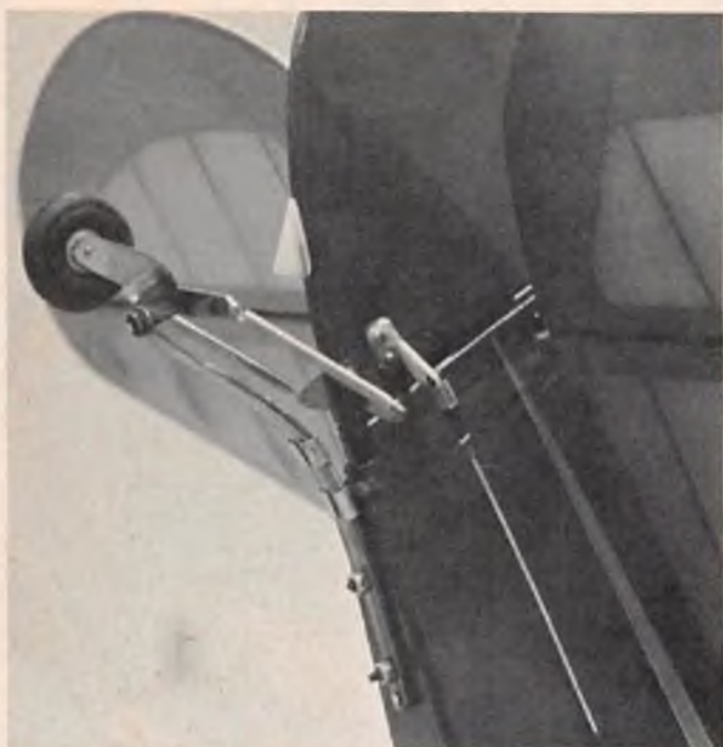
Scale-like Wimpy tail wheel was built by Bill Tuttle – who is a locksmith by trade. Anti-scratch rudder bumper isn't needed.
