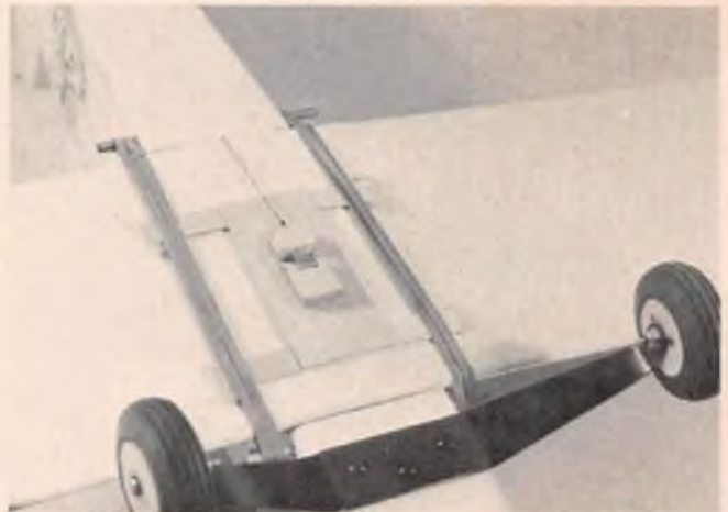
Bomb release mechanism mounted and ready. Trip line is attached to throttle servo arm in fuselage. Bomb release is easily mounted under rubber bands holding wing.
