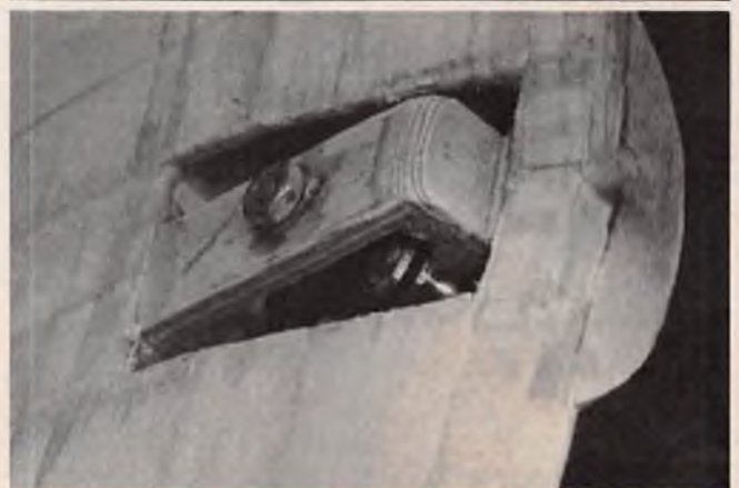
Servo wheel installed on the centerline of the wing. Vertical 3/8" strip of plywood, with horizontal servo mount strip reinforces the wing. Servo wheel is held in place with a 4-40 bolt through a blind nut. Note the ball-link.
