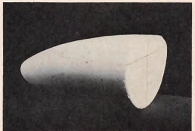
Photo 4. The form has been shaped and is ready for the glass cloth. The block was roughed out with a hacksaw blade, rough sanded with #80 garnet paper and finished with #150 garnet paper.
