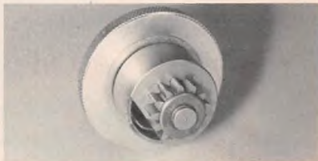
# 6: A simple method to make sure you're getting good shoe contact with the clutch bell, is to cut a hole in an old clutch bell and look through the hole to check alignment.
