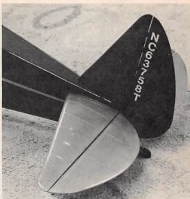
Fin and rudder of the Super are a half-yard high and are covered with silk and clear doped as is the rest of the model.
