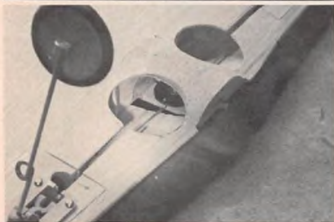
FW 190 gear extended. The 90° bends on the end of the actuating rods haven't been secured yet with nylon wire retainers.
