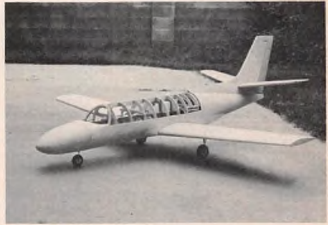
Photo 6. The top has been covered with heavy glass cloth and the whole part sanded smooth. Then both the bottom and top were covered with medium weight glass cloth. In mixing the epoxy, pour one part in the cup, add micro-balloons to a paste consistency, then add the second epoxy part, stir well and apply. The 10-Minute epoxy allows ample time if you don't fool around too much. The use of micro-balloons keeps the epoxy from running and also makes the epoxy easier to sand.
