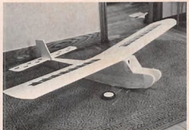
Almost ready for covering. Note the camera port-windshield.
