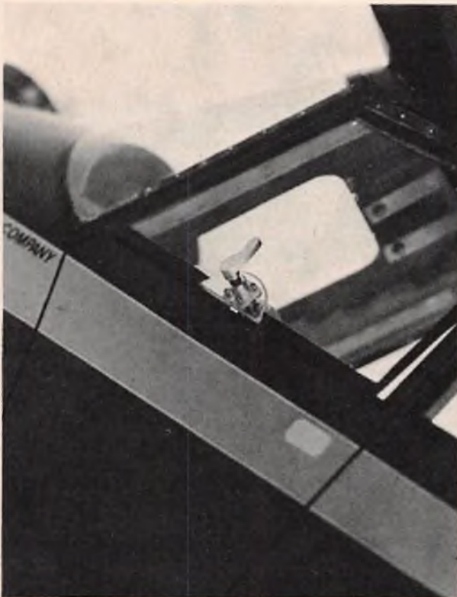
Close-up of the cabin window latch. Super Wimpy's wings are bolted and doweled into position so opening hatch allows receiver switch to be protected inside. Side windows are 1/16" Plexiglas.
