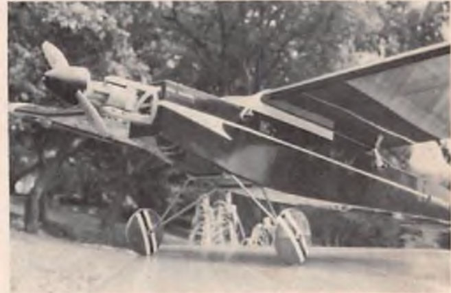
Completed aircraft showing the cabin structure added. Note the built-up balsa and ply wheels to save weight.
