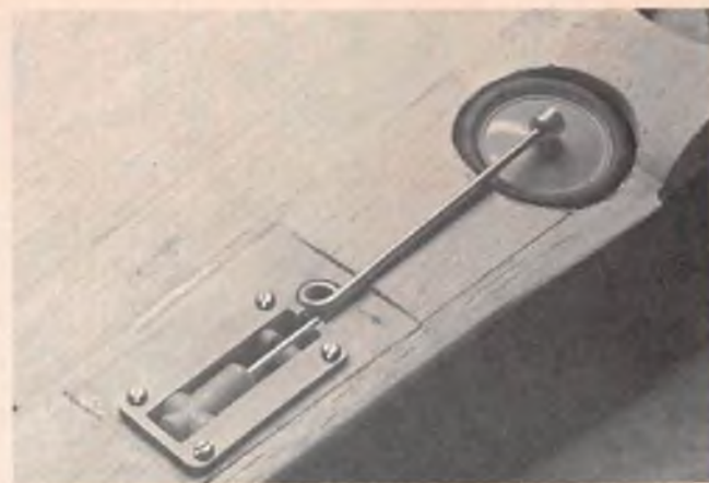
Left-hand gear leg bolted to its plywood mount. Ply is epoxied to two wing ribs, rests on the "false" leading edge and butts up against the real leading edge and lower main spar. Model in the photo is a HOB FW 190.
