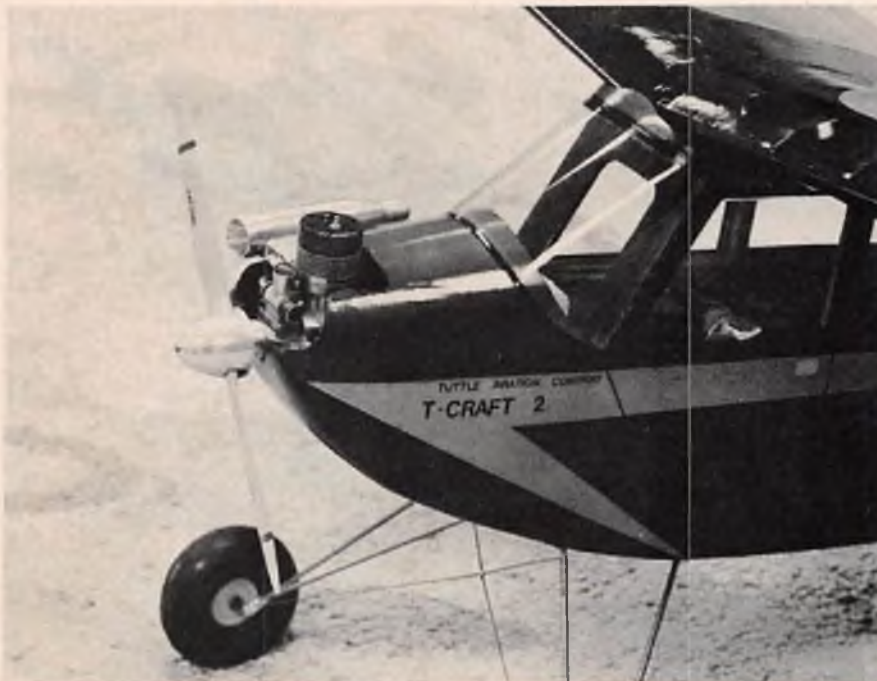
That's a 78 in the nose! And the wheels are six-inchers! 6" were added to the nose of the enlarged Wimpy, but 2½ pounds of lead were still necessary to bring the big bird into balance.
