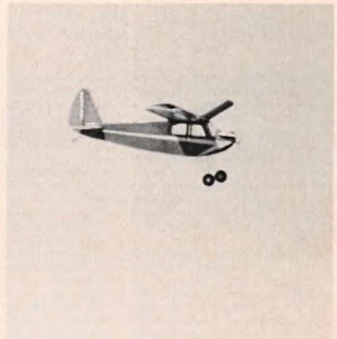
Fox 78 is lost in the nose of the Super Wimpy. The wheels are six inches on 3/16" struts. Dentist Dr. Roger Tennyson designed the original Wimpy that was the basis of the Super.
