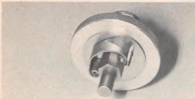
# 5: This is an extremely lightened shoe which works exceptionally well on very slippery tracks. Caution must be taken not to go too light.
