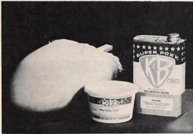
Photo 7. Now that the shell is sealed with epoxy, any irregularities can be filled with a paste made of resin and micro-balloons. After sanding those filled places smooth, apply a coat of resin to the entire part. Sand the resin smooth and you should have the nice fiberglass that you need.
