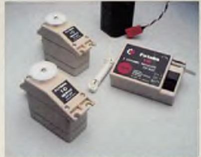
The FP-2F system includes two S7 servos and a double-tuned, RF amplified receiver.
