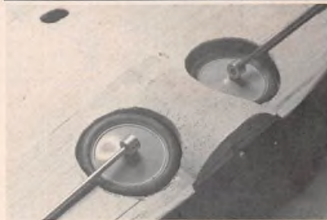
Wheels tucked away in their wells. The wheel holes are about 1/32" larger than the wheels to permit lining them later with card stock. Hole to the right of the wing centerline is to allow access to the Du-Bro servo connector set screw - which allows adjustment of the "servo wheel to servo" pushrod.
