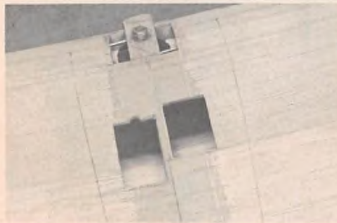
Retract servo goes in the hole to the right of the doubled center ribs - the aileron servo goes on the left. The position of the actuating rods shows that the gear is retracted.
