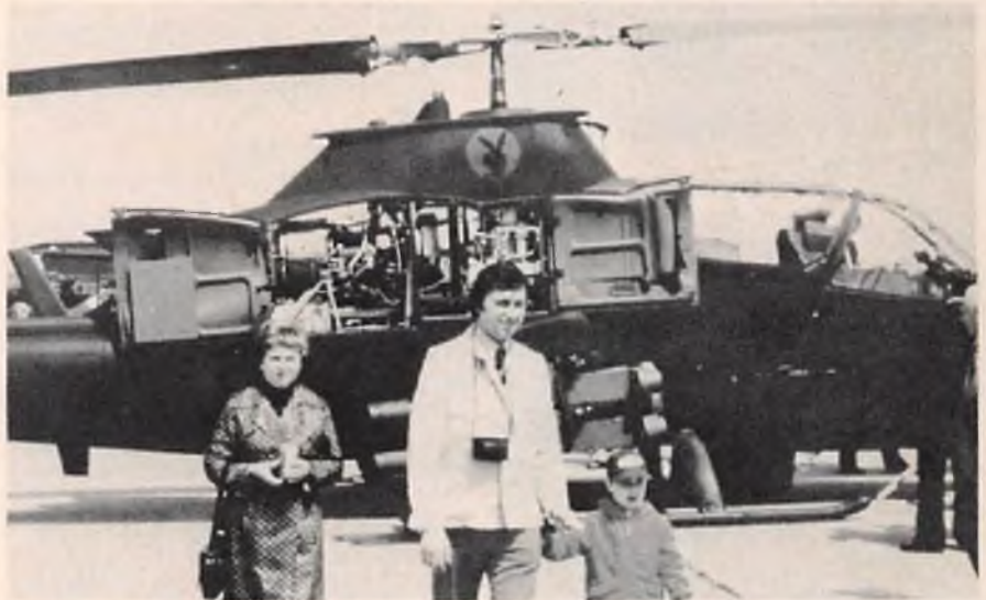
AH-1Q "Cobra" belonging to the 334th Attack Helicopter Company. Cowling is opened to reveal the engine and transmission. This is "Q" Model, designed to fire the tow anti-tank missiles.
