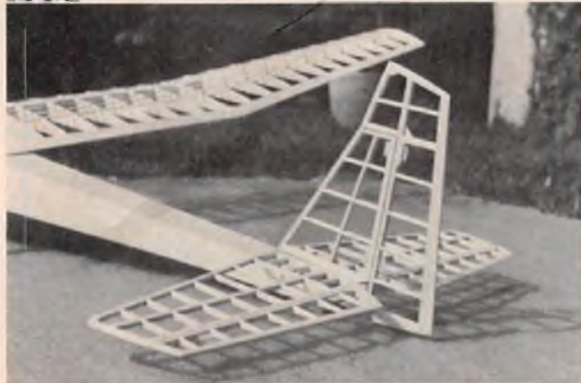
Completed tail group ready for final covering. This shows the long tail moment on the Butterfly II. Very important to keep weight as far forward as possible.
