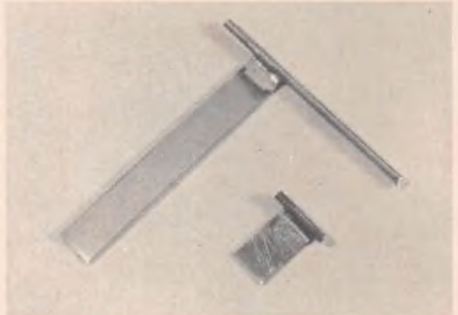
Solder lever parts together using larger pieces. More manageable this way. Then trim 'em to size.
