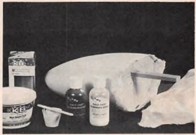
Photo 6. The top has been covered with heavy glass cloth and the whole part sanded smooth. Then both the bottom and top were covered with medium weight glass cloth. In mixing the epoxy, pour one part in the cup, add micro-balloons to a paste consistency, then add the second epoxy part, stir well and apply. The 10-Minute epoxy allows ample time if you don't fool around too much. The use of micro-balloons keeps the epoxy from running and also makes the epoxy easier to sand.
