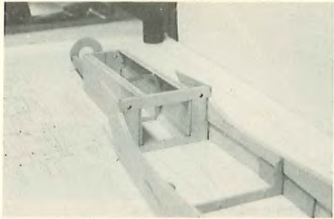
Fuselage built flat on board over plans, makes for a square fuselage.
