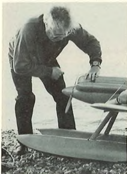
Author starting up the Quadra — needed fins filed down to enclose it in cowling but did not lead to any overheating problems.
