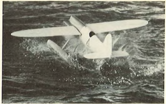
S-4 away for a short flight. Note right rudder held on to counteract torque and 'P' forces, pushing the port float into the water.
