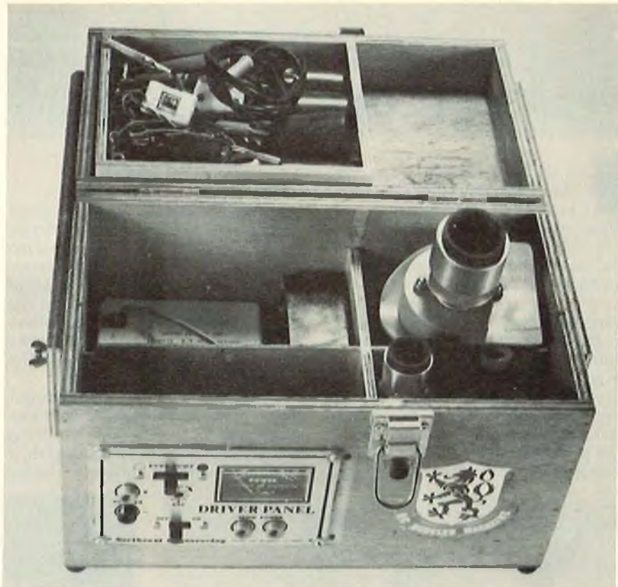
The Northeast Engineering Driver Panel mounted in our electrical box. Box contains starters, glow plug connectors, and 12V lead acid battery.
