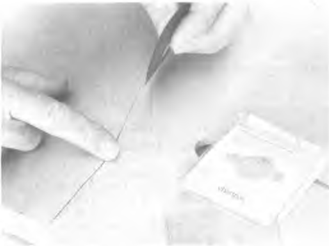
Drafting tape in 1/64 thickness is an easy way to lay down panel lines. Craft and drafting supply stores carry the tape.
