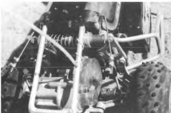
The Fun Racing Product's side bars and rear cage allow easy access to motor and gear box for quick change.
