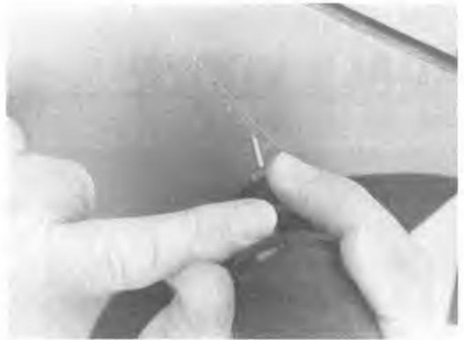
Sharpened steel or brass tube chucked in Dremel tool makes fast work of producing rivet pattern on models of metal covered aircraft. Two hands for beginner or expert!
