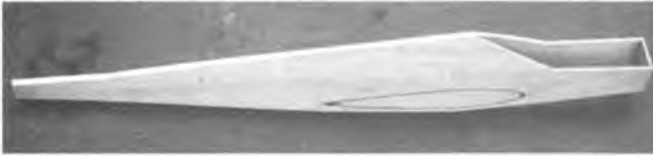
Top view showing wing cut-out outline.
