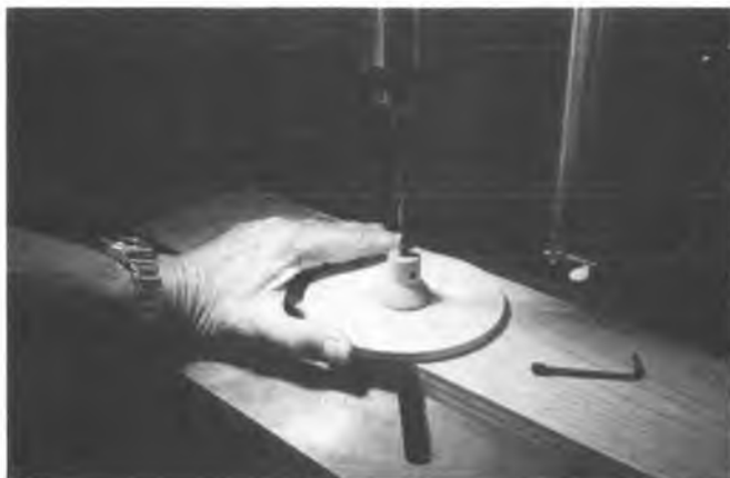
Drilling Spool & Disc: use drill press for accuracy. Note previously drilled and tapped set screw hole.
