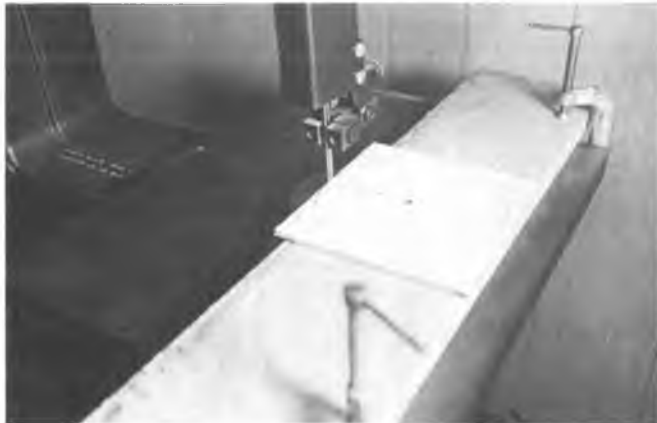
Bandsaw Jig: Note compass pencil line at edge of ply, and radial line at front edge of blade.
