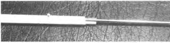
Fiberglass arrow shaft pushrod described in text. Wire extension is motorcycle spoke and is blocked in place with hardwood dowel. Makes strong and dependable pushrods for large models. Dotted line indicates depth of dowel plug.
