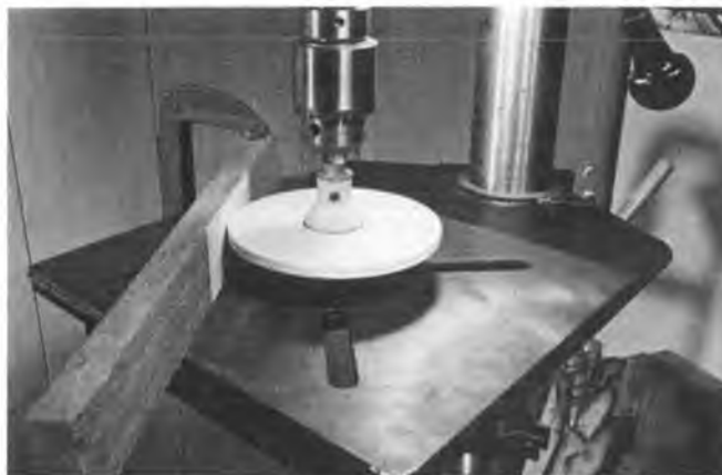
Jig For Edge Sanding: Lightly pressing unclamped end of 1 x 2 against spinning disc gives true 5" diameter.
