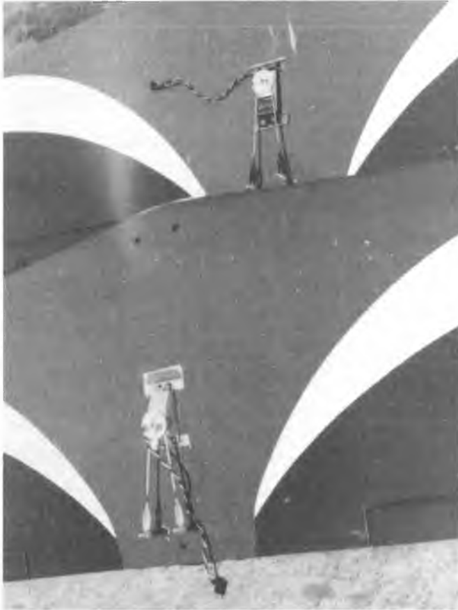
Aileron servo installation, can you tell the built-up from foam?
