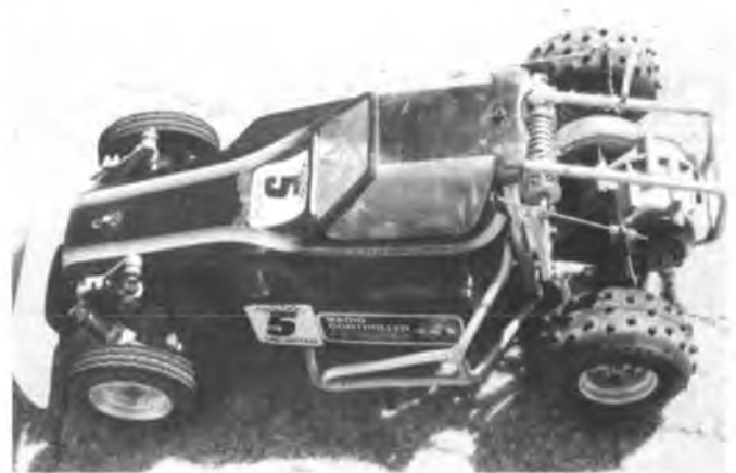
Side bars and rear cage not only look good but offer a lot of protection.
