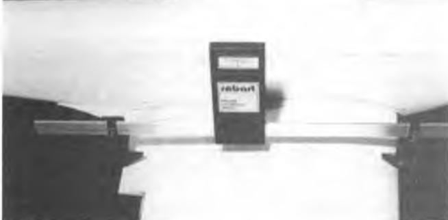
Checking wing incidence.
