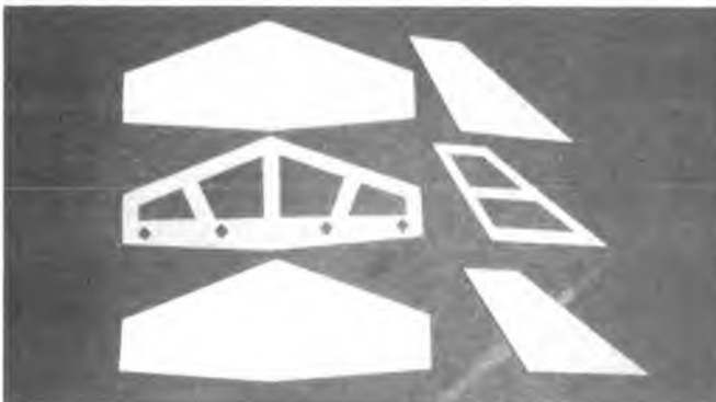
Empennage parts ready for assembly. The Klett hinges were cut off to match the slots shown in the stabilizer.
