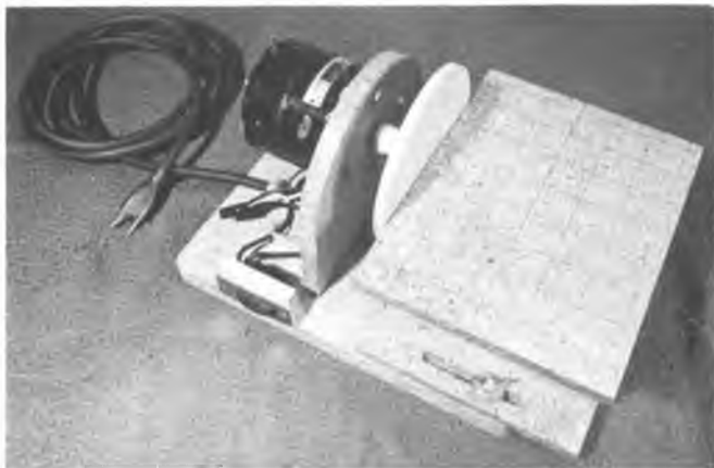
Completed Sander: Small tubes on top of motor are for light machine oil to bearings.
