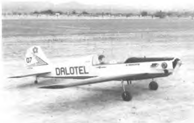
The winning ship. Hanno Prettnr's "Dalotel," powered by twin geared S.T. .75's.
