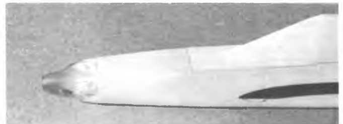
Fuselage nose sanded and shaped into engine mount.
