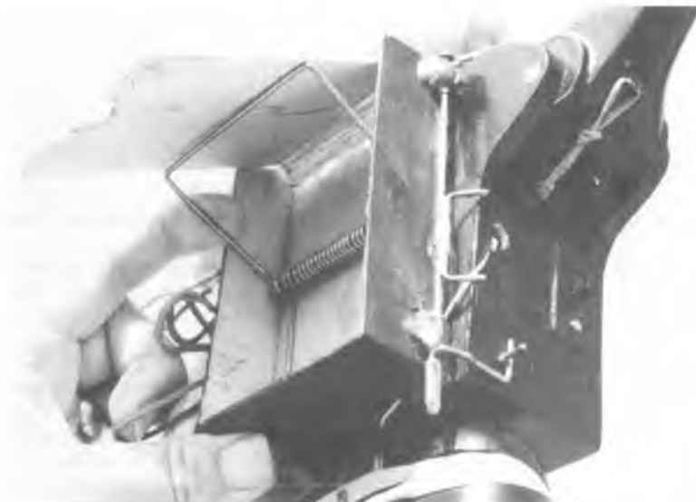
Close-up of the "mouse trap" like spring and hinged flap which flip the emergency chute out of its pack. The rotating hooks and the push-pull pin which hold (and release) the emergency chute are clearly visible here.
