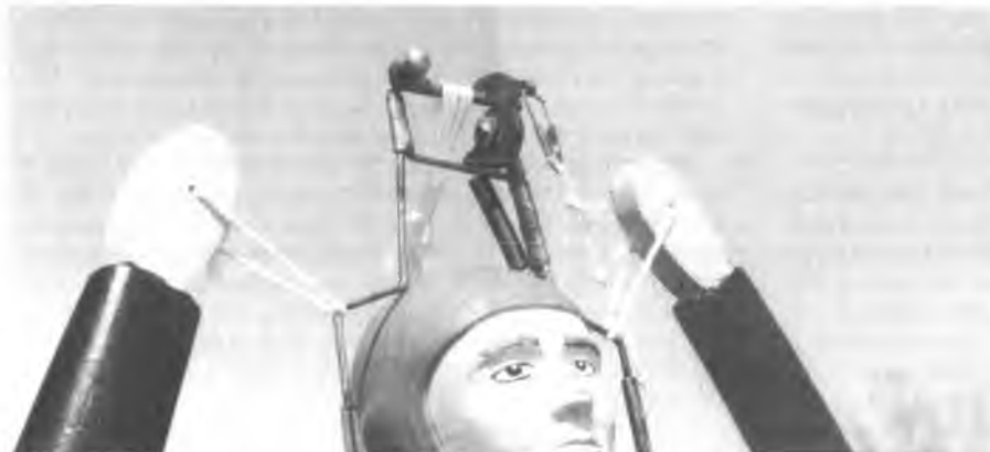
Close-up of the main chute release mechanism. The servo pulls the string which rotates the spring-loaded hook . . . allowing the rotating pin to rotate upward and release the main chute shroud lines.
