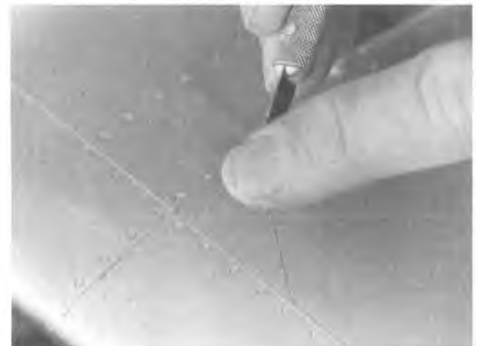
Final step after color coats are on is to remove panel line tape. End result is a fine groove in the surface that simulates the butt joint of flush aluminum panels.
