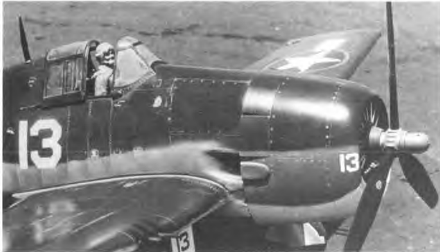
Bob Walter used panel line and rivet techniques described by Art when he built his F6F Hellcat. Hellcat has combination of flush rivets, flush Dzus fasteners and round head rivets.
