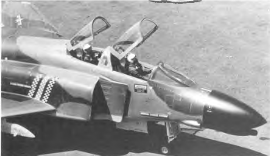
Hot tube system produced nice flush rivet pattern on Tom Cook's new F4E ducted fan model. Photo at U.S. Scalemasters Championship contest.
