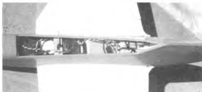
KPS-18 servos side-by-side with KPR-7L receiver and Motorola batteries --- all in the wing.
