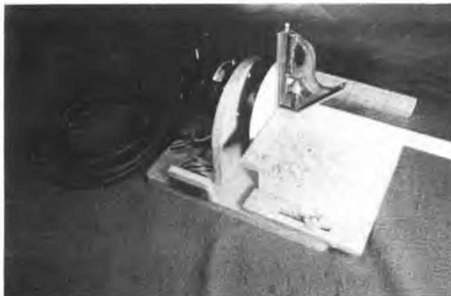
Checking table to disc for 90°.
