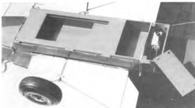
An upside down view of the drop plane's underside, showing the tray in position. An access hatch has been opened to show the tray servo. The rotating hooks and push-pull pin are clearly visible.
