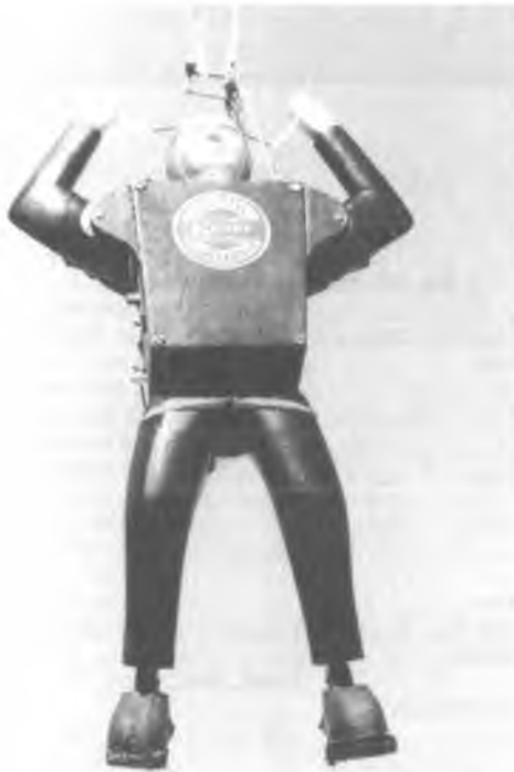
Dan suspended from his main chute. The main chute shroud lines attach to the rotating pin on the harness above his head.
