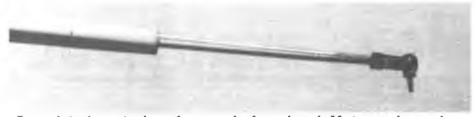
Completed control surface end of pushrod. Motorcycle spokes are threaded with 4-40 thread to fit large Du-Bro ball links making very substantial pushrods.
