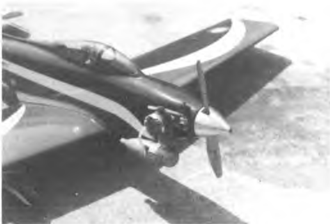
OS .61FSR installation, note wheel pants.
