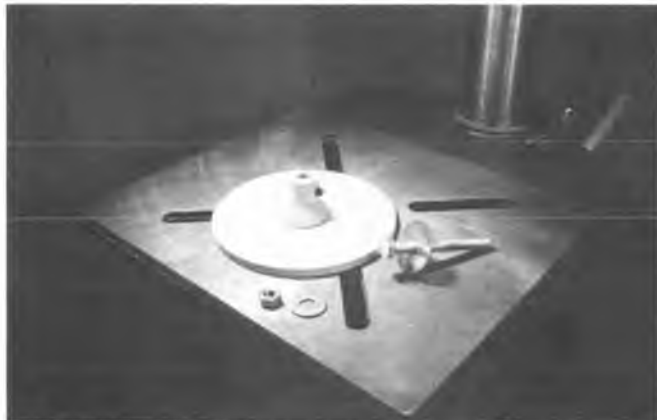
Bolt, Nut & Washers: Used to mount disc in drill press for edge sanding with jig.
