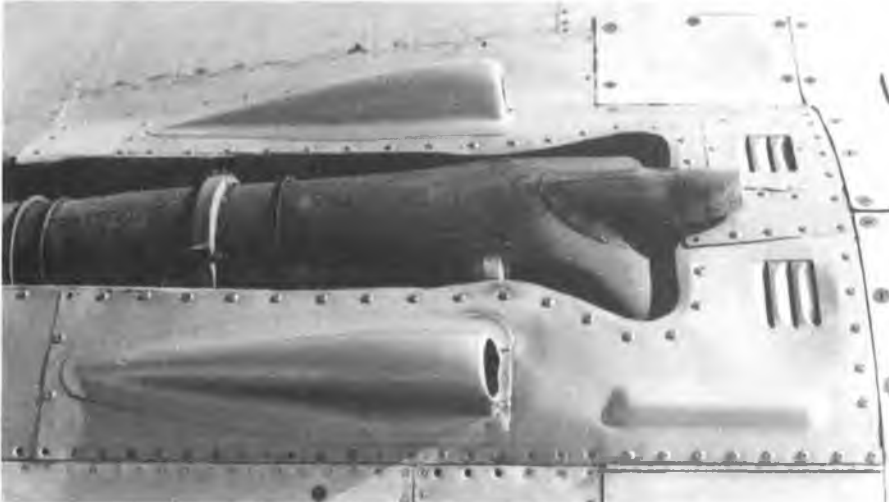
Boom section over wing of P-38 is a study in surface detail variety. Flush, overlapped and hinged panels. Flush rivets, flush cross point screws, round head cross point screws and flush Dzus fasteners all show in photo.
