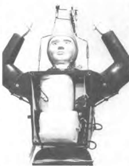
A close-up with the chest access hatch removed. The hatch is held down by four screws. The Rx is located in Dan's upper right chest area, and the main chute release servo is just to Dan's left of the Rx. The 250 ma battery is in his tummy area, with the emergency chute release servo out of sight behind the battery. The rotating pin on the wire harness shows well in this shot.
