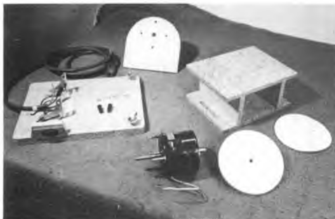
Sub-Assemblies: Note long screws projecting from motor housing used to mount motor.
