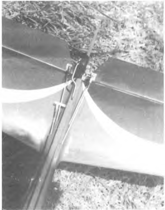
Tail wheel and pushrods, note steering pushrod.
