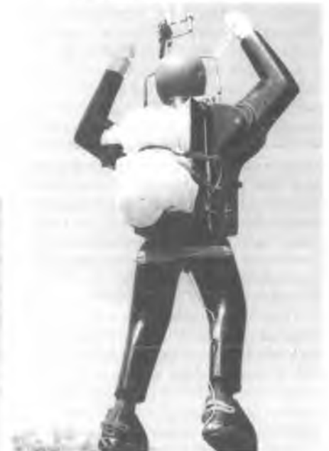
Back view, showing the emergency chute in packed position. The rotating hooks (and the push-pull pin) which hold the rubberbands which hold the emergency chute in its pack are visible. The Rx antenna is on the back of the right leg.
