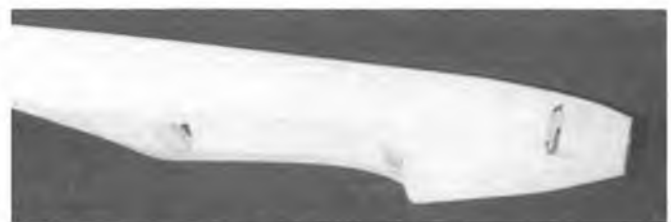
Fuselage carved and sanded to shape.
