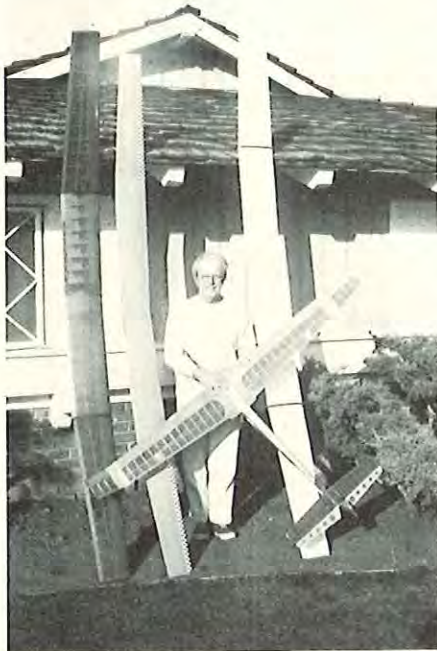
On the left is the 385 wing. Center wing is flat bottomed 385 section. On right is the "laminar" section. Smaller wing on fuselage is Eppler 387. Cirrus wing not shown.
