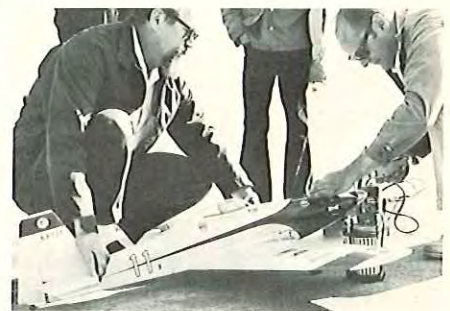
1/4 Midget, left has homemade retracts. F.A.I. Mustang has Goldberg retracts. K & B Super Poxo finish on Paul White's entries.
