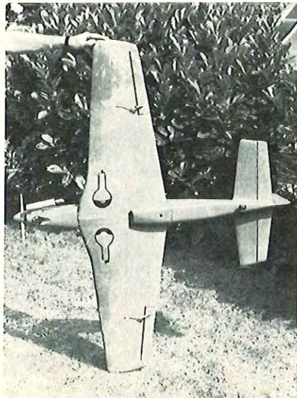
LEFT: Details of KDH retract gear installation on John Evan's Mustang. Non-scale wheel covers allow better streamlining. ABOVE: Photo detail of engine cowl on Evan's Mustang. F.A.I. rules allow engine cylinder protrusion of only 1 cm. from cowl. Arrangement for adequate cooling essential.
