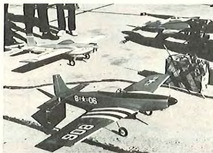
1/4 Midget, left has homemade retracts. F.A.I. Mustang has Goldberg retracts. K & B Super Poxo finish on Paul White's entries.
