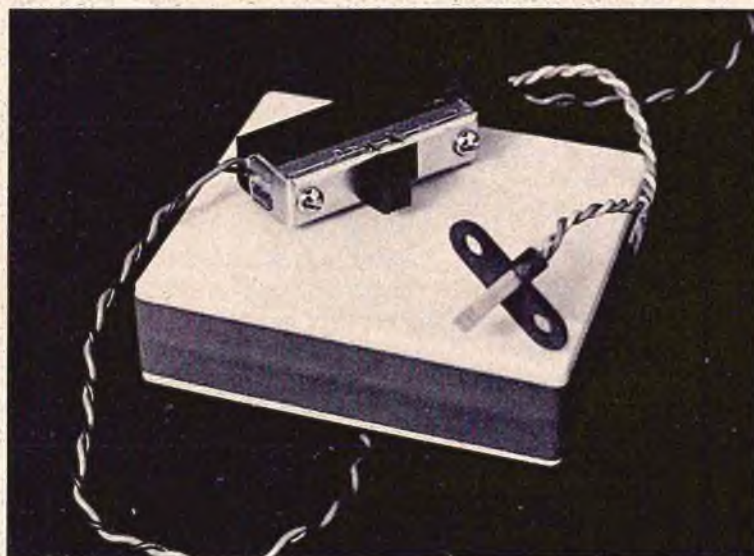
The flat battery pack is rated at 500 MAH and weighs under 4 ounces. Switch harness and charging jack are wired as an integral unit with the battery.
