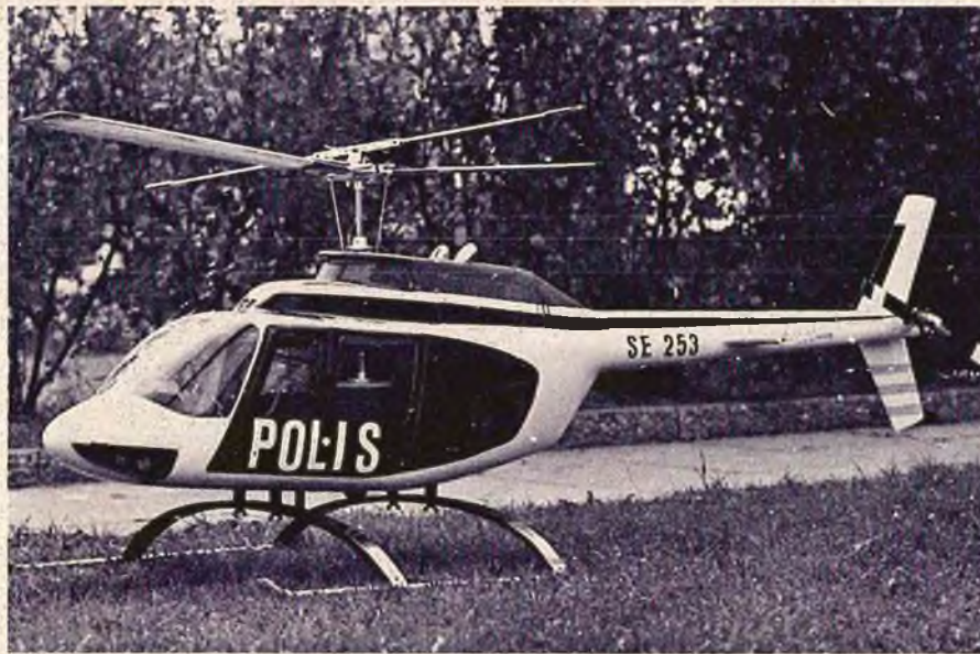
Jan Levenstam's Jet Ranger utilizes a MacGregor radio, Veco .61. Photo from recent Swedish competition.
