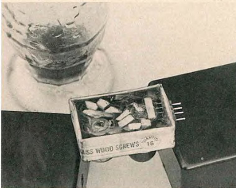
ABOVE: With the wired unit resting level on a pair of boxes, the interior of the box was filled with brimming with Francis Products' surfacing resin. A few chips of balsa were sprinkled into the box first to prevent the resin from cracking as curing occurred. The hardened resin makes the unit ultra sturdy and completely short circuit proof.
