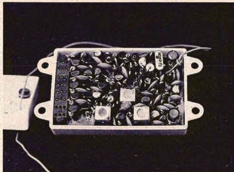
Receiver has exceptional sensitivity due, in part, to the use of an RF amplifier, a very unusual feature for a unit in this price range.
