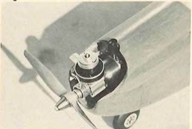
This is a view of the muffled Cox .049 installed in the nose. The spring starters are a big help in getting the engines started.
