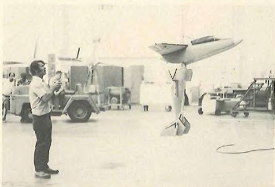
Nick Zirola flying the Nutcracker in the vertical mode. The model is flown suspended by a tether approximately 30 feet long. In case of loss of control, or an engine failure, the tether keeps the model from getting away or hitting the floor.
