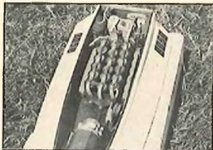
American 'Sea Ram' on 2:1 gear mount. Water cooled nicad cells. 22" length, runs at around 600 watts.
