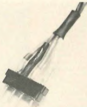
Feedback wire is the dark wire that is added to your servo.
