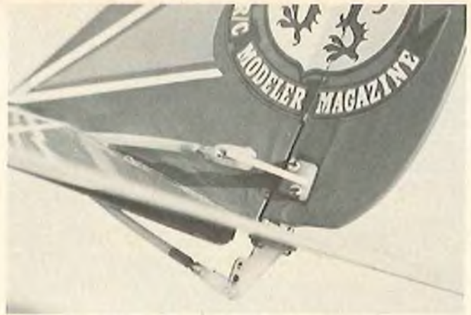
The other end of the Gold'N-Rod pushrods showing the rudder and elevator linkages.
