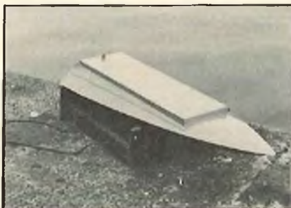
Dave Wooley's electric 'Bullet 30'. 500 watts, speed around 30 mph with hydro type hull, speed of over 40 mph possible.
