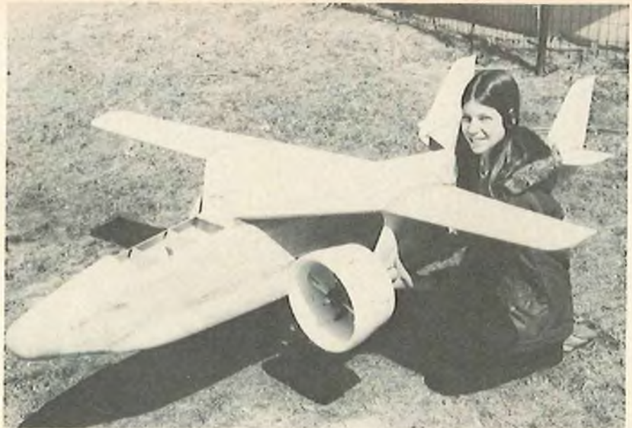
The Nutcracker uses typical model airplane construction techniques. Foam and balsa wing and tail surfaces have proved to be ideal. Sheet balsa over formers have produced light, rugged fuselages. Light fiberglass cloth and resin is used over most of model.
