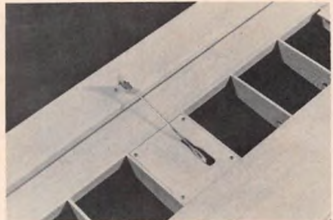
Installation as viewed from bottom. Aileron adjustment is easily accomplished by removing keeper from control horn and rotating wire. Threads in clevis can readily be seen at all times with nothing hidden.
