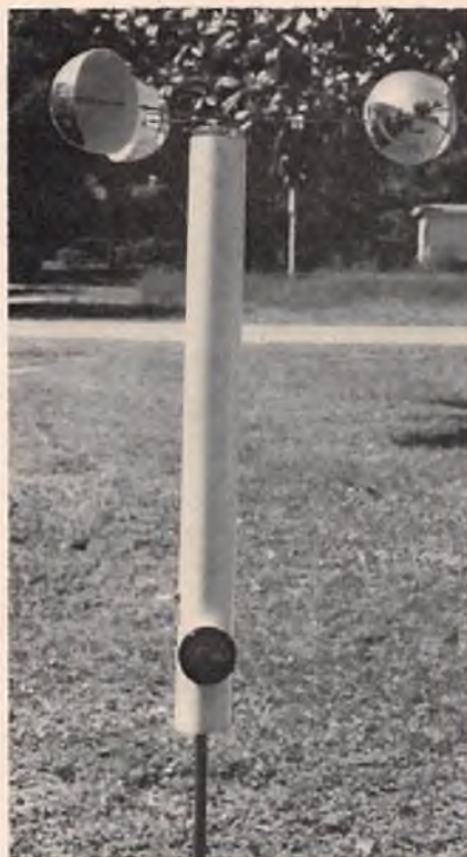
Anemometer stuck on a pole ready to go to work. Most any type mounting will work as long as it's sturdy and you can read meter.
