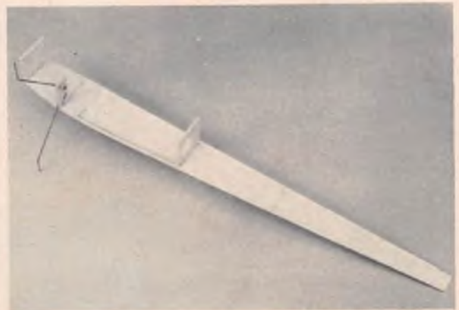
Formers installed to right fuselage side – use small triangle or square to align properly.
