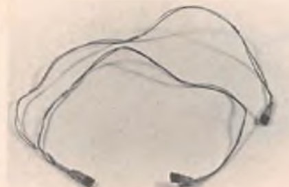
Special "Y" cable required to hook up servos mounted outboard in wing. Take extra care to observe polarity.
