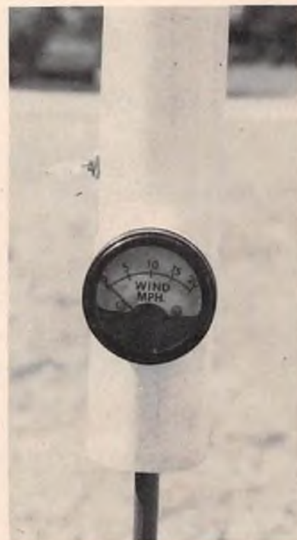
This is the meter. Switch is for low speed/high speed. If conditions are super windy, just flip switch and double numbers.
