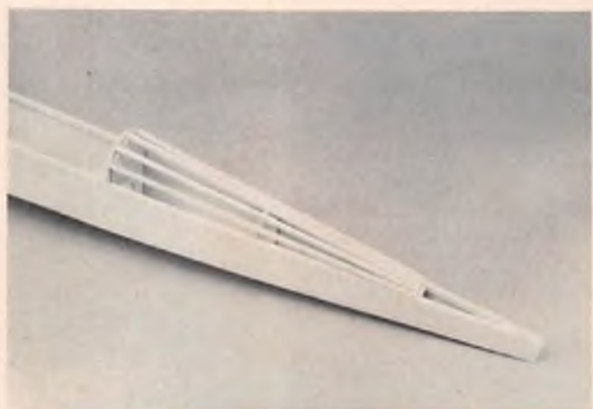
Rear of fuselage completed with formers F-5A, 5B & 6 in place and stringers installed.
