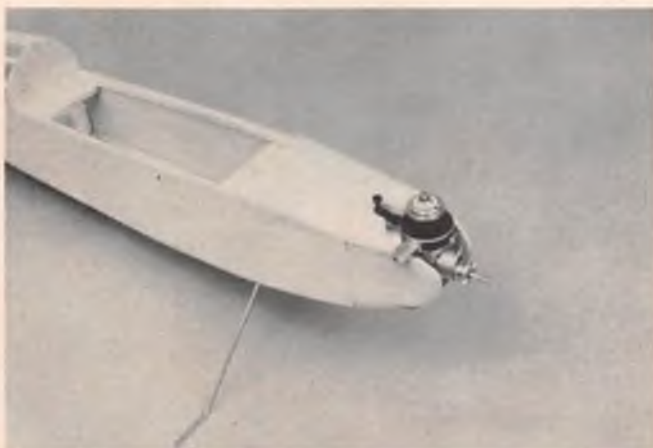
Engine installed and nose blocks glued in place and sanded to shape.
