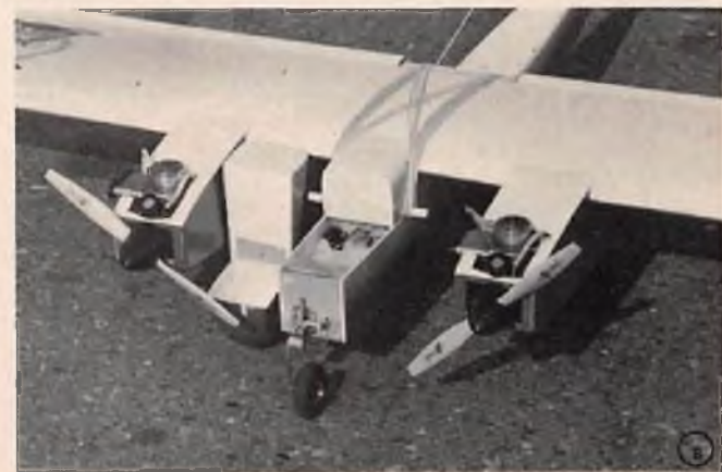
(1) Framed up engine nacelles ready for installation on wing. (2) Bottom view of wing center section showing throttle servo & linkage. (3) Forward fuselage section showing removable foam nose block. (4) Completed fuselage ready for covering. (5) Completed twin ready for final covering & equipment installation. (6) Completed wing with throttle & aileron servos installed. (7) Rudder & elevator servos installed showing ample room for even the largest of equipment. (8) Nose block removed giving good access to receiver & battery pack. This allows easy adjustment to nose wheel tiller arm.
