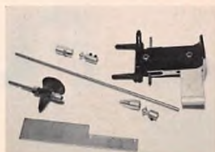
The break-down of all the parts in a parallel drive system: engine coupling, main shaft, underwater coupling, parallel shaft, skeg and rudder strut.
