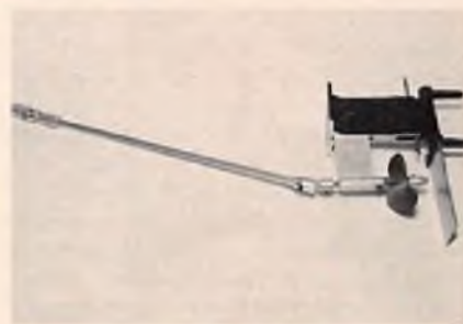
The parallel drive with all the parts in place, as they would be in a boat.
