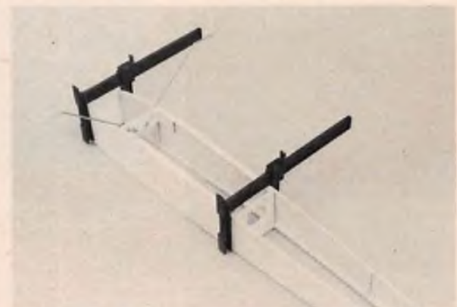
Using model clamps to hold securely, join two sides.
