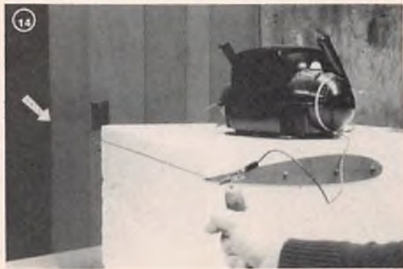
Cutting the tapered wing – the nail is 70" from, and level with, the root template.
