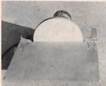
Note hinges inset in table top for flush surface.
