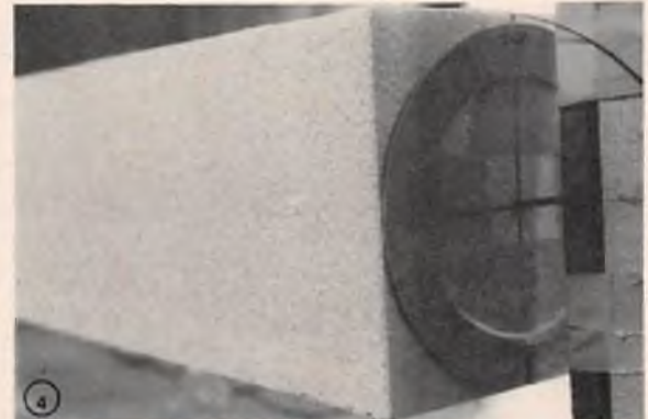
Set up to rotate fuselage block on nails.
