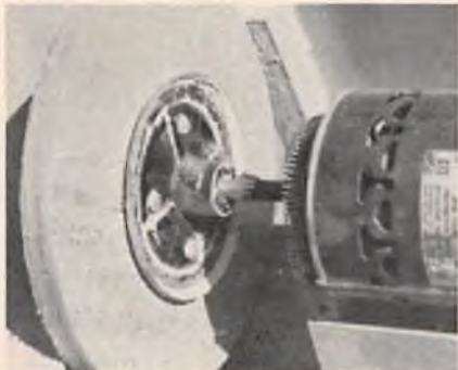
Close-up of adapter made from cut down squirrel cage blower with vanes removed.
