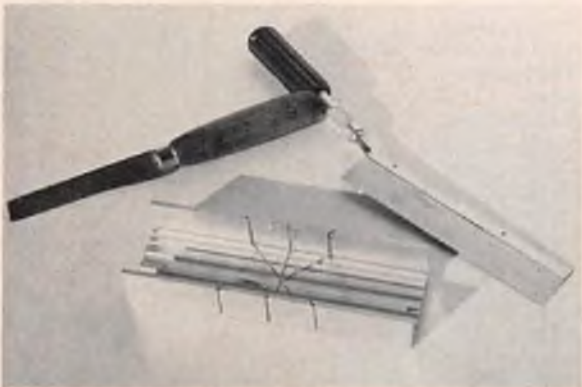
ABOVE, L to R: Cork knife, miter box and X-Acto saw. RIGHT: Top is a Stanley plane - L to R: 3/32" screwdriver, screw starter, 1/8" x 4" screwdriver and long nose wire pliers. BELOW: RCM epoxy mixer Mod. II with mixing sticks. 5 min. epoxy tubes held in a baby food jar. BELOW, RIGHT: Top is a 1/2 size miter saw with X-Acto razor saw on bottom.
