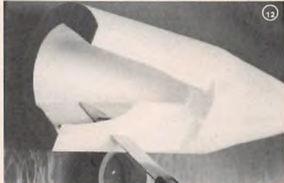
Trimming wing saddle on rear half of fuse.
