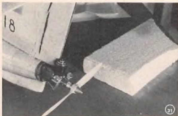
Good TD .051 and 6/3 pusher prop on a tank mount.
