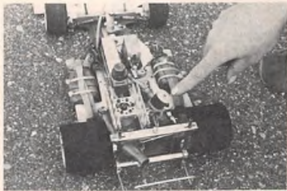
Roger Berquist's carb. air filter (see text), chassis is Delta Super J powered by Dye modified K & B .21.
