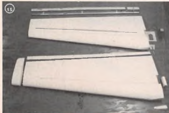
(Front of picture): Pieces cut off to fit plan. (Back): Pieces of wood to be glued for finished wing.
