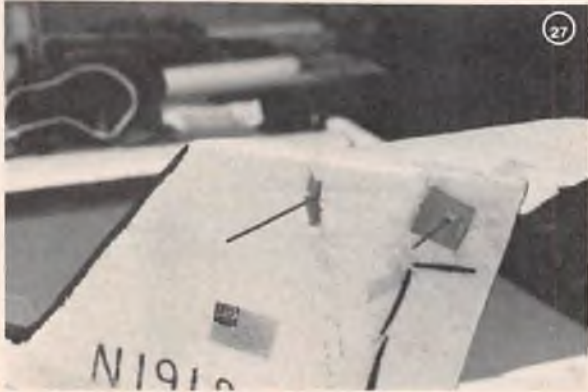
Close-up of tail fin with 1/16" wire set up for flying stab.
