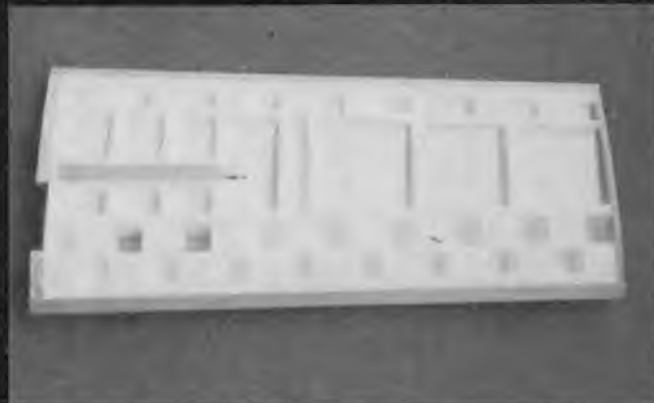
Sullivan foam wing ready for sheeting.
