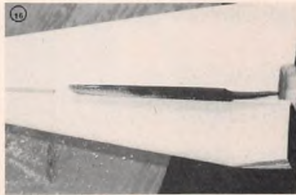
Cutting groove for spruce spar.
