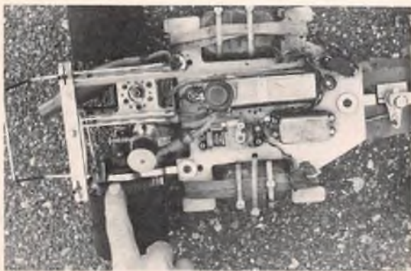
Disk brake on Roger's car --- this machine took 3rd in '78 Formula I U.S. Championships.
