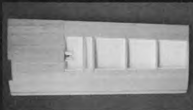
Sheeting and capstrips added to Sullivan foam wing. Plans also show a built-up wing.
