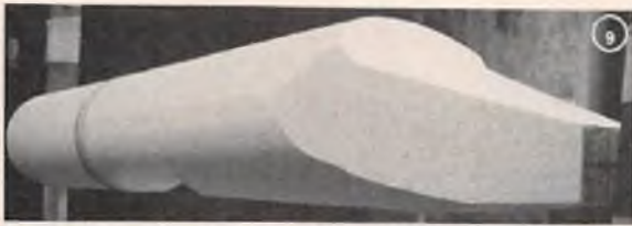
Ready to rotate fuselage to cut off center tail cone.
