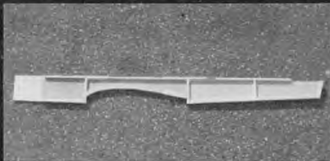
Fuselage side complete with nylon wing hold-down bracket attached.
