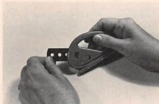
Blade changing is a snap. Any standard double edge razor blade will do.
