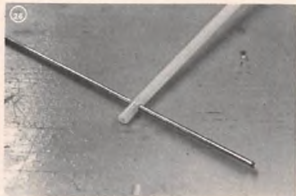
Inner NyRod with 1/16" wire (flown one year without any signs of wear and no problems).
