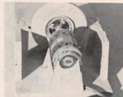
View showing spring hold-down clamps for motor.
