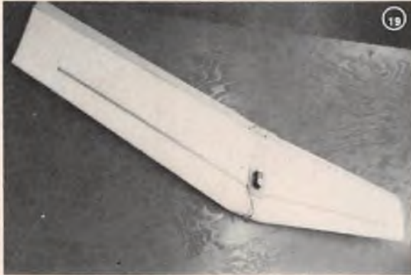
Finished wing with ailerons, servo tray, servo, and center fiberglass (with Hobbypro II glue).
