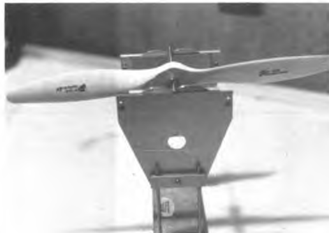
Legs can be extended to allow large props to swing through.
