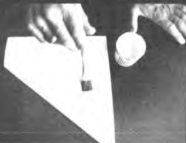
Apply 50-50 allphatic resin/water mixture — let dry and apply second coat.
