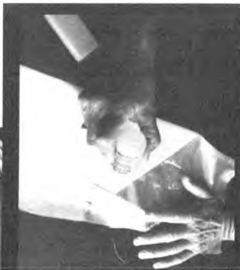
Tack cloth at trailing edge of wing, pull tight, tack at leading edge, pull to trailing edge and tack again.
