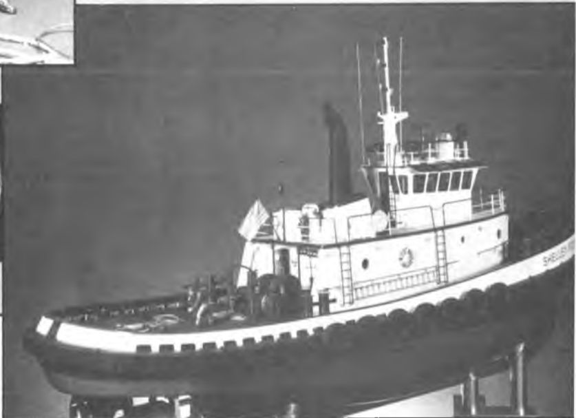
View of starboard side showing position of ladders, railings and other components.
