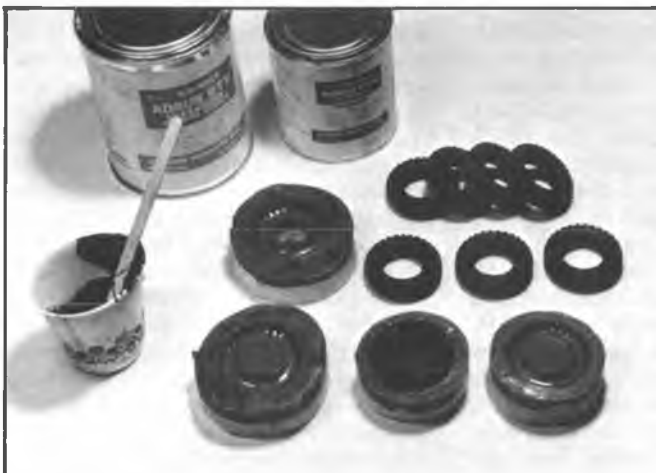
The manufacturing of rubber bumper tires using Abrub RTV molding rubber.
