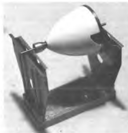
Spinners and backplates are easy to balance, High Point instructions tell you how.
