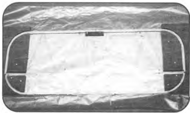
Plywood jig used to form the double pieces of 1/8" x 3/16" spruce in the stab, elevator, fin and rudder.
