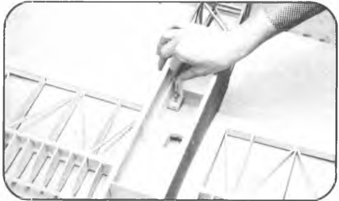
An easy method of marking the spots for drilling the 1/4" holes for the nylon 1/4 x 20 wing hold-down screws.
