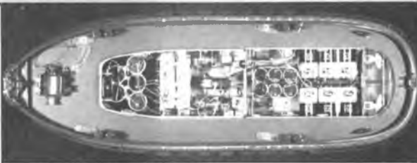
Placement of power plant in hull.
