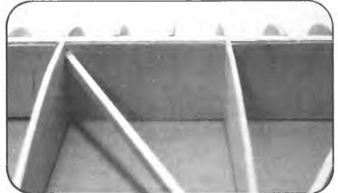
Webbing for main spars is 1/16" vertical grain balsa butted against rear of main spars. Diagonal braces are 1/8" x 3/16" spruce.
