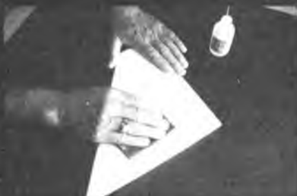
Sanding the glassed and primed surface.
