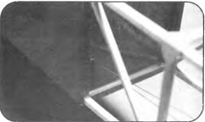
Control cables shown exiting the fuselage. Note that both cables exit through the same piece of Inner Gold'N-Rod.
