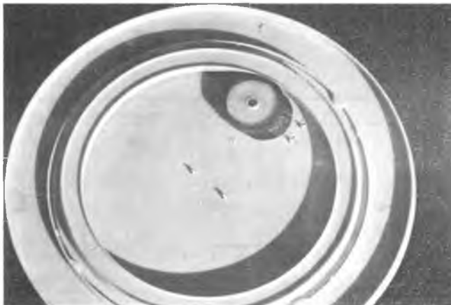
Bottom view of training table showing yaw servo wheel.
