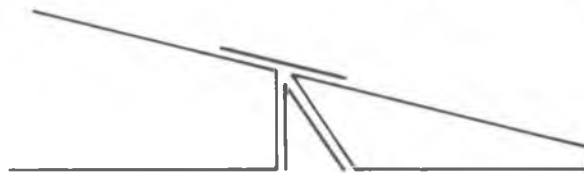
MONOKOTE HINGE AS USED ON THE LAZY ACE
