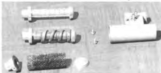
Exploded Fox muffler showing the different modification explained in text. (Top): Standard Fox core. (Middle): Core wrapped with screen and tube for internal preheater. (Bottom): Core cut to allow muffler to accept more screen, an external preheater must be used with this type of modification.
