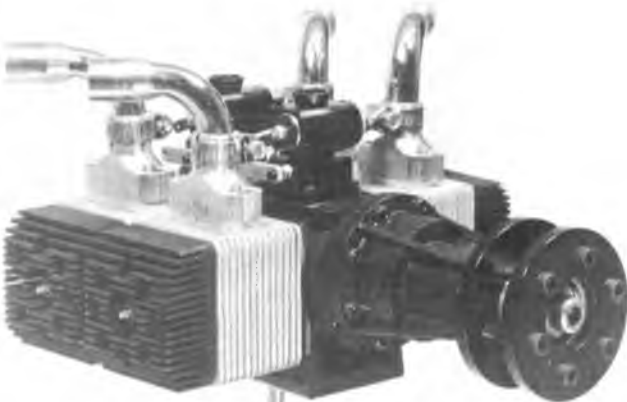
The horizontal four with black anodized parts, exhaust headers, Perry carbs and 2.055:1 reduction gear drive.
