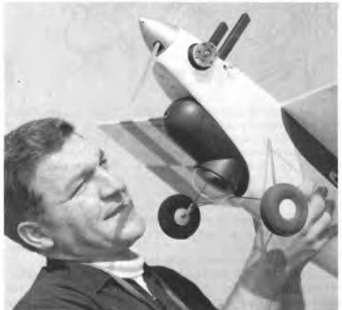
The Ross Twin was used by Jan Sakert and Dick Riggs in a 1/2 size version of the first RPV project to use off-shelf model hardware.
