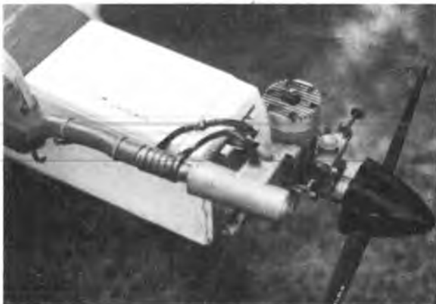
Complete installation using the external preheater.
