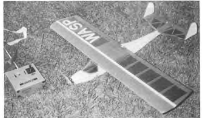
The Wasp is designed for use with any of the 05 sized motors available today using 6, 7, or 8 cells of 1.2 AH capacity for long pleasing sport flying.
