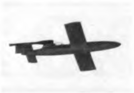
Joerg Vogelsang's manned V-1 model. At Quarter Scale, model was noisy, fast, and impressive. Was clocked at 262 mph and flew very well.
