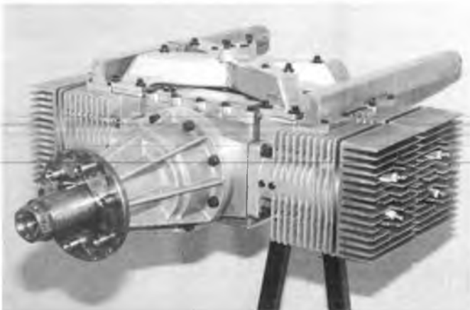
The model R-1 is a four cylinder, two cycle, horizontally opposed engine of 1000cc (61 cu. in.) displacement. Weight is 127 lbs. and delivers from 75 to 95 horsepower.
