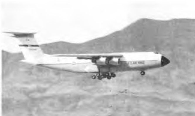
Full scale or model? Hard to tell in this photo. Model was capably flown by German modelers. C-5A equipped with operating flaps and spoilers. Note flaps partially deployed.
