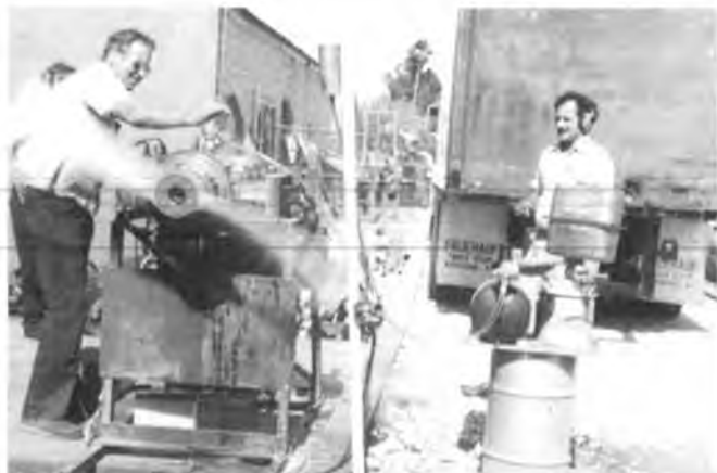
The model R-1 on test stand can be operated on diesel fuel, gasoline or natural gas.
