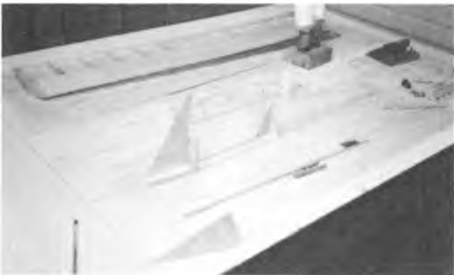
Fuselage formers F-4 and F-7 epoxied in place. Make sure they are perpendicular.
