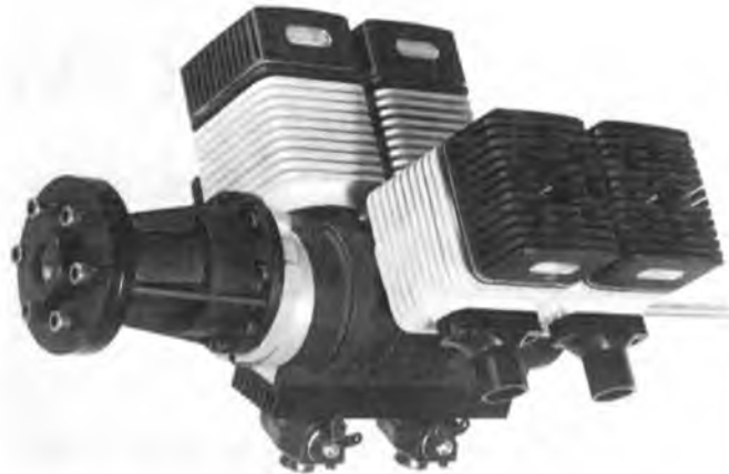
The 90° V four has displacement of 2.66 cu. in. (3.972 cu. in. to be available soon) and comes with either a direct drive or with 2.055:1 reduction gear drive as shown here.
