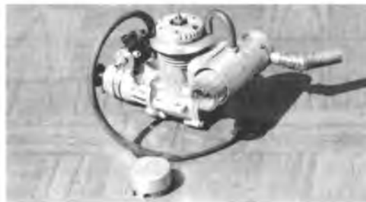
K & B 40 outfitted with boat type preheater and screen in the muffler (probably the best of all the smoking 40's).
