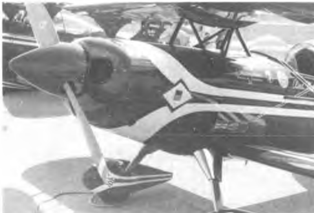
Note the "Q" tip on Clint McHenry's prop. Tip is intentionally formed back to reduce noise.
