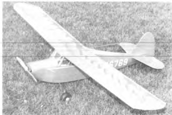
Jim Zaremski's Porterfield with SR 16 cell 900 mA battery pack. Flight duration up to 8 minutes with little increase in weight.
