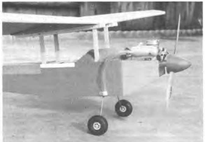
Putt 'N Paul with cable clamp holding exhaust tube.
