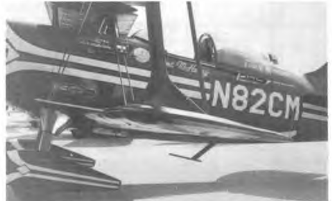
"Spade," aerodynamic booster on aileron of Clint McHenry's Pitts. Everyone used them.
