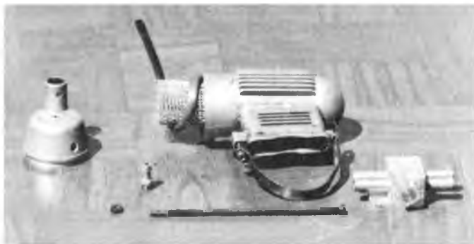
Exploded view of O.S. muffler showing preheater tube and screen along with a home-made high volume smoking valve. (Note tube exits muffler through hole drilled in edge of stinger housing.)
