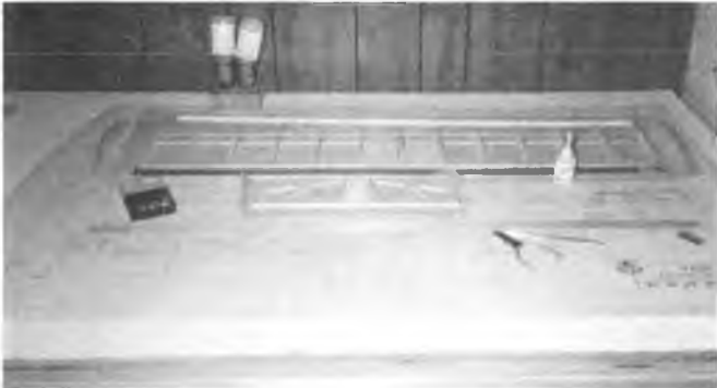
Wing and stab framed. This takes less than one hour using Super Jet.
