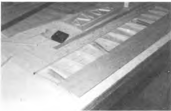
Leading edge cemented to top spar with cyanoacrylate. Clothespins used to secure during cure time.
