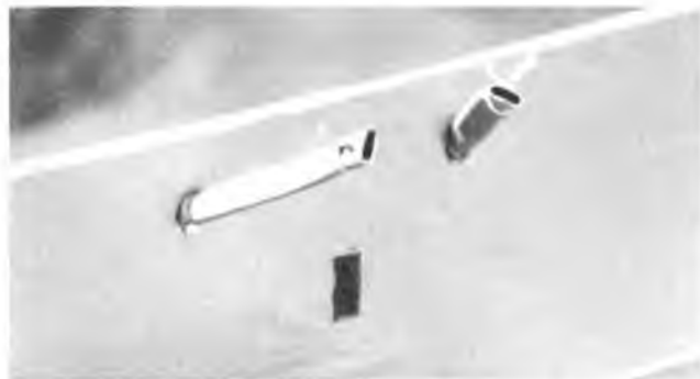
The underside of the first set of wing used with K & B twin exhaust. (Note: No "T" is necessary with the twin exhaust.)
