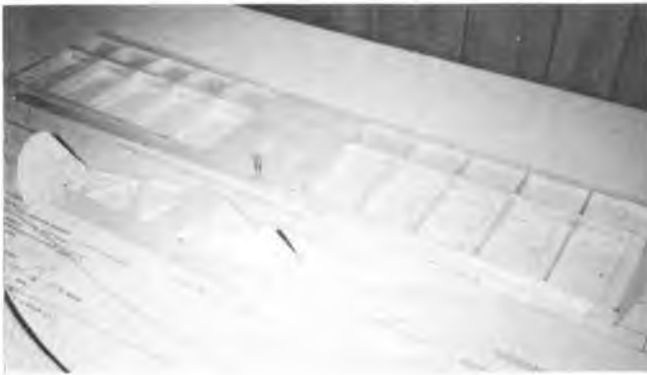
Wing and stab ready to cover. Wing requires fiberglass reinforcement around wing hold-down dowel and nylon hold-down bolt area.
