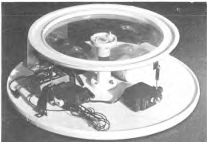
Completed training table minus top plates. Prototype used track portion which is not necessary.
