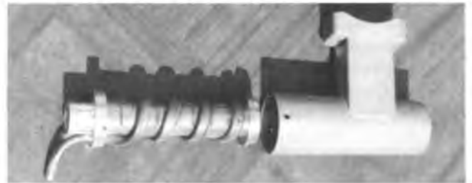
Exploded view of Fox muffler with an internal preheater. Note screen around aluminum core and one of the four or five holes drilled in the end of the copper tube.
