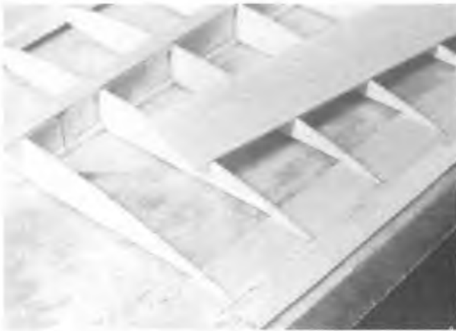
Fiberglass tape spot glued with CA prior to epoxy for top surface. Note 1/16" x 1/4" support under center of trailing edge — will preform lower surface curve.
