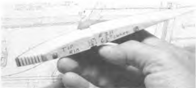
Tip ribs showing leading and trailing edge squared off before removing from templates.
