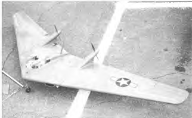
This Northrop N9M-A by Bill Young was powered by twin electric motors and features retracts.
