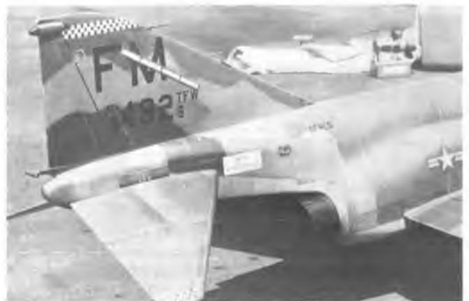
The business end of Tom Cook's 1983 National Champion Sportscale model of the F-4 Phantom. Tail cone opens to release drag chute — afterburner nozzle in full power open position.
