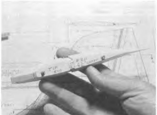
Set of tip ribs after shaping. Note bevel on outside edge of tip template only.
