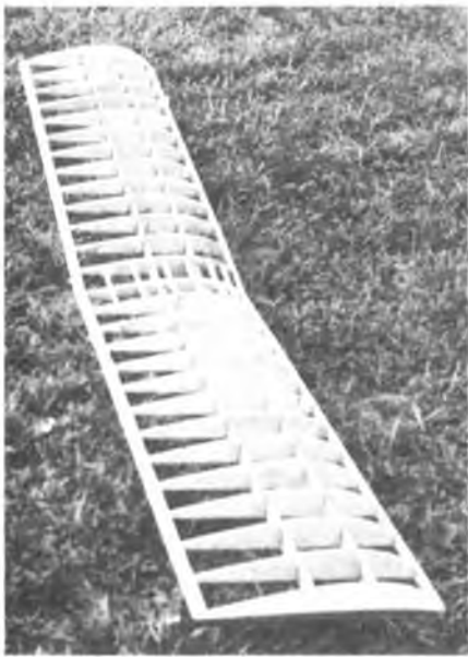
Completed wing ready to cover.
