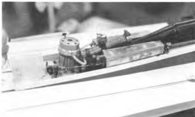
(7) Engine installation in the tunnel hull.
