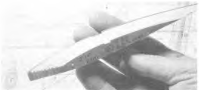
Ribs after separating from template and squaring off top and bottom edges should be very uniform when restacked.
