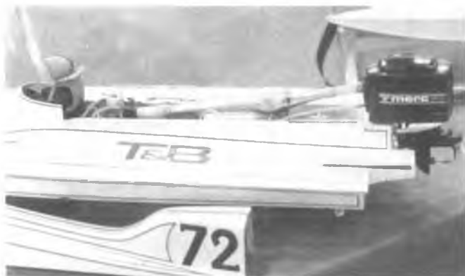
(9) This one has a K & B 6.5 marine engine mounted inboard.
