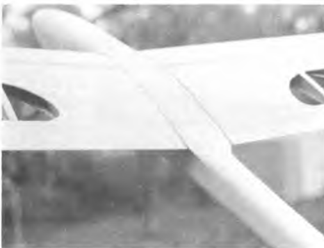
Wing and fuselage mating showing fillet contours.
