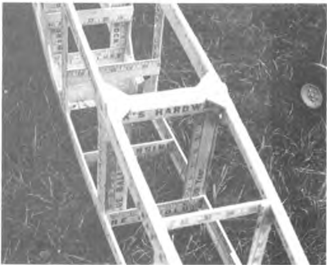
Fuselage at wing trailing edge showing gussets and cross pieces for radio tray.
