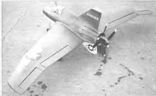
Bill Young also built this Northrop XP 56. Electric power with contra rotating props.
