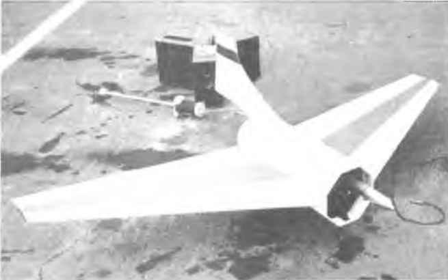
Who says modelers aren't ingenious? Clay Soule powered his wing with a Byrojet ducted fan unit.
