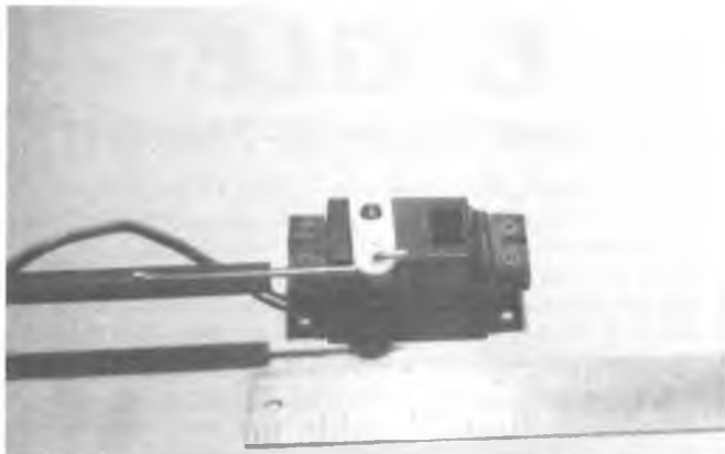
Airtronics servo used in author's Der Jaeger. Note the large arm permitting use of motorcycle spoke as connection between carbon fiber arrow shaft and servo arm. The heavier arm permits drilling a hole large enough to accommodate the spoke without weakening the arm excessively.
