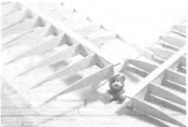
Lower trailing edge tapers to fine edge. Wing box ready for addition of tubing.
