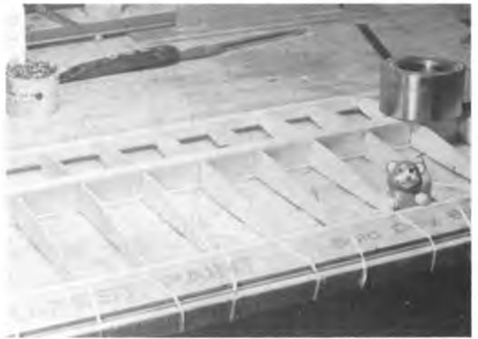
Rubber bands and yardstick apply good pressure to trailing edge while epoxy sets up and will guarantee a straight trailing edge. Upper surface then sanded to fiberglass and epoxy for a sharp trailing edge.
