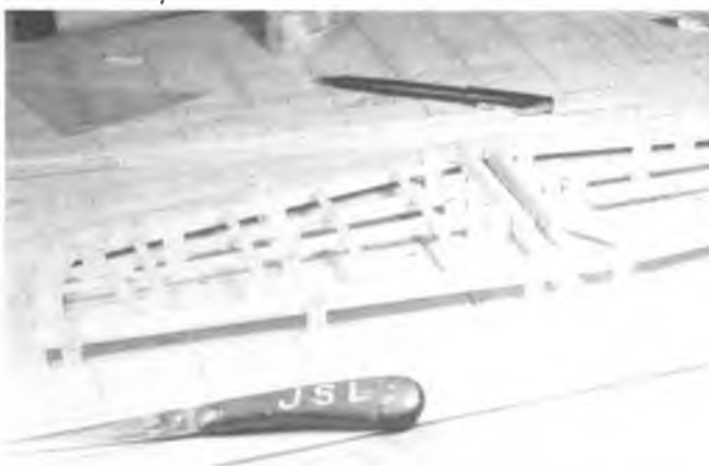
Horizontal stab framed up on jigs. Centerline of stab is positioned 1 2\"/>
