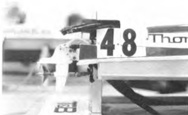
(8) Homemade outdrive system on tunnel hull.
