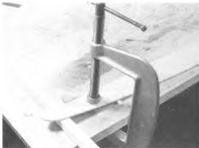
Prebending forward fuselage sides before gluing on triangles will hold curve and make forward assembly easy. Note bulkhead locations premarked.
