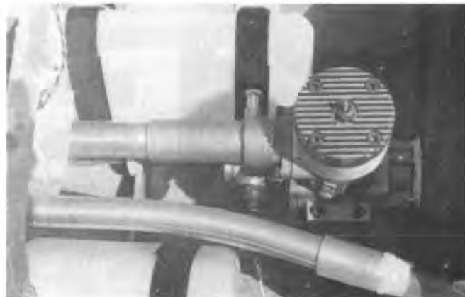
Velcro straps make installation and removal of saddle tanks in a ducted fan model easy. Straps go around tank and are glued to fuselage side. Vibration proof but easy to separate.
