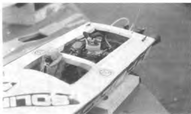
(10) Five foot boat with 45cc chain saw engine.
