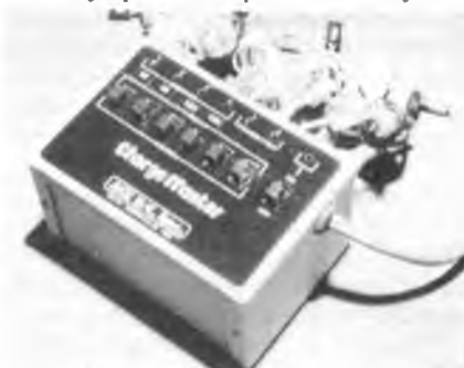
Ace R/C Inc. makes this multi-charger either in kit or assembled form. Provides charging for four RX batteries and two TX from one source. RX charge connections are marked with charge rate to prevent overcharging the wrong battery and connectors can be arranged to suit your own needs. (Note one TX connector for EK and one for Airtronics.)
