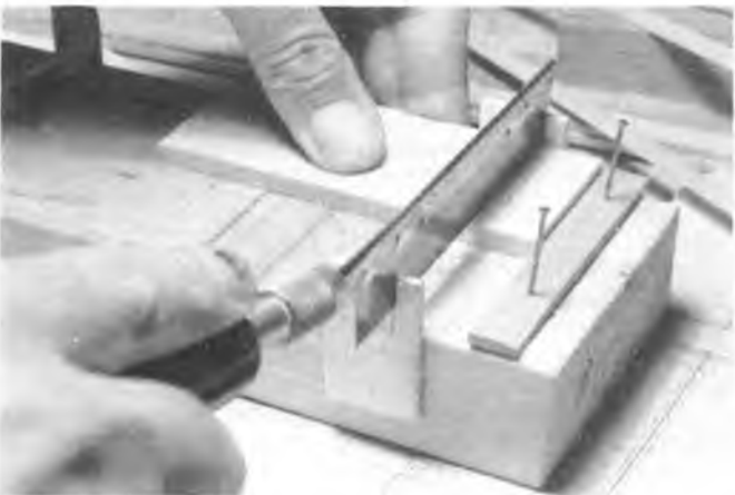
Jig made from 2 x 4 for cutting shear webs.
