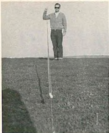
Technique: Hi-start with metal stake and ¼" flat rubber, unstretched. More line to be added. The hi-start parachute is rigged so that chute is kept closed until the glider is released. The parachute opens to keep line from snarling and to mark spot where ring landed.
