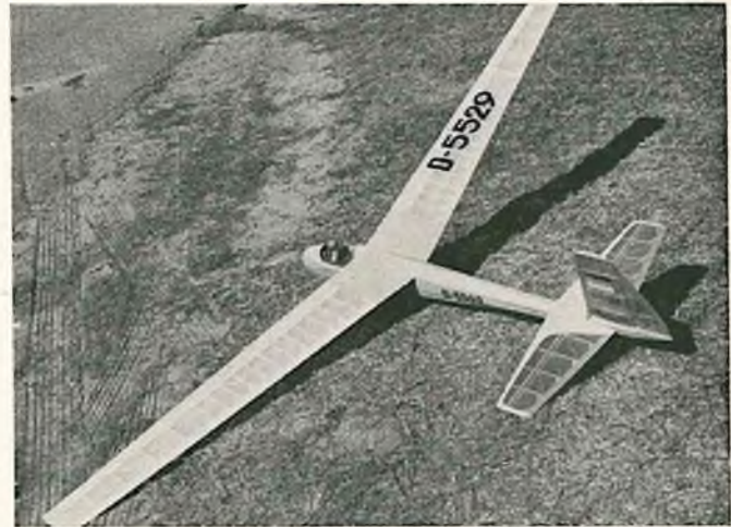
Type: Scale K-7 for rudder only, thermal capability with lightweight R/C rig.
