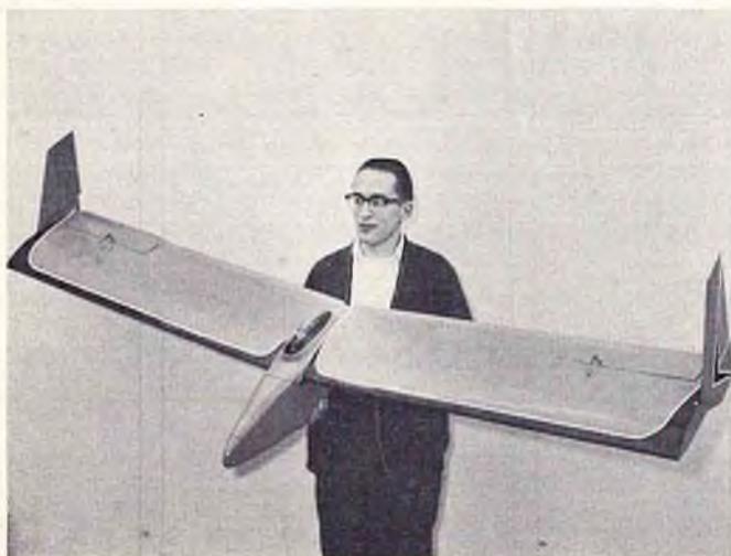
Type: Flying wing glider (plank style) with elevons and rudder. R/C equipment in pod.
