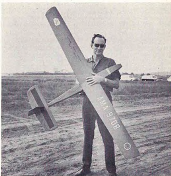
Type: Styrofoam and balsa wing, fuselage and stab, with balsa rudder. Light and strong.
