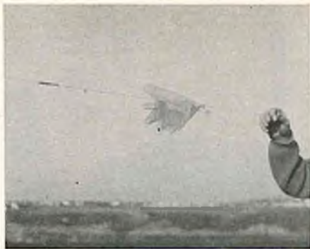
Technique: Hi-start with metal stake and ¼" flat rubber, unstretched. More line to be added. The hi-start parachute is rigged so that chute is kept closed until the glider is released. The parachute opens to keep line from snarling and to mark spot where ring landed.
