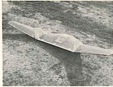
Type: Dihedralled and swept flying wing with rig in center section. Needs more vertical area.
