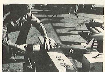
Tony Brown, Conejo R/C modelers, with entry built from RCM plans. K & B .40 FR, MonoKote, 4 lbs., Kraft radio.
