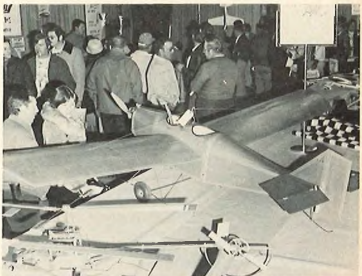
Airplane covered with nothing but cardboard. Designed by Dave Gray, these big machines fly beautifully - - - use gear reduction.
