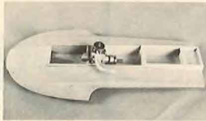
The Hughey Hydro 50 with a Webra Speed .60 engine installed. The engine has a Stidwill Special cylinder head and an ED AMC carb.
