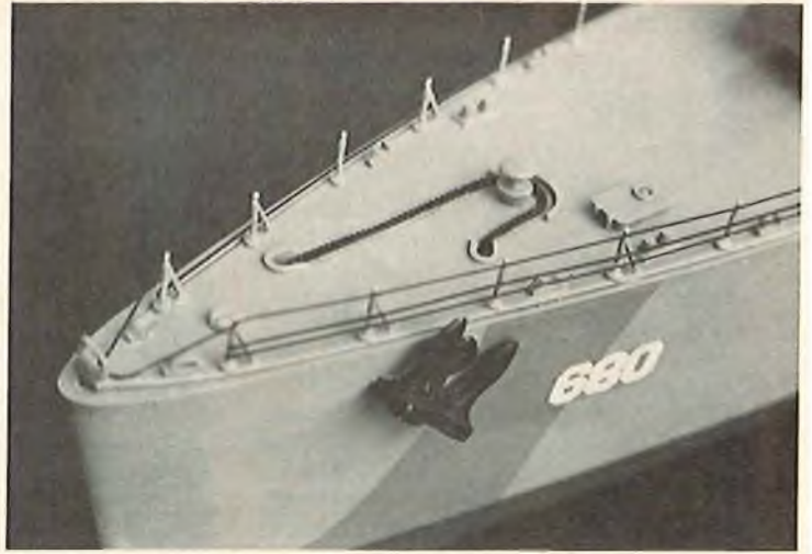
A view of the foredeck. Note bow hold-down screw, anchor chain painted and glued; seal off original switch slot with scrap plastic and cement.
