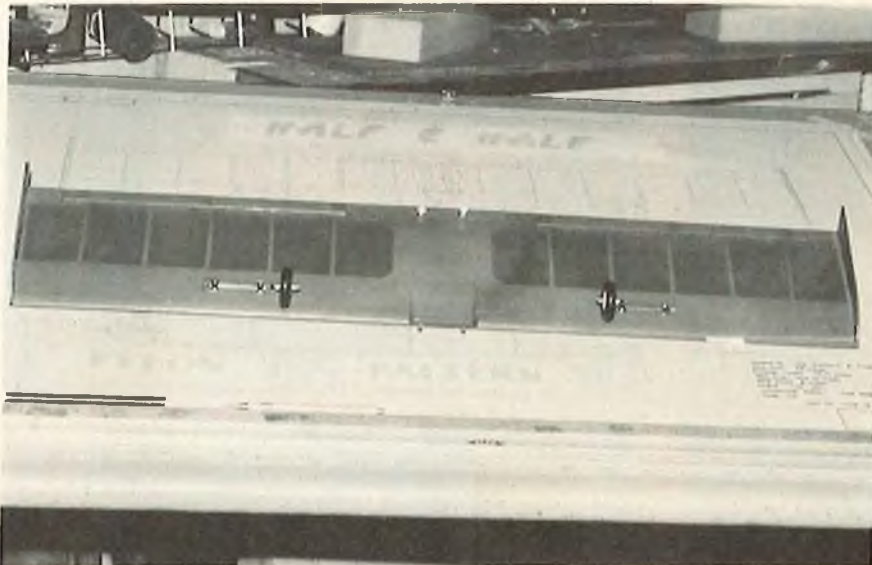
ABOVE: The completed Half & Half wing with landing gear installed. BELOW: A close-up of the gear mount.
