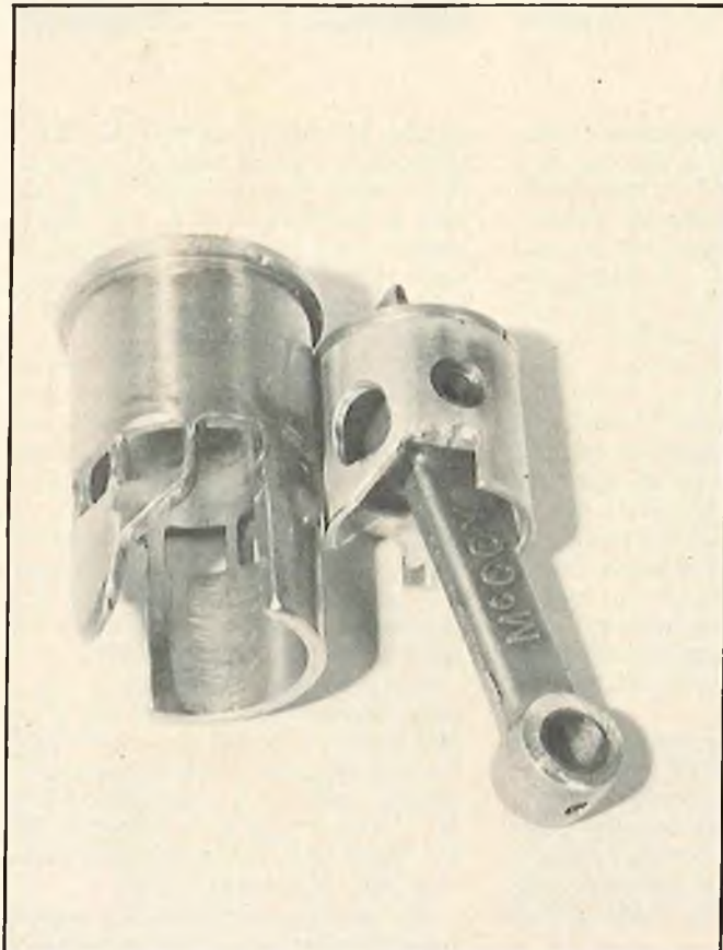
"Semi-Schneurle" Veco-McCoy type engine used by Gene Husting to win both Summer and Winter 1975 So. Calif. Series. Intake port has been added between original intake and exhaust ports. You can tell the conversion was all done by hand with a Dremel, but it sure worked!
