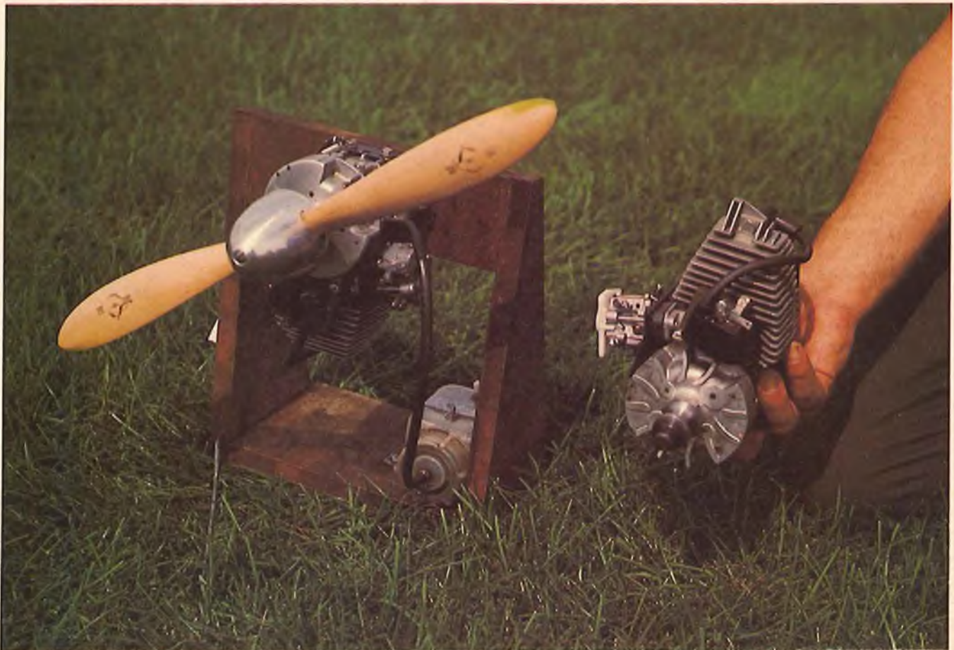
The source of all that performance, the Quadra engine. Note the fuel draw height in the mounted engine and the inverted mounting. It runs best this way and is easier to start.
