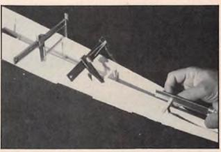
Installing upper 1/4"sq. cross braces in aft fuselage.
