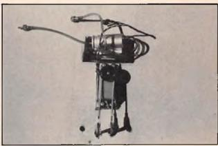
Alleron servo and pneumatic gear actuator installation. Note differential ailerons and Hydralock installation.
