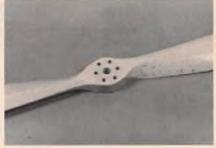
Drilled prop to accept the six No. 8 socket head cap screws. Front washer is used as a drill template as accurate drilling is a must. E.W.H. will furnish pre-drilled props upon request.
