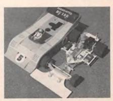
A different point of view is shown on Earl Campbell's car. Large 31/4" rear tires are used to give maximum rear traction. The rubber compound is light so turning weight is no problem.
