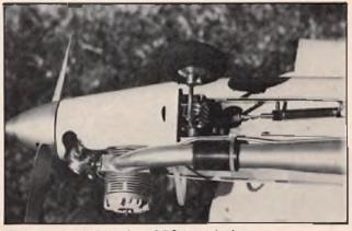
Webra speed .61 using OPS tuned pipe.
