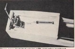
Nose gear installed along with actuator pushrod.
