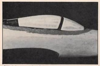
Fillet lay-up with Sears filled epoxy cement and micro-balloons.
