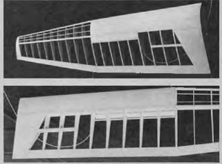
TOP: Completed MK.II wing panel. Note the D-Tube sheeting as compared to the MK.I. ABOVE: Bottom view of MK.II wing panel. Note spoiler cable.
