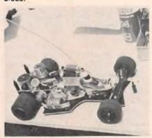
Phil Greeno had the fastest Foreign entry on the straightaway, with his K&B powered P.B. car. You'll notice his rear tires are as small as his front tires, which gives a very low final drive ratio for quick acceleration. Most of the Foreign entries ran very small rear tires.
