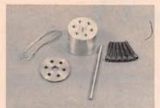
The E.W.H. prop adapter. Special screws allow lock wiring for extra safety. Lock wire is included with adapter kit.
