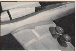
Wing fillets made from Stg Epoxolite.
