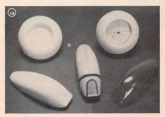
The molds and finished vacuum formed parts.
