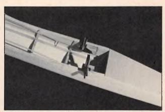
Installing hardwood wing hold-down blocks.
