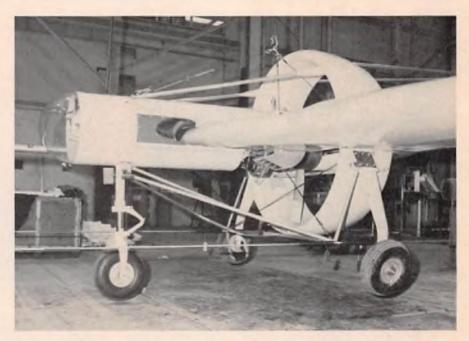
This photo shows the Lucite bubble covering the TV camera in the nose. The pilot flew the craft using this camera.
