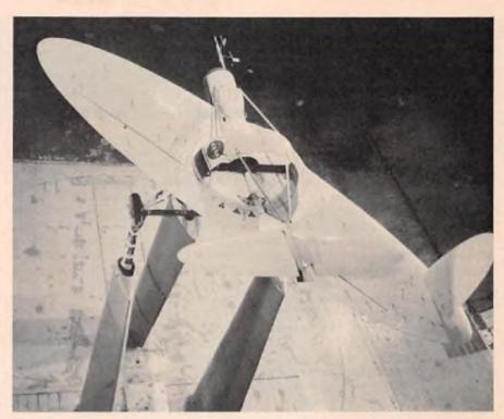
Here the Oblique Wing RPRV is undergoing tests in a NASA wind tunnel. Note the ducted engine in the center of the craft.
