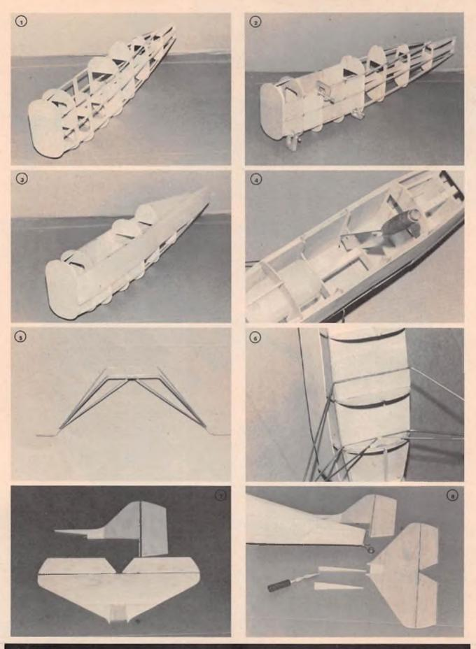
(1) Basic fuselage structure built on 1/2" sq. balsa crutch. (2) C-clamps used to glue 1/16" ply doublers inside fuselage. (3) Start of the outside sheeting. (4) Crutch is cut out at servo location. (5) Landing gear bent & soldered ready for installation. (6) Landing gear installed. (7) Tail feathers ready to attach. (8) Filler blocks trimmed to shape prior to assembly.
