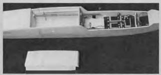
Ballast hatch cover ready for sanding. Servos shown for location only: fuse needs final carving & sanding.
