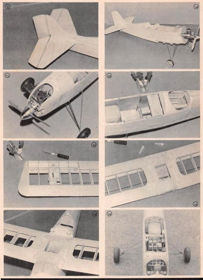
(9) Tail glued in place. (10) Engine mounted and ready for cowi blocks. (11) Cowi shaped and sanded. (12) Wing hold-down block epoxied in place. (13) View of alteron belicrank and linkage. (14) Alteron servo compartment showing wing dowels and nylon hold-down screws. (15) Wing in place. Hatch cover not shown. (16) Wing removed showing very neat radio installation. Pliot has a full instrument panel.
