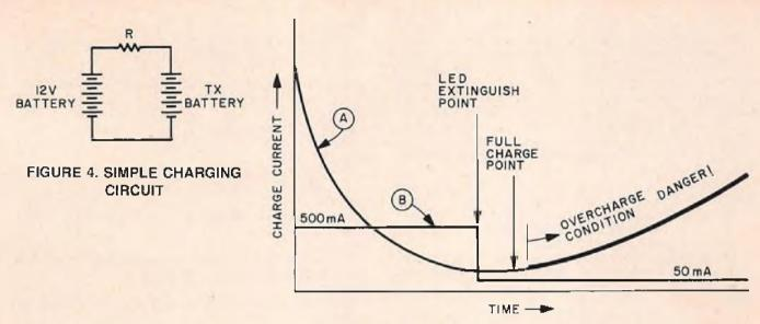
FIGURE 5. COMPARISON OF CHARGE CURRENT CURVES
