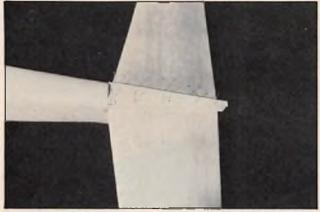
Build up of tail for fin installation.
