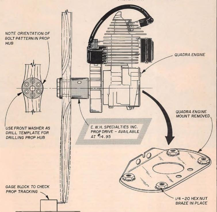
TO ALIGN PPOP FOR PERFECT TRACKING, SIMPLY TIGHTEN THE SIX NO.8-32 SCREWS, AROUND THE PROPHUB, EVENLY. THIS IS HOW IT'S DONE ON FULL SIZE AIRCRAFT. BY ALL MEANS — BALANCE THE PROP CAREFULLY.
