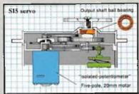
Within each sturdy nylon case lurks a custom monolithic, singleinline IC and a separate output Stage 9 pin IC for the optimum in selectivity and accuracy.
