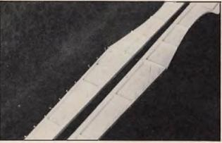
Fuselage sides built up showing vertical stiffeners and doublers.
