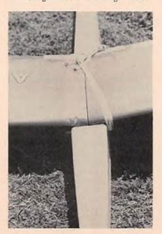
Results of snagging a winch line on launch. Photo shows untouched Oly II at completion of flight.
