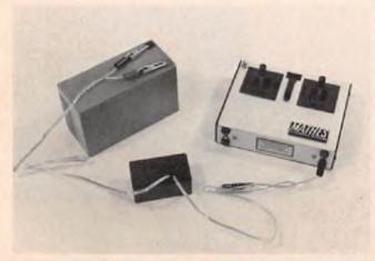
Transmitter being charged from 12V battery with MK TX.
