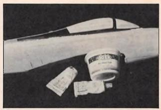
Canopy secured in place with cyanoacrylate adhesive and micro-ballons prior to making fillet.
