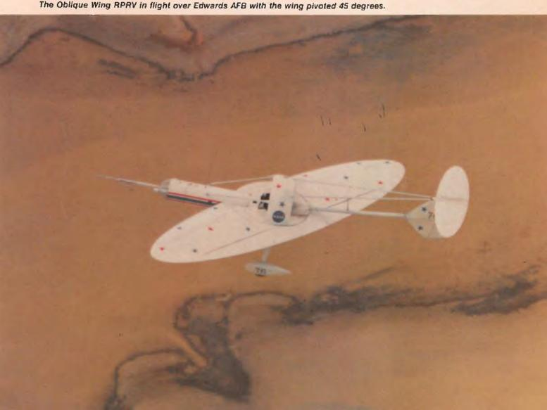
technology without subjecting human pilots to these risks. The concept calls for large scale models of the test aircraft to be flown by a test pilot located on the ground. The pilot radio controls the model in its test maneuvers using television and telemetry.
