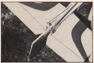
Bottom view of stab showing dual elevator pushrods. Ball link used on rudder horn.
