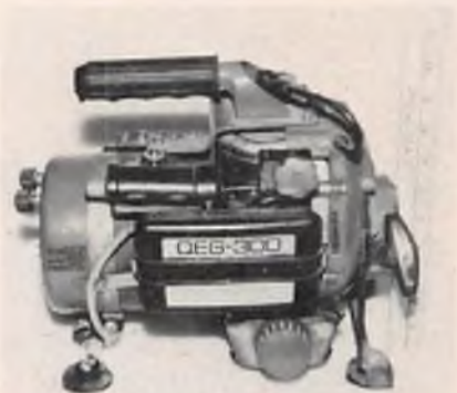
Japanese 250 watt power plant. Engine will be modified for model use by author. Cylinder head is immediately under handle base, everything to the left of the "3" in "300" will be discarded.
