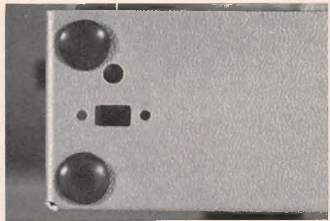
The completed holes are easy to make in the aluminum case material and are few in number.
