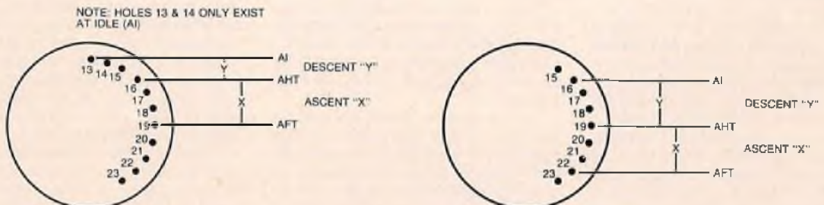
FIGURE 5 "X" ASCENT VALUES ARE THE SAME, WHILE SHOWING THE TWO DIFFERENT "Y" DESCENT VALUES
