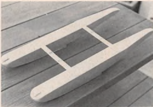
Float structure of the SSS. Note aligning blocks, and balance weights on nose.
