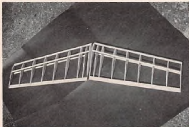
Basic wing panels completed prior to adding the leading edge sheeting.
