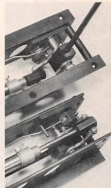
Close-up of the pivoting and locking details of the Custom Retracts. Left and right hand units are shown.
