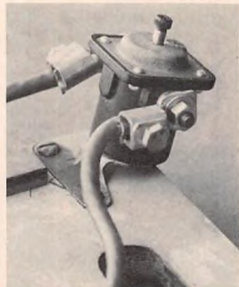
Modified solenoid. Note shoulder bolt to operate switch with foot. Screws and nuts replace rivets that retain cover after modification.
