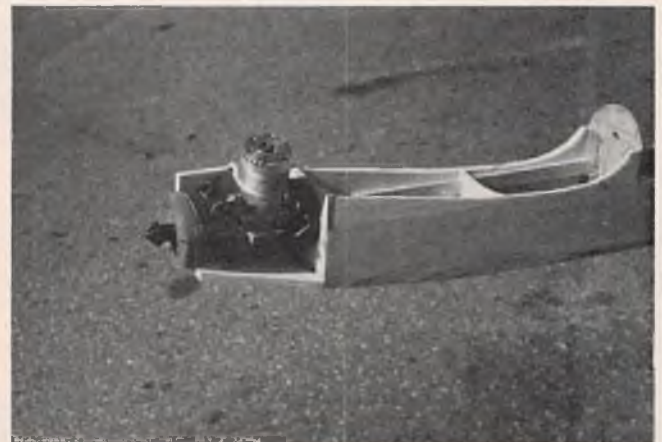
K & B .40 installed in tail of fuselage. Cowl blocks are being installed. Note rear portion of Goldberg spinner used for guide.
