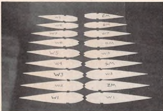
Complete set of wing ribs for both wing panels.
