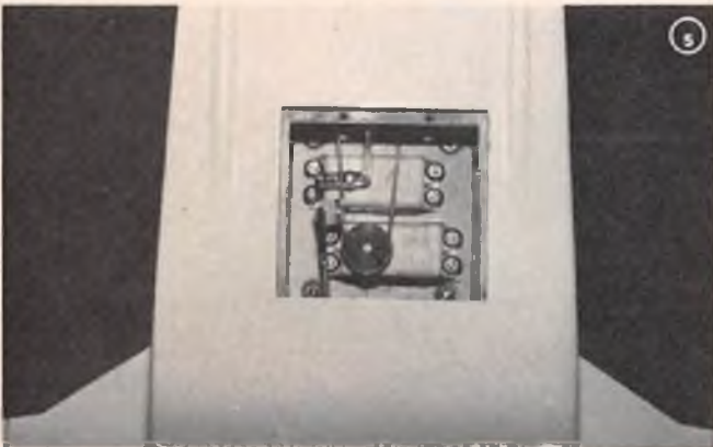
(1) Bottom view of elevator and dual rudder pushrods. Note wire skids on sub flins. (2) The main gear retracts outward to maintain good gear-down geometry. (3) Ample room inside for dual fuel tanks and radio equipment. Dual tanks help to localize the fuel mass at the C.G. (4) Inside of fuselage looking aft. Everything strapped in place. (5) Hatch removed on bottom of fuselage to show rudder and elevator servos.
