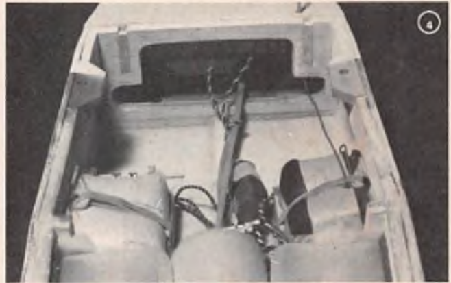
(1) Bottom view of elevator and dual rudder pushrods. Note wire skids on sub flins. (2) The main gear retracts outward to maintain good gear-down geometry. (3) Ample room inside for dual fuel tanks and radio equipment. Dual tanks help to localize the fuel mass at the C.G. (4) Inside of fuselage looking aft. Everything strapped in place. (5) Hatch removed on bottom of fuselage to show rudder and elevator servos.
