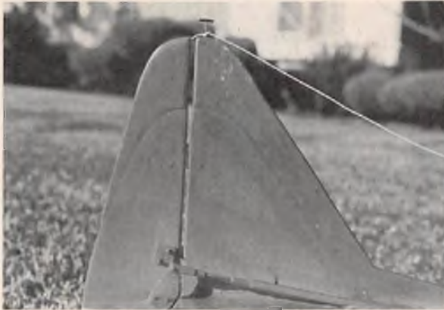
View of vertical tail surface after additional area added. Indentation line shows original size which caused snaprolls.
