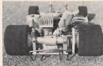
Gene Husting's car with the AMPS differential installed. This differential was 4 ounces heavier than the stock axle, but without the wing, only added 2½ ounces to the car.
