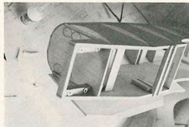
Side sheeting ready for gluing. Note bevel on bottom of side sheeting.
