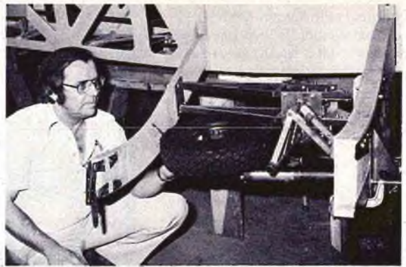
Cliff cut and welded all of the steel struts and fittings himself.
