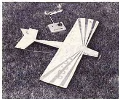
Jackrabbit uses 7% thick flat bottom airfoil.
