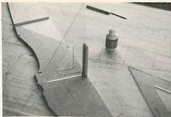
Use right angles to get cabane mount blocks square.
