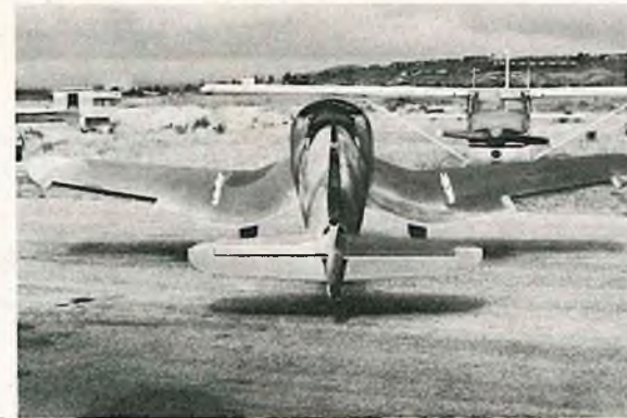
The polyurethane blocks have the glass cloth/epoxy covering and has final sanding. White streaks were replaced with sheet aluminum for wing attach access.
