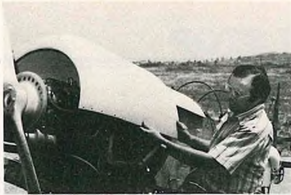
Fitting the fiberglass engine cowling was the same as with an R/C scale model except it was a bit larger.
