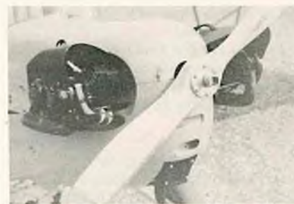
Note Sensenich trademark on prop, safety wired hub bolts and even scale clamps on hoses and scale spark plug.
