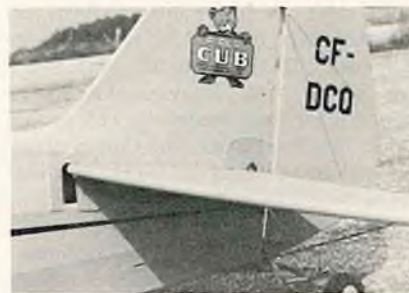
Cub trademark, access panel for elevator horn and adjustable stab, along with scale tail wheel all contribute to the realism of this project, which flies as well as it looks.
