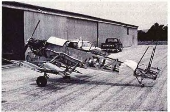
Sandbags were used to counter-balance engine weight at this point.
