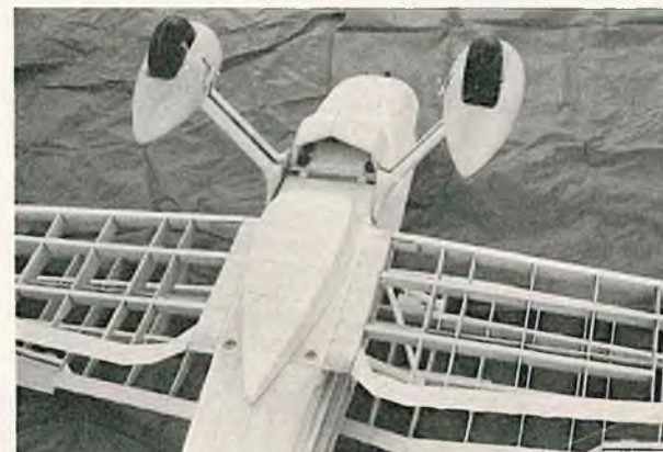
Framed aircraft viewed from bottom showing L.G. detail and aux. fuel tank.
