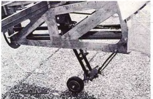
Tail wheel has leaf spring and is retractable.
