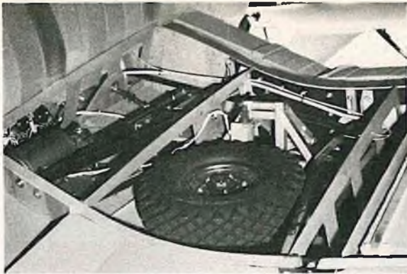
Landing gear nestles snugly into the wing when retracted.
