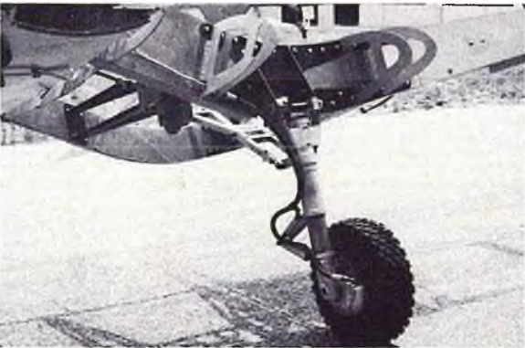
Landing gear details are visible in this photo. Note gears to rotate strut as gear retracts.
