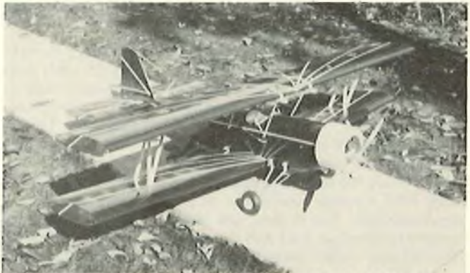
Dan Yarchin's Lazy Ace, aluminum cowl and .90 four stroke engine.
