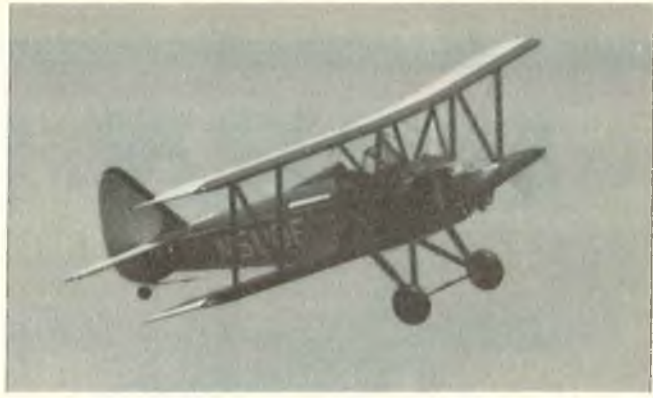
Moucha Sr.'s Fly Baby on maiden flight. Great kit and excellent flying machine. Model's test flight was made without cowling on Quadra engine, later flights included cowling with no difficulty.
