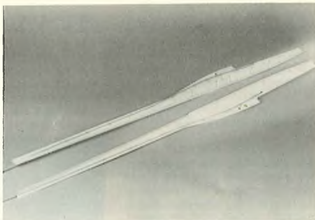
Fuselage sides with pushrods and longerons installed.
