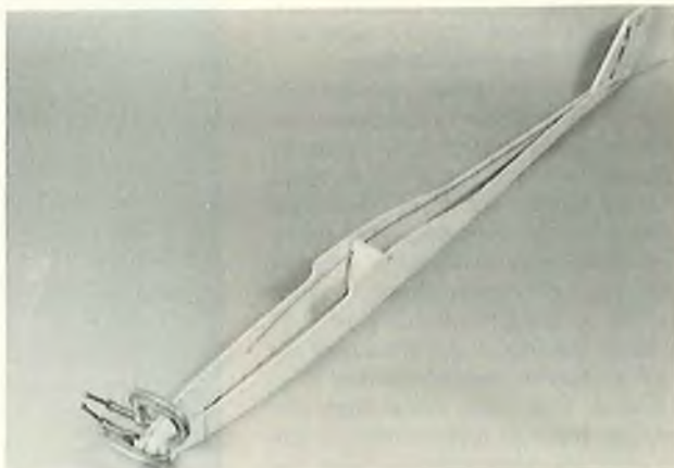
With F4 installed, glue nose block in place.
