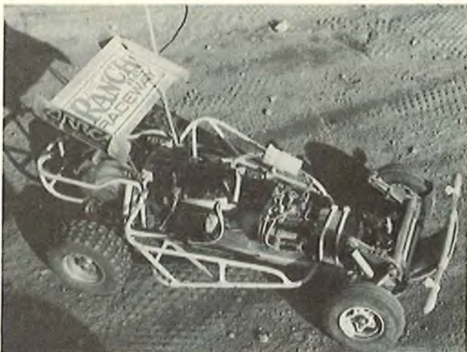
Gil's Tamiya car has been considerably lightened, ball bearings added throughout, special shock hangers in rear, special speed control, custom nerf bars added, special wing all add up to a winning combination.
