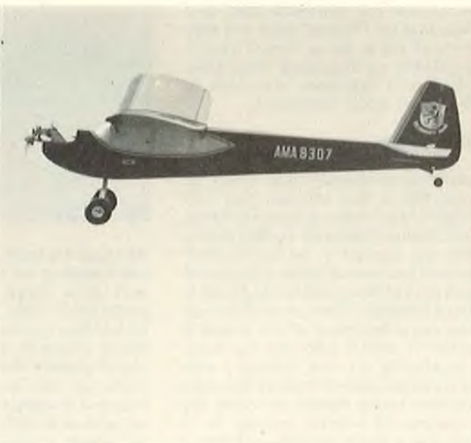
These are in-flight photos, however, the engine/drive combination was at an unfair disadvantage as the aircraft was just too much for the available thrust to sustain flight. When mounted in a proper aircraft, the Prop Drive unit can be a viable item.
