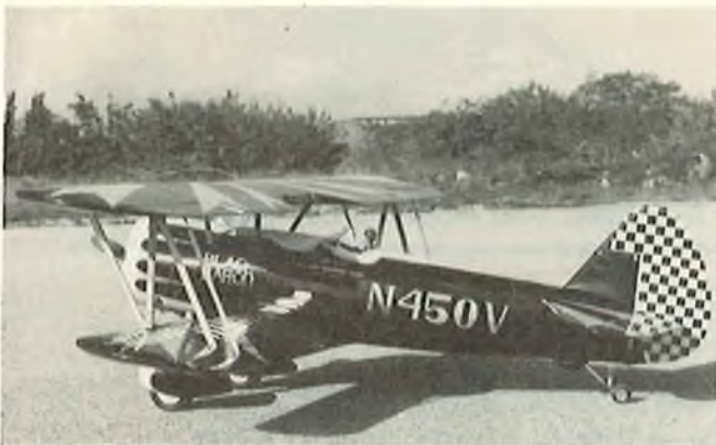
Beautiful scratch-built Stearman from Godfrey's plans. Patterned after Bill Barber's Black Baron. Kawasaki TA51 powered with 22/8 Zinger prop. Dry weight is 30 lbs.
