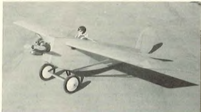
Dan Yarchin's Lazy Ace, aluminum cowl and .90 four stroke engine.
