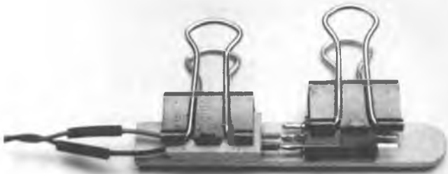
One of the best connector soldering jigs available. A popsicle stick and two paper clips. It works simply great! See RCM April 1981 Here's How. Don't forget the shrink tubing before soldering.
