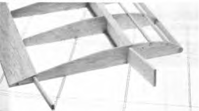
Notch center and tip dihedral break ribs. Zap braces in center section.
