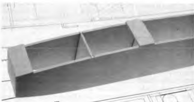
Zap in hatch hold-down plates.
