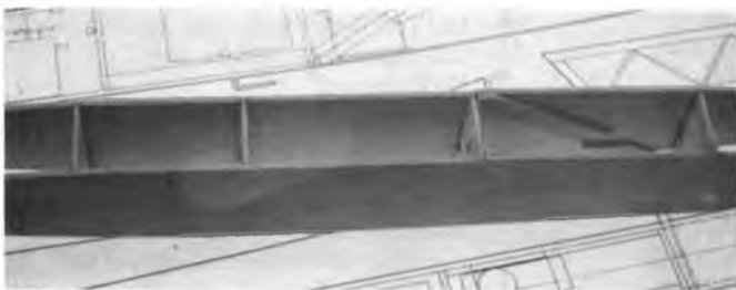
Join right hand side to formers.
