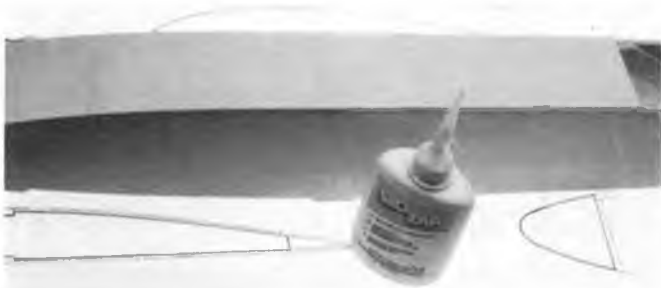
Zap in forward bottom (cross grain).
