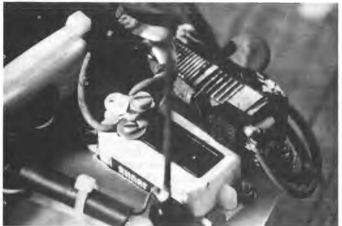
Shows microswitch mounted on servo with servo tape.
