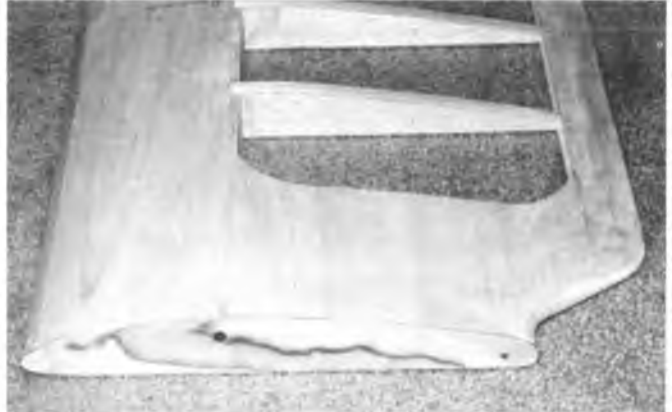
Top view of inboard end of finished wing panel. Retaining screw not shown.
