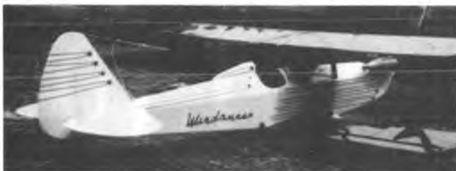
Jimmy Sikes of Dalton, Georgia, rewarded us with a photo of his first scratch-built model. It is the Wayfarer (RCM plan No. 482, $6.95) powered by an HB .40 PDP engine. Jimmy used a split linkage on the elevators. He states it is a real smooth flier.
