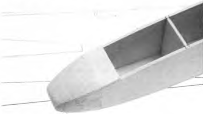
Zap on nose and shape.
