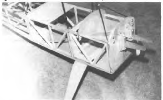
Details of engine mounts and landing gear supports.
