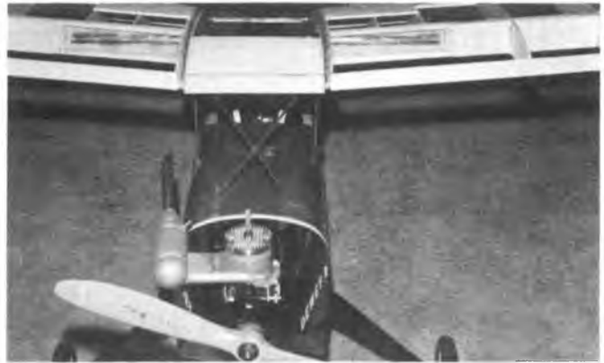
View showing wing panels mounted and carry-over tubes tack cemented to spar web. Dihedral and alignment is established here. That's a K & B .61 up front.
