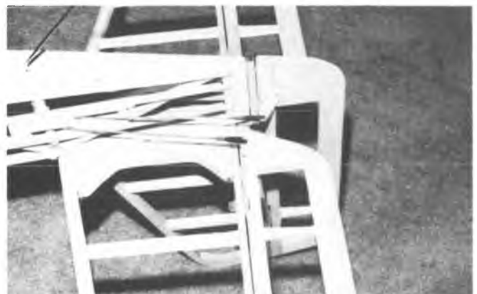
Plates with slots for pushrods to facilitate covering and support rod eyelets.
