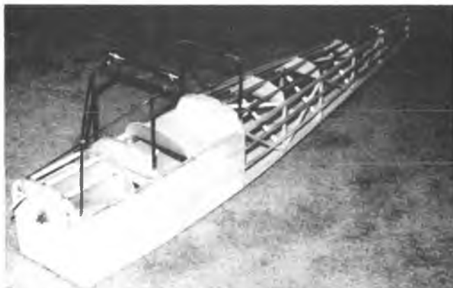
Fuselage with side 1/16" ply planking and stringers. Sand everything smooth and flush where stringers meet side planking.
