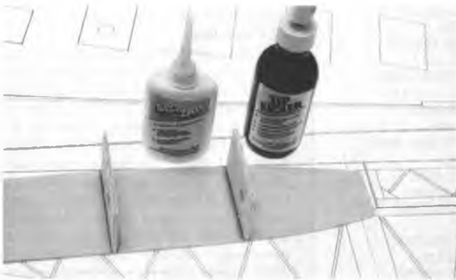
Zap and Kick formers and joiner to left side.
