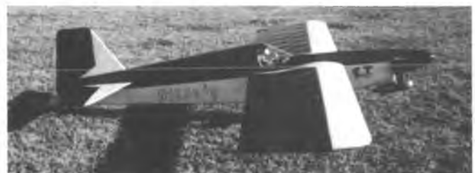
Bob Williamson, Inola, Oklahoma, increased the plans 50% and powered his 84" wingspan Magnum with an O.S. Max .90. He says it is the best flying model he has ever flown. Magnum plan #745, $6.50.
