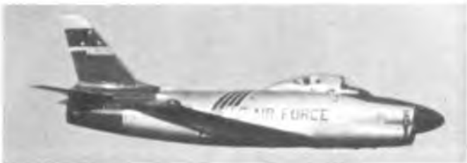
F-86D from the Byron kit on its first flight, 5 p.m. Christmas Eve, 1982. It sure would have spoiled builder, Bob Temple's Christmas if it had not flown right. OPS 65, Spring Air retracts and that is a radome on the front, not a prop spinner.
