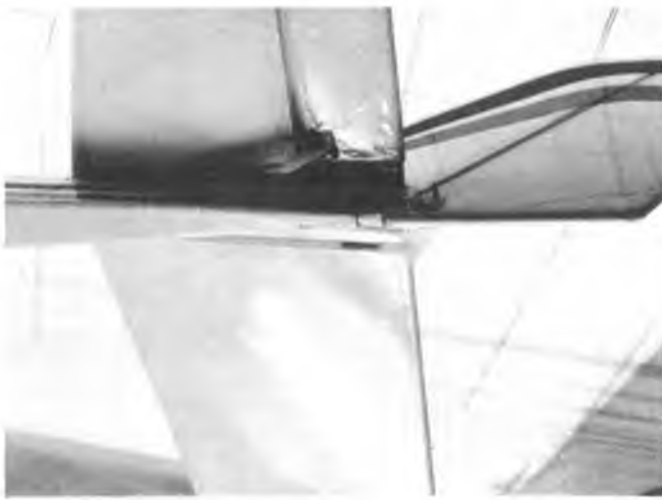
Pushrod hook-up. Clean and simple.
