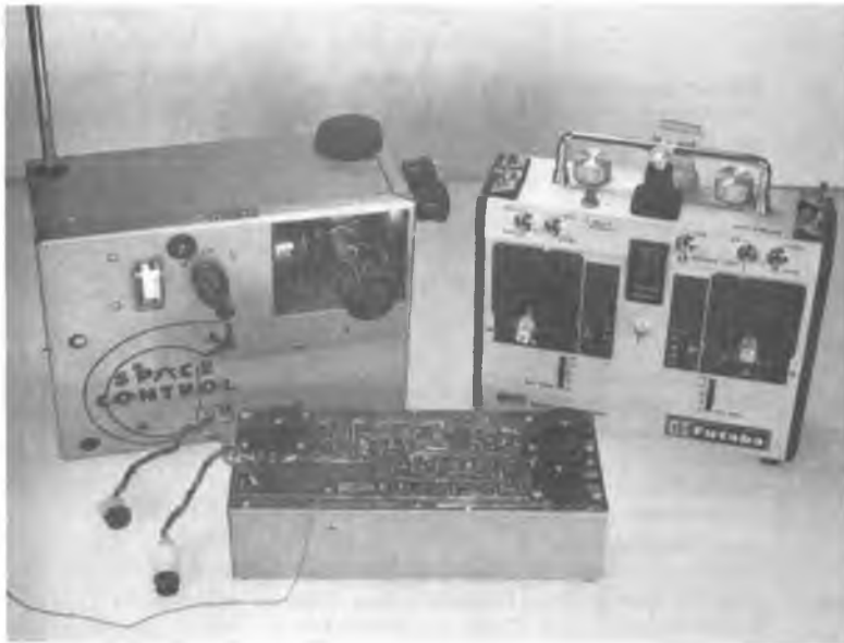
Space control, an analog system, was the first commercially available proportional radio for model usage. The famous brick contained receiver and three servos. Futaba's multi-function programmable transmitter is shown for contrast.
