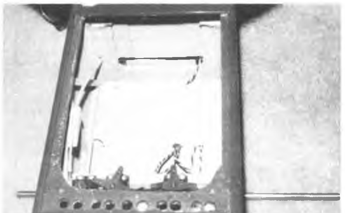
Simple snap in hatches to keep things in place can provide substantial clear cargo space. Room for two more servos to drop cargo or perform other tasks is provided.
