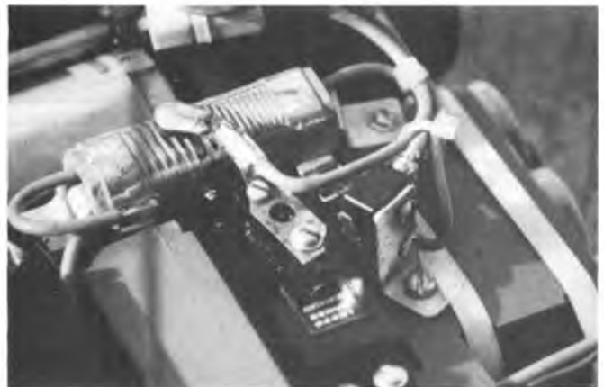
Shows microswitch mounted on "L" bracket as indicated in drawing as #2.
