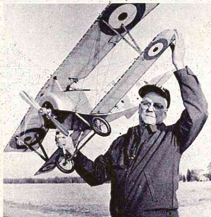
Roscoe Hibbard and his Proctor Nieuport II. Enya 60 swings 20" laminated prop, easily hauls 7½ lb. beauty. Wheels by E.B. no longer available. Kraft radio.
