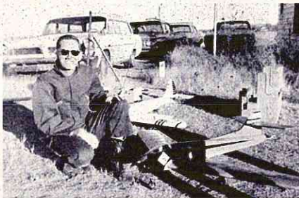
Jim Mowrey and orig. Jayhawker. Mercó 61, 25° sweep wing & stab, 60" span, split rudder. EK radio, ship took 2nd in Oklahoma City Hobby Fair.
