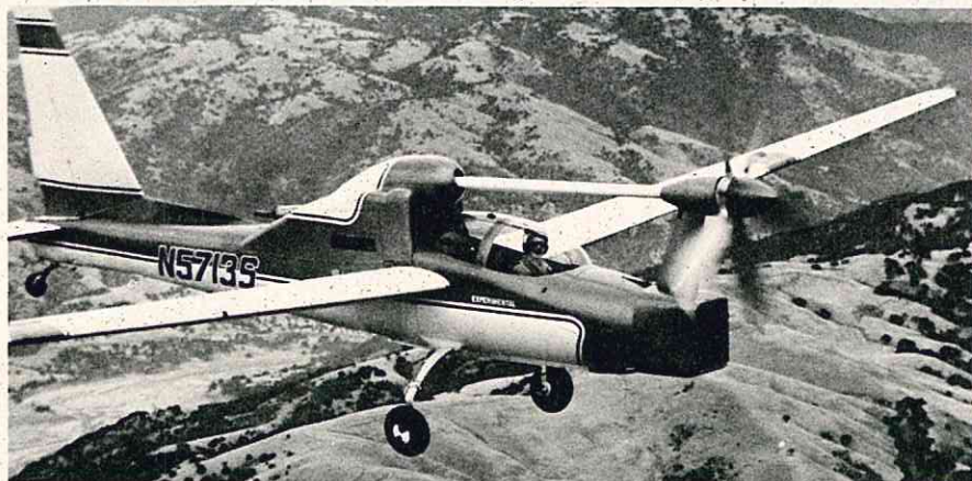
A quiet flying acoustic research aircraft developed by Lockheed Missiles & Space Co., Sunnyvale, Calif., wings silently over the California's central valley. Called Q-Star, aircraft has been developed from unpowered Schweizer SGS 2-32 sailplane. Lockheed is using Q-Star in tests of aircraft acoustics and airborne equipment.
