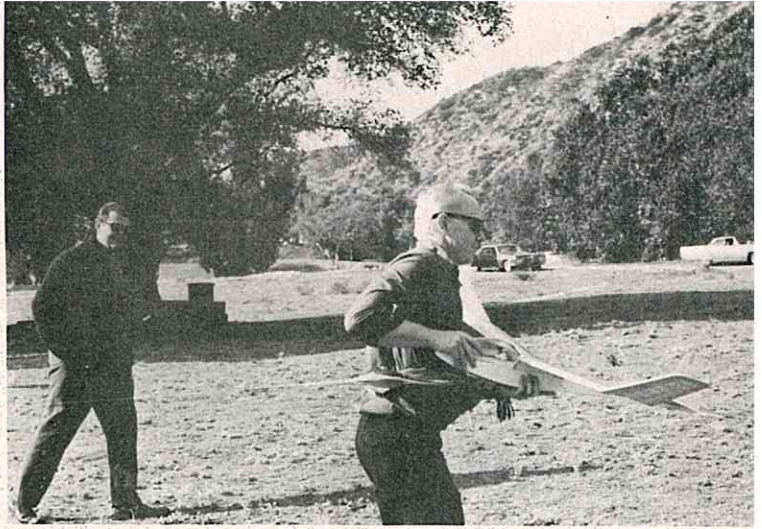
As Ron Neal watches, Don walks back with glider to obtain maximum stretch. Note chute attached to tow hook.
