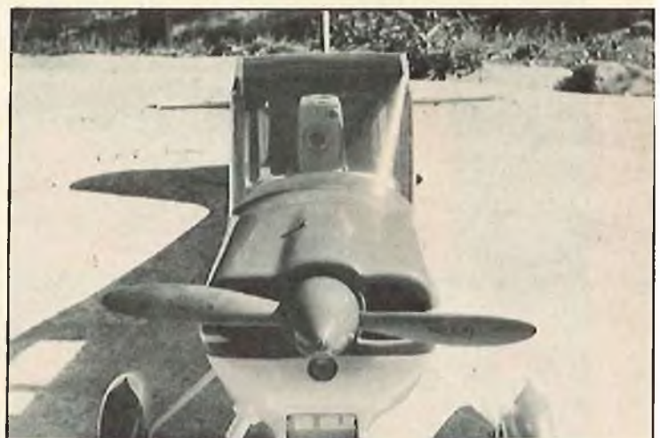
This front view shows everything mounted in place. The camera is angled two degrees from level. The top of the needle valve can be seen in the movies. The 14/6 prop is literally dwarfed by the width of the Citabria cowl.
