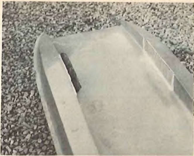
The turn fins on the catamaran. They are 1/3 of total length back from bows and bent inwards 35°.
