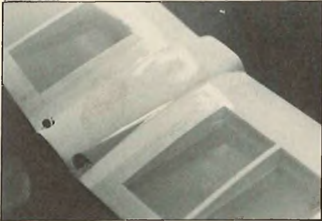
Center section of wing showing nylon hold-down bolts.
