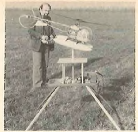
The Helpe Heli Trainer, developed in West Germany by Helmut Fett, is one of the finest reflex trainers produced to date.
