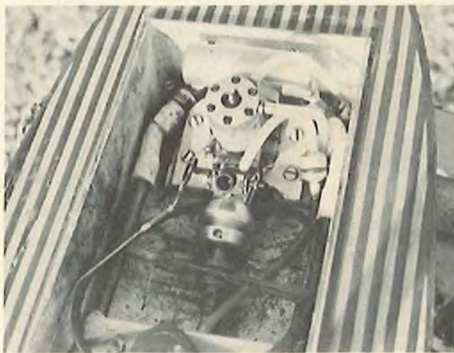
Compare the throat bore to the Perry carb on this K & B 21 inboard.
