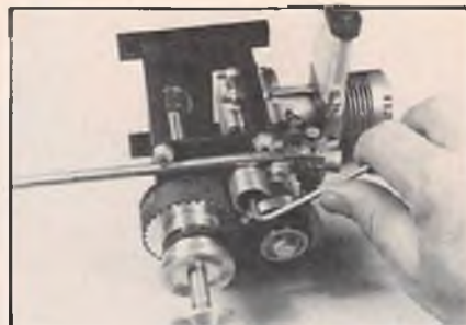
I used a screwdriver to put pressure against the idler to get the right tension on the belt. Use just enough but not enough to have a lumpy feel when you turn the prop over.
