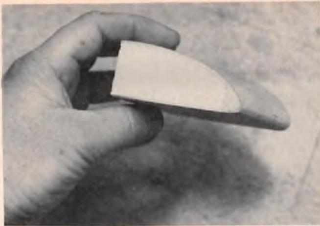
Test wing panel section sheathed and leading edge applied with Supertape.
