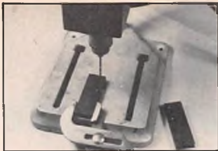
Remove plates from unit and drill holes for threading or for using bolts and nuts. Hold plates firmly so they will not grab on bit and cause injury.
