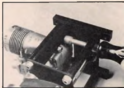
As a safety, I install aircraft lock nuts to bottom of bolts.
