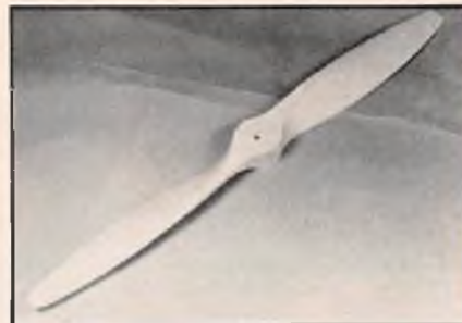
Grish prop as it comes from the box. Sanding and rounding of edges is necessary.
