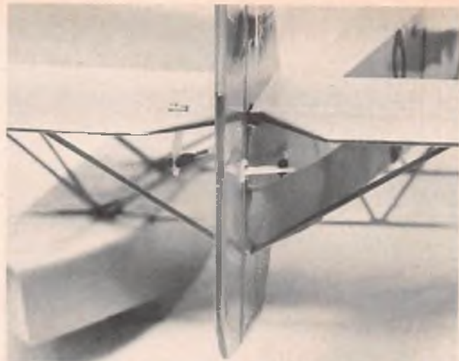
ABOVE LEFT: This frontal view clearly details the intricate array of struts used on the HM-II. ABOVE RIGHT: Scale placement of the pushrod exits and control horns is evident here.
