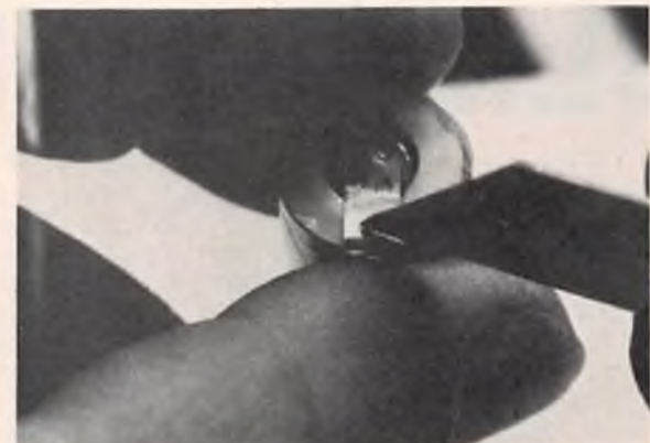
A bright surface ensures proper tinning.
