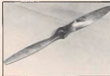
Finished prop was stained with walnut and rubbed for an antique look. Clear R & S Perfect Paint was used to fuel proof.
