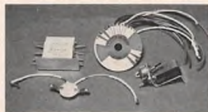
Workrite electric controller, designed for 1/12 scale cars, but excellent for boats. Photo shows printed circuit board, wiper fixed to Futaba servo disc, on/off switch and charge jack, and resistor bank.
