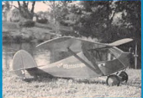
Wing span 49 inches, weight area 338 sq. inches, 2 or 3 channel radio, 049 glow or 05 electric.
