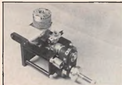
Motor and muffler installed and ready for tightening the idler pulley against the belt.
