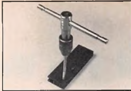
Here, tapping for 6/32 bolts is made easier by using bacon grease as a lubricant.
