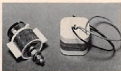
Astro-Flight Marine 05 electric motor - complete with plastic mounting - and power pack - four 1.2 ah nicad quick-charge cells.
