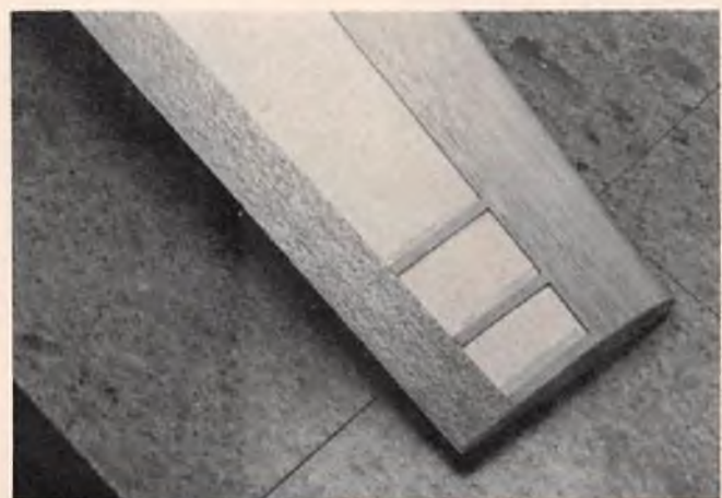
Sailplane wing panel partially sheeted, leading edge, ply wing tips, and false rib capstrips applied with Supertape.
