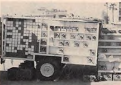
The Central Florida R/C Auto Racers Club have an efficient trailer that not only holds the track boards, but opens up into stands for placement cards and radio impound.
