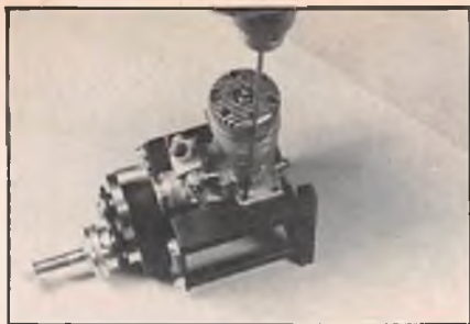
Temporarily mount the engine to the pulley and bearing plate and mark for drilling holes. Here I use 5/32 wire sharpened as a bit to mark hole locations.
