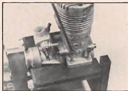
With motor re-installed into bearing plate, you can now put in the engine bolts. Ball wrench works well for installing bolts.
