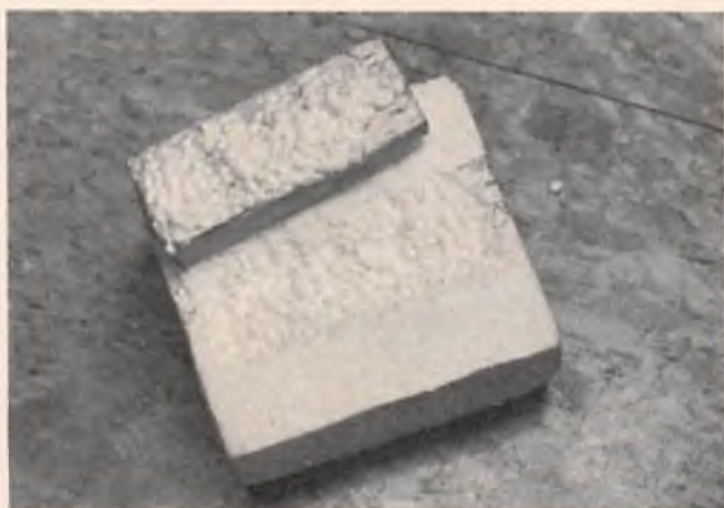
Balsa block torn loose.
