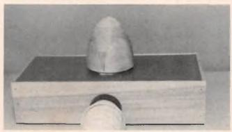
The spinner mold on the base ready to make a part.
