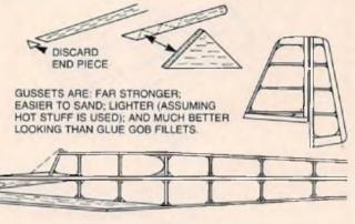
GUSSETS CAN BE FORMED EASILY AFTER HOT STUFFING IN PLACE, USE A ROUND DOWEL WITH A LIGHT GRADE SANDPAPER. (SEE CABIN AREA ON FUSELAGE IN THIS ILLUSTRATION.)
