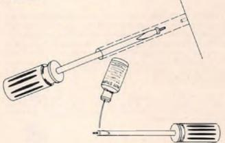
**Doubler Construction Made Easy:** Drill small holes in doublers before assembly (about every 1/2"). Fit the doubler in place and apply Hot Stuff in each hole and, finally, around the edge. If the doubler is huge and no sanding will come into it (from a fuselage curve for instance), the holes could be very large and lighten structure at the same time.
