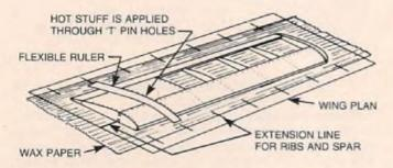
BOAT HULLS, AS WELL, A SNAP USING THIS METHOD. "HOT STUFFING" THROUGH 'T' PIN HOLE HAS BEEN DESCRIBED AS SIMILAR TO "BLIND RIVETING" AND IN MOST CASES, ELIMINATES THE NEED FOR CLAMPS AND OTHER HOLDING DEVICES. AS SOON AS IT'S HOT STUFFED, IT'S DONE.
