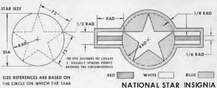
THE CIRCLE ON WHICH THE STAR IS CONSTRUCTED AND NOT TO THE OUTER EDGE OF THE SLUE OUTLINE
