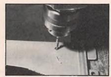
Larger hole so that nail passes freely through metal bracket.
