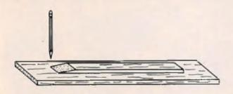
Step #2: Apply Hot Stuff over pencil line and wipe quickly with the edge of a piece of spruce to smooth before curing takes place. Note: Inside and outside of trace line should be coated as far as necessary --- usually 1/2".
