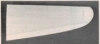
Assembled and sanded wing. Allerons and inboard sections temporarily attached, later removed for installation of hinges and torque rods.
