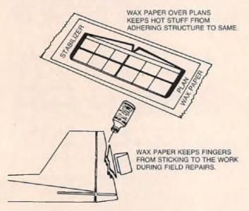
Dihedral Wing Panels: To make duplicate dihedral angles, place the root end of the wing panel at the very edge of the work surface. Block up the tip to desired height. Put a drop of Hot Stuff between the work surface (if wood) and leading and trailing edge. Sand root ends using the vertical work surface edge as a guide. Remove by sliding sharp blade between surface and structure.
