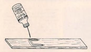
Step #3: Hot Stuff the object to be faired in position with trace lines. Now sanding can be done to fair the one into the other while Hot Stuff protects bottom piece against gouging. Caution: A heavy hand will gouge anything.
