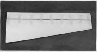
The two core pieces, and the tapered spar. Basswood was used for the latter, though plywood is acceptable.
