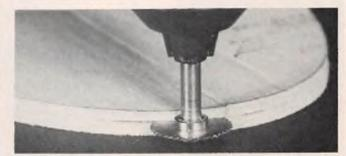
Cutting the slot around the perimeter of the tail surfaces for installation of plywood reinforcement.
