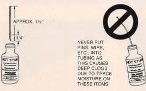
PREPARING FOR USE - UNSCREW CAP, INSERT TEFLON APPLICATOR TUBE 1/4" INTO THE CENTER OF THE FLAT SPOUT. IF HOLE SEEMS TOO TIGHT, USE A PAPER CLIP TO OPEN IT SLIGHTLY, THE FIT SHOULD BE
