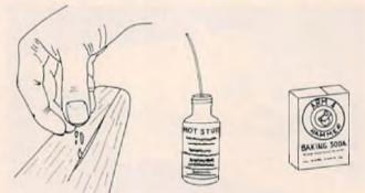
SPRINKLE BAKING SODA INTO SHALLOW GAPS, WIPE OFF EXCESS. APPLY HOT STUFF. DEEP GAPS (HOLES) SHOULD BE FILLED IN STAGES (SODA & HOT STUFF - MORE SODA & HOT STUFF), THEN SAND
