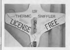
It operates on the 49 MHz band, at one tenth of a microwatt power, When it's approved, you won't have any excuse for missing that thermal and winning the contest. Unless, of course, you blow the precision landing. Wonder if anyone will ever come up with a homing device that you can stick on the spot and force the sailplane to come to rest right side up with the nose nestled up against the spot?
