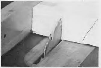
Cutting a slot for the full length full depth spar, added for extra strength.
