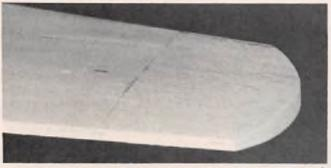
The wing tip, now shaped and sanded to the taper of wing top and bottom.
