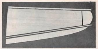
Sheeted core, shown with the rest of the pre-shaped balsa pieces required to give it the elliptical shape.
