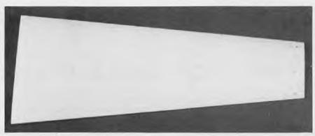
The elliptical wing core, looks like any other wing core before the addition of balsa covering, leading and trailing edges.
