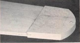
The curved wing tip, sanded to outline shape, in position prior to shaping and sanding.
