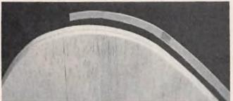
Plywood insert prior to installation in rudder. Procedure for making described in text.
