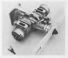
box without a prop at 2 lb., 12 oz. It is ported to run at high speed so the suggested ideal prop size is 13" diameter with 16/4 given as the largest practical prop. 11/8 as the smallest. But with 3 hp being developed at 14,000 rpm, don't worry about prop sizes. Duke says, "Leave the huge propellers for motors that are not capable of revving up."
