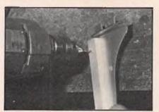
Smaller hole through both wood and metal brackets.
