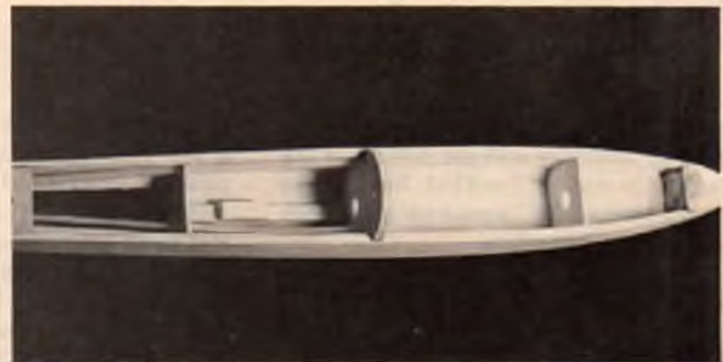
Fuselage bottom installed with towhook mount in place, note pushrods.
