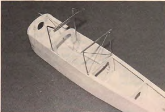
View showing forward cabane struts "glassed into" corner of F2 and side. Also see engine mount blind nuts and throttle cable installation.
