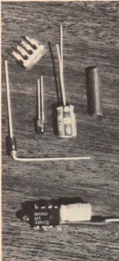
FIG. 3. Components of flashing LED indicator and top view of finished module before encapsulation in black epoxy. LED shows operation of Solar array but draws only micropower.
