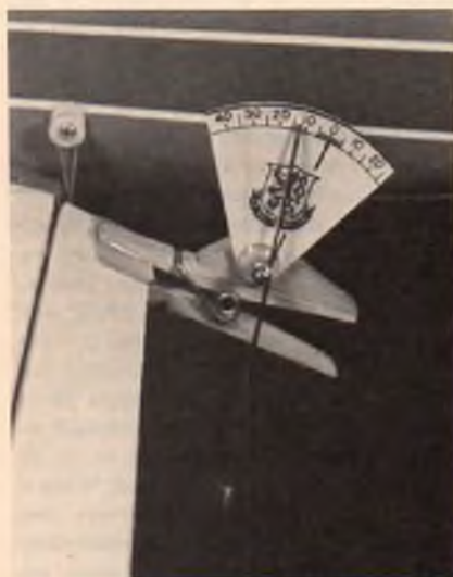
Gauge dial is calibrated in degrees.
