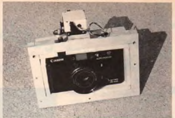
Camera mounted in module. Servo actuating mechanism sets right on top. Fundamentally simple and quite reliable when properly adjusted.
