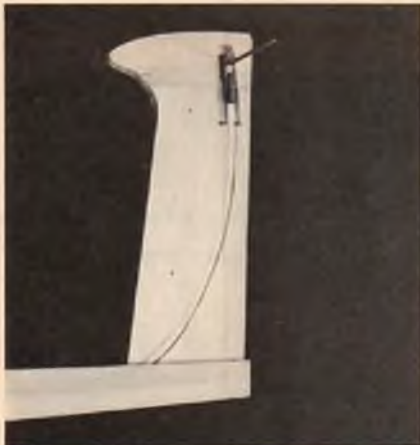
Su-Pr-Line pushrod with Rocket City ball end link. Trial fit into fuselage before covering sides.
