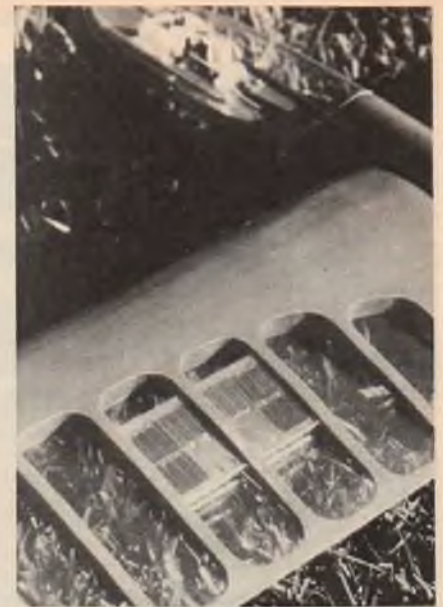
FIG. 17. Another view of airborne Solar battery mounted in plane.
