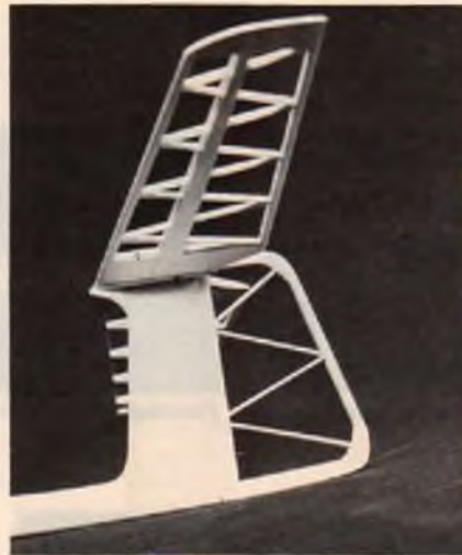
Flying stab viewed from underneath.
