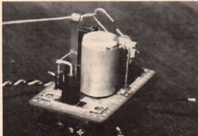
FIG. 13. Regulator-charger details: Trimming potentiometer; trigger adjustment and hardware mounted on heatsink of regulator; connections at microswitch terminals. Trigger line is stranded white Dacron.
