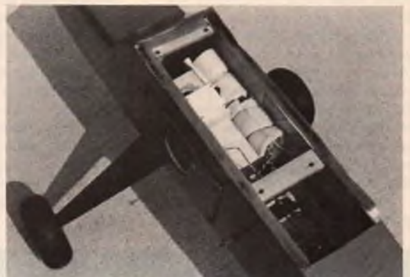
Camera installation in Telemaster. Only 1 1/2 lbs. extra with plenty of spare room.
