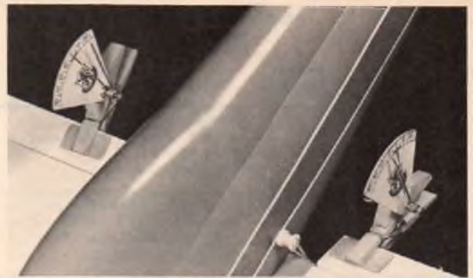
Two gauges in use showing aileron differential.
