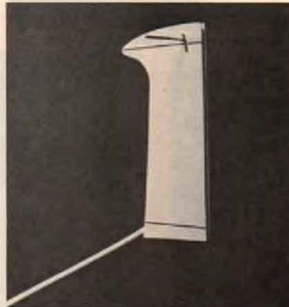
Vertical fin with pushrod installed and side sheeting attached. Notice reference lines used for alignment when gluing to fuselage.
