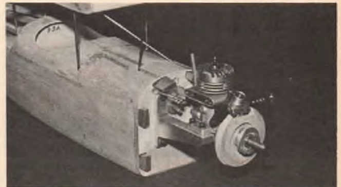
NR2 and NR3 pressed onto engine nose and cowling blocks mounted on F1. Cowling pattern can now be fitted. Note blocks are off-set thickness of cowling material for smooth joint.
