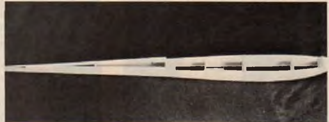
Fuselage sides with formers and noseblock in place.
