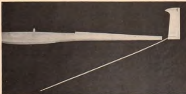
Glue vertical fin in place before sheeting top and bottom of fuselage.
