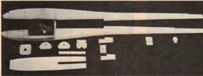
Fuselage sides showing triangle stock glued in place. Note F-2 is at a right angle to fuselage side.
