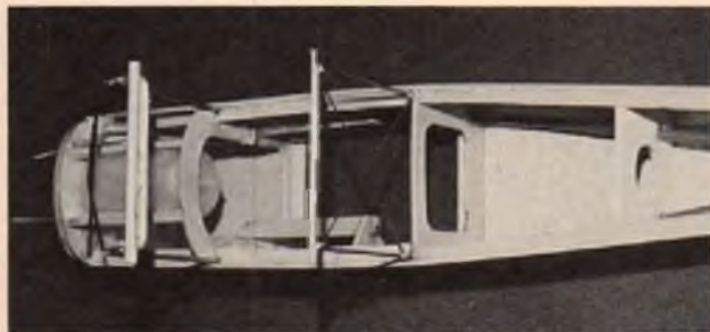
Forward cross struts "glased" to F1 and top longerons. Keep ends at F1 "in" enough to avoid interference with front cowl sheeting. Note servo rails.
