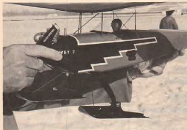
Detail of skis showing music wire spring holding nose up.
