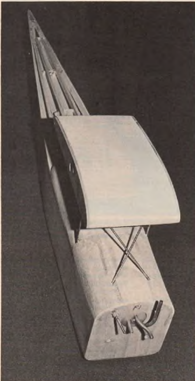
Finished and rough sanded fuselage and center section.
