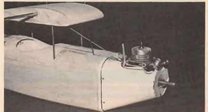
Oversize vellum pattern taped to nose ring and F1 blocks. Note pattern has been marked at F1, to clear the muffler, and that the centerline at the bottom of NR2 has been defined.
