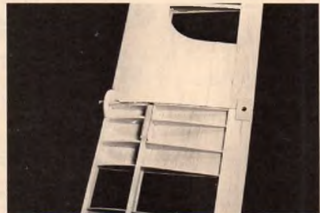
Wing center section showing wing mount brace at trailing edge.
