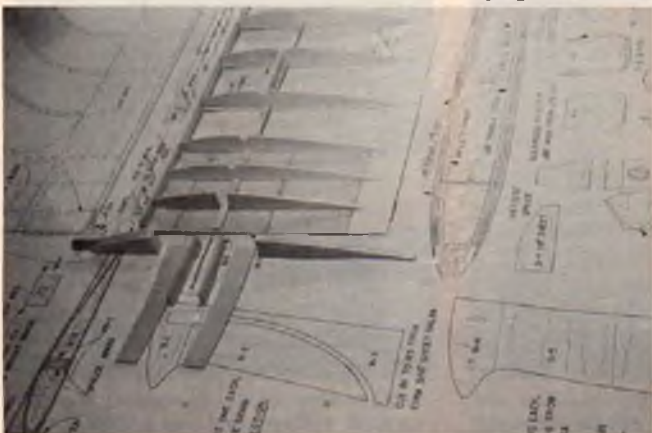
Right wing half, the first 3 ribs are cut to clear the 1/16" birch ply dihedral braces. Note the wing mount assembly with the 1/4" dowel in place.
