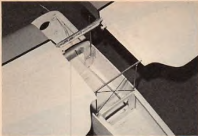
Wings are attached and wholly supported by cabane wires and are not dependent on any wood parts of center section for strength or position.
