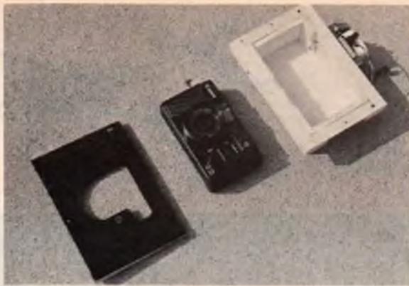
Front cover, Canon AF 35M and camera module. Rubber foam lining and shutter button can be plainly seen.
