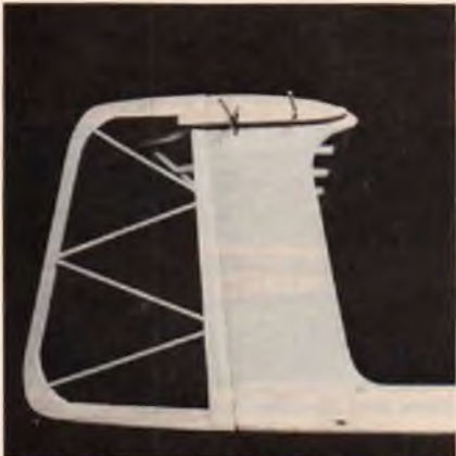
Vertical fin with flying stab mounts in place.
