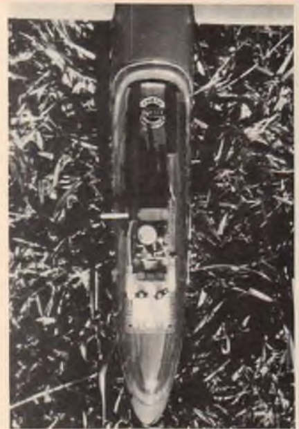
Fig. 12. Regulator-charger in nose of Hobie Hawk. LED flasher is mounted between control rods, aft of circular decal.
