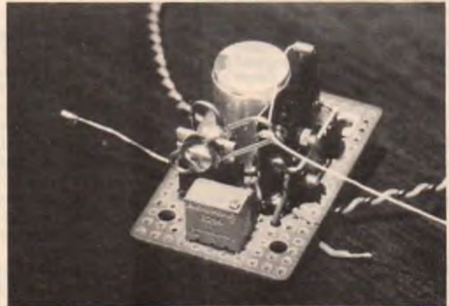
FIG. 14. Regulator-charger details: Slide switch; diodes forward of microswitch; microswitch-capacitor bracket. Outboard lead of resistor R-2 shows behind bracket.
