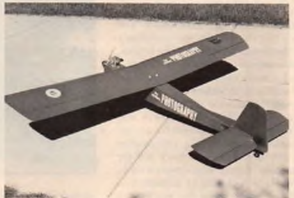
1973 Telemaster that has hauled a number of projects aloft. Webra .91 on front is good for short fields and gets up there quick.
