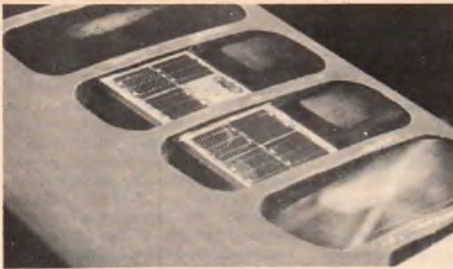
FIG. 1. Pair of Solar arrays mounted in wing of Midwest Hobbie Hawk. Covering is clear Super MonoKote.
