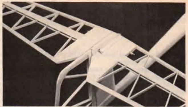
Flying stab and rudder are trial fitted.
