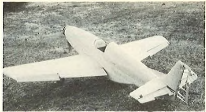
Big P-51 is the work of Michael De Muth of Ellicott City, Maryland. Mustang was begun in 1980, and the builder says he got carried away and has been adding features almost ever since. Mustang has functionally sprung gear, working trim tabs, 28/15 flying prop and all gear doors are operated from separate system to retract gear. Hopes to fly this year. Some task for a beginner!
