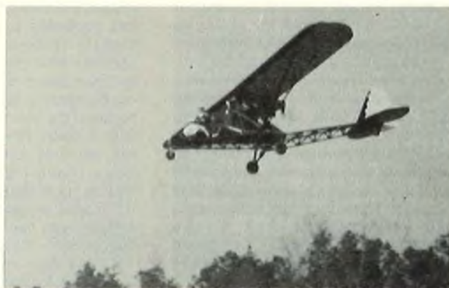
Breezy airborne. Power is 1.6 Homelite engine, construction is spruce, bass and plywood with some sheet aluminum as well. Weight is 27.2 pounds. Pilot and passenger are hand carved Popeye and Olive Oyl.
