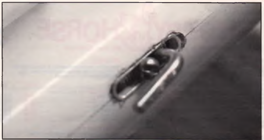
Adjustable towhook installed in the fuselage.
