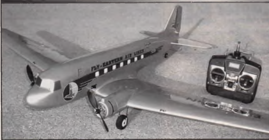
Photo #1: Great Planes DC-3 Electric ARF. 60" built-up wing with fiberglass fuselage, the model also includes two Speed 400 electric motors with a speed control, powered by a single 9.6v 1800 mAh NiMH battery pack.
