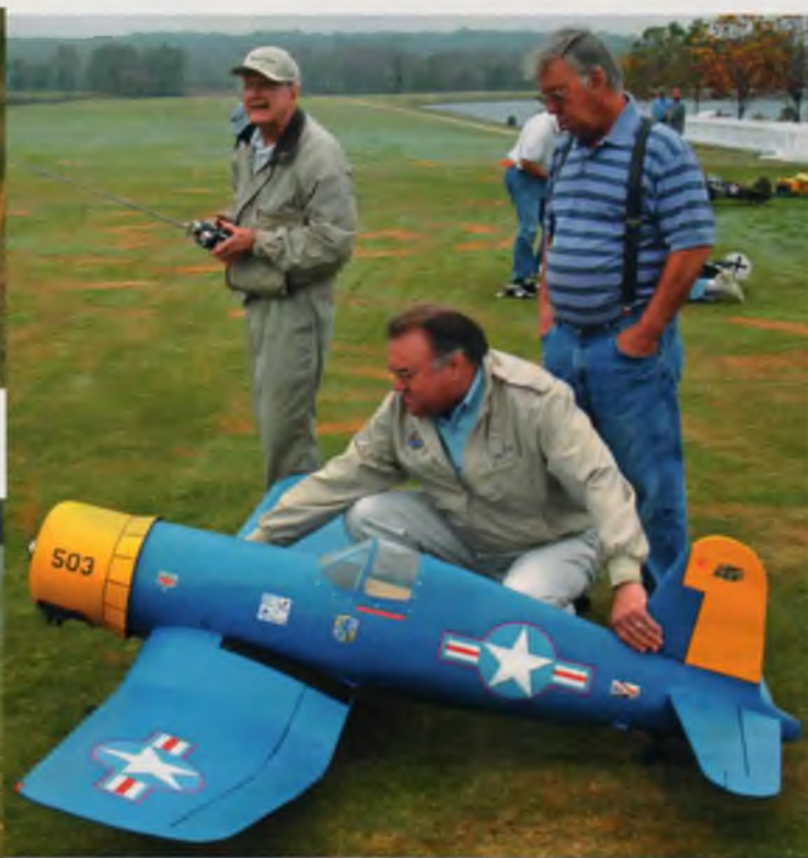
ABOVE: 87-year old Slick Larsen scans the skies before taking off. Good friend Gene holds while Bob Johnson looks on. Slick's airplane of the day (he has over 50 in the hangar) is a Zirol Corsair F4U powered by a G-62 with Robart retracts.
