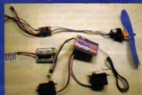
FMA M5LV low voltage system shown with a low voltage M20 gear motor. The motor is available from Bob Selman Designs.
