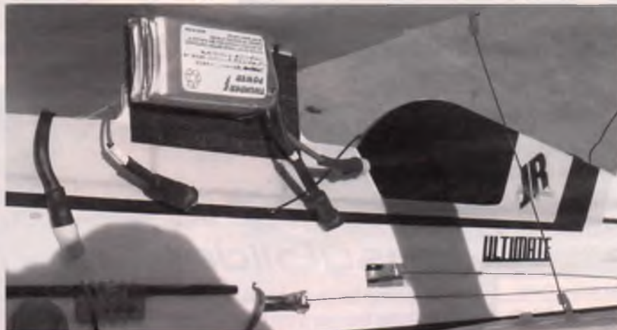
Ultimate; proper battery location.
