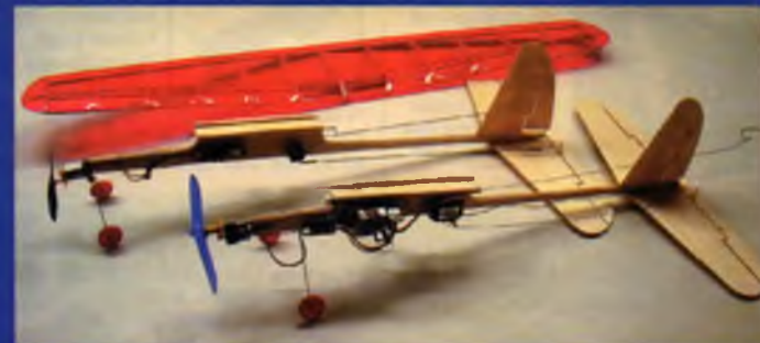
The Micro Flash in the foreground has the FMA M5 with 2 PS20 servos and an M20 low voltage motor. The model in the rear uses an RFFS 1000 receiver and two Selman magnetic actuators and a KP 00 gear motor. Both models fly with a single Kokam 145 mAh LiPo cell.
