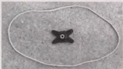
Prop saver: Futaba (6 arm) servo arm with 2 arms removed and a 3mm nut pressed into the center.
