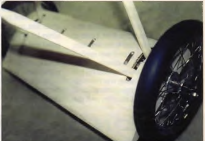
The landing gear wing has front and rear halves and they are attached over the spreader bars with metal straps. These removable straps allow for easy disassembly if needed to replace the rubber band shock absorbers.
