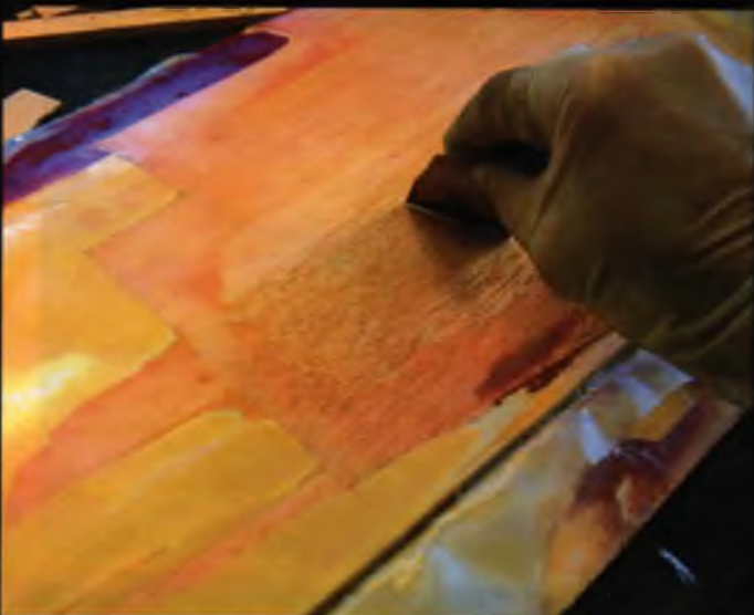
Photo #7: Applying 3/4 oz. glass with card.
