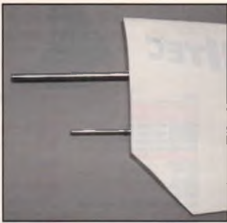
The Nova uses a full flying stabilizer, joined with steel rods.
