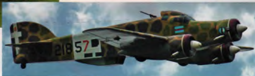
ABOVE RIGHT: Ty Brown, Kannapolis, NC, does a fly-by with his Italian Savoia-Marchetti SM-79 three-engine bomber. Ty scratch-built this 110" almost 1/7 scale beauty with two Magnum .52 4-strokes in the outer nacelles and an O.S. .91 4-stroke in the nose. The ever-popular Latex paint was used to produce this colorful scheme, which can be easily lost in the grass. 22 lbs. ready to fly. Bad weather, yep, but PhotoShop came to the rescue with the blue sky and clouds!
