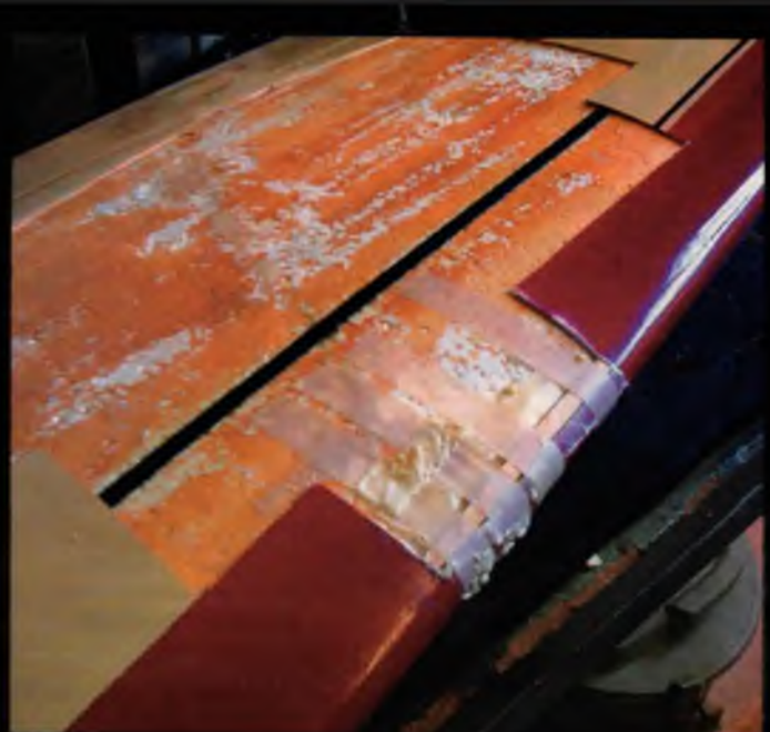
Photo #4: A doubler added to the back of the leading edge.
