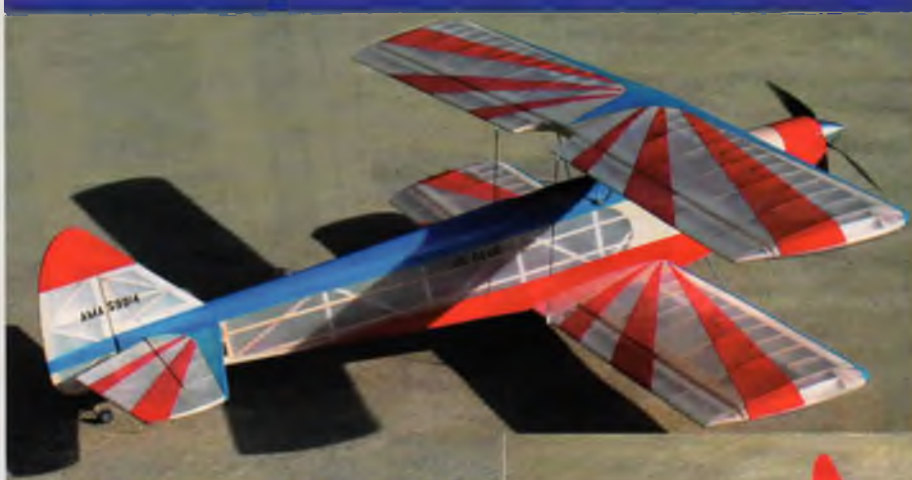
ABOVE: E Bipe built and flown by Joe David of Columbus, Ohio. The E Bipe is a conventional balsa and plywood model exquisitely covered with silk and dope.
