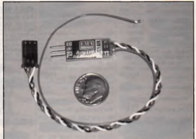
LEFT, Photo #3: Close-up of FMA Super 20 speed control, size only 1.15" x .75" x .40". Features include proportional throttle, throttle end point adjustment (EPA), motor brake (on/off), battery eliminator circuit (BEC), low voltage cutoff appropriate for NiCd, NiMH and LiPo battery packs, and motor restart. Note: the Super 30 speed control is slightly larger with the same features except for a higher 30 amp output. RIGHT, Photo #4: "Auto Cell Detect Low Voltage Cutoff," this handy device plugs in-between your receiver and speed control to give you auto low voltage cutoff when used with speed controllers that don't provide a low voltage cutoff or the low voltage cutoff is not appropriate for LiPo battery packs.
