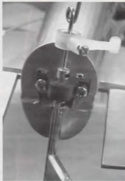
The author chose to use the top part of the tail wheel strut to drive the rudder. This allowed him to eliminate the complexity and weight of the supplied rudder pushrod.
