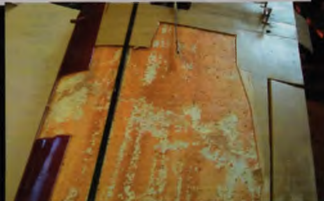
Photo #2: Top of wing after glue has dried and masking tape is removed.
