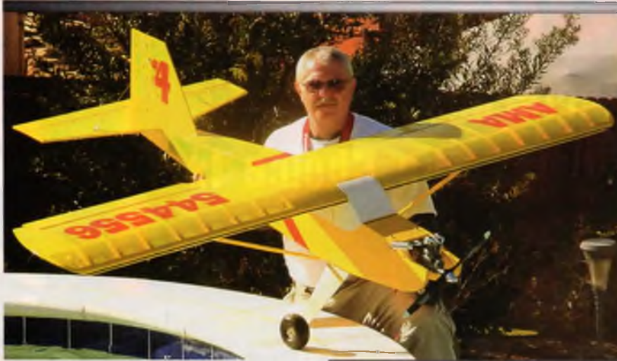
LEFT: Paul Ramirez of Rockwall, Texas, scratch-built this version of the LT-40. It's 20% larger and is powered by a Saito .91. Paul is returning to this great hobby after a 3-year lapse! Can you say LT-40 on Steroids?
