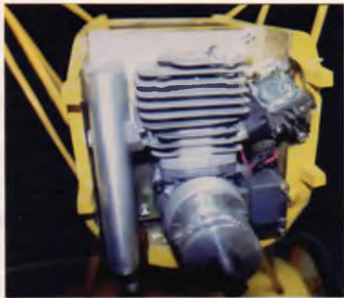
The G-45 with custom Bisson muffler was a tight fit. Cooling air exits through gaps in the top hatches.
