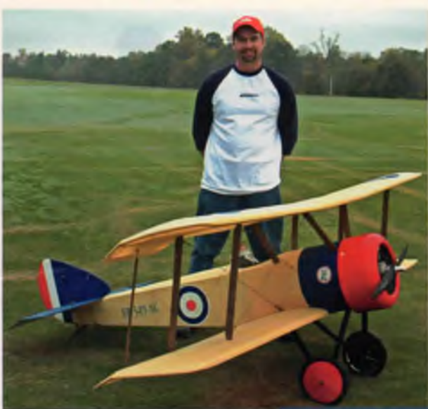
ABOVE: Mike Bost, Rockwell, NC, stands behind his dad's 1/3 scale Balsa USA Sopwith Pup. The Pup is covered with Solartex, weighs approx. 29 lbs. and is powered with a Saito 325 five-cylinder radial. Mike flew the big Pup very realistically.
