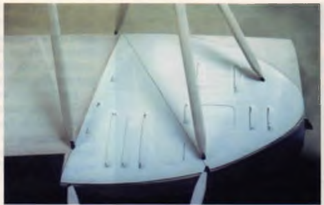
The two-piece fiberglass fuselage cheeks must be lightly sanded with 220 grit sandpaper (in preparation of paint) and holes need to be drilled for the cabane struts and landing gear.
