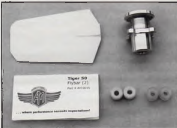
Optional parts from Audacity: 3D paddles and flybar, a fan hub for the O.S. 50 Hyper, and hard and even harder dampers.
