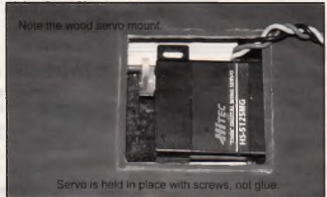
A Hitec HS-125 Wing servo fits easily in the wing bays of the Nova. This is the flap installation and the ailerons used HS-56HB servos.
