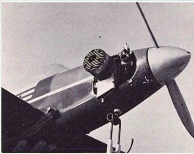
Upper left: View of engine installation. Note Johnson throttle installed on S.T. 60. Above: View of center section of wing showing installation of Orbit Proportional servo and linkage to ailerons. Left: Author and original prototype. Below: Full view of red, white, and blue Patriot.
