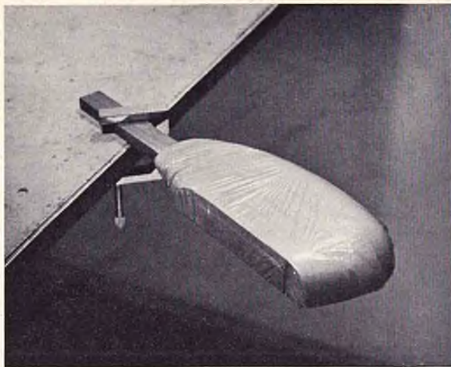
STEP 1. Original male wheel pant form mounted on supporting stick and covered with Saran Wrap. Wrinkles will not show in finished molded part.
