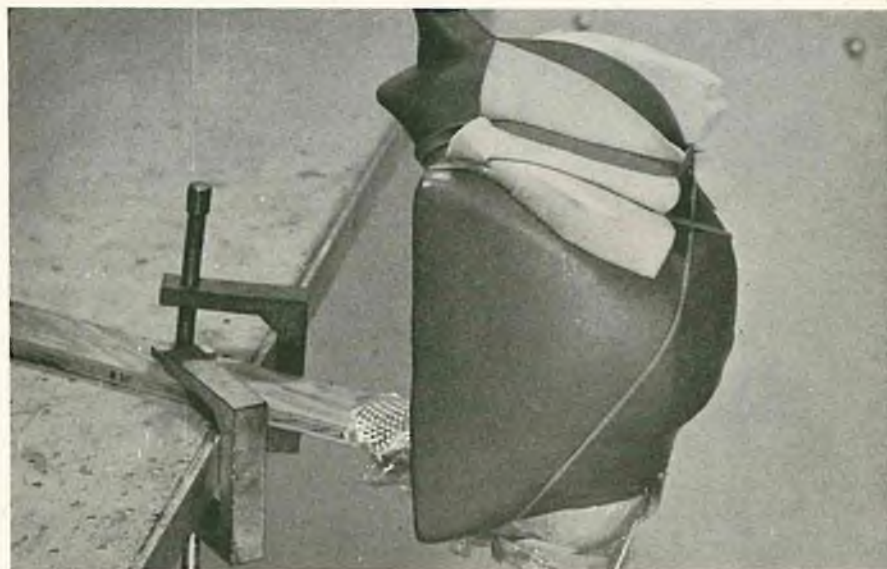
Balloon over form with sponge used to apply pressure on concave sections while glue cures.
