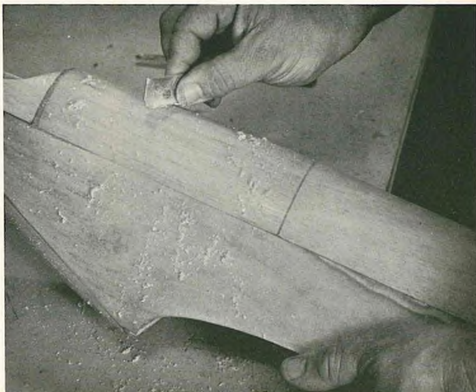
STEP 3. An Enders Speed Blade is used to scrape the hardened glue to a smooth, even surface.
