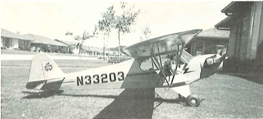
1ST PLACE: C.J. Viosca, 3450 Salisbury Drive, Dallas Texas 75229. Piper J-3 from a Sig Mfg. Co. kit. MRC F-700 Radio, O.S. Max H40P engine. Weight 6½ lbs. Totally scale.
