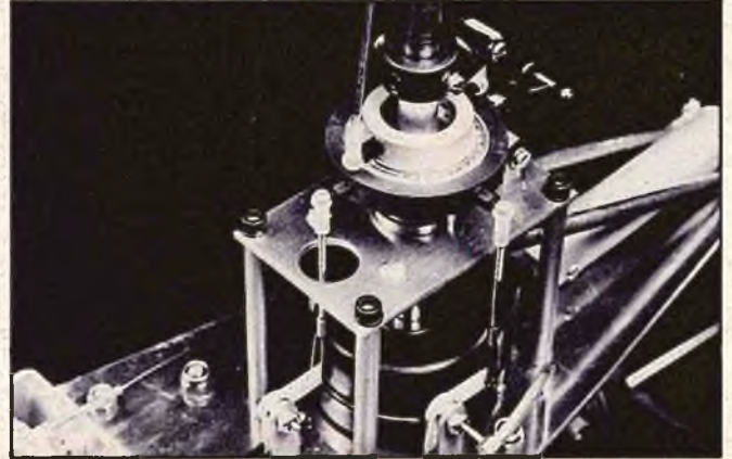
Bellcranks connected to swashplate.
