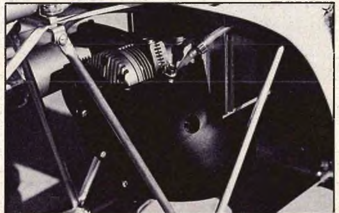
LEFT: Perry Air Filter installed on K & B .61. Slotted extension soldered to needle valve with heat shrink guide for screwdriver adjust. ABOVE: Plastic cooling shroud in place.
