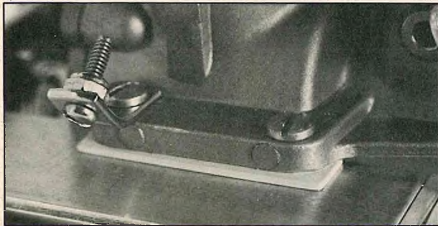
ABOVE: The K & B .61 installed on frame with belt in place. Belt should deflect 1/16" with 1 lb. pressure for proper tension. RIGHT: Cooling fan is installed.
