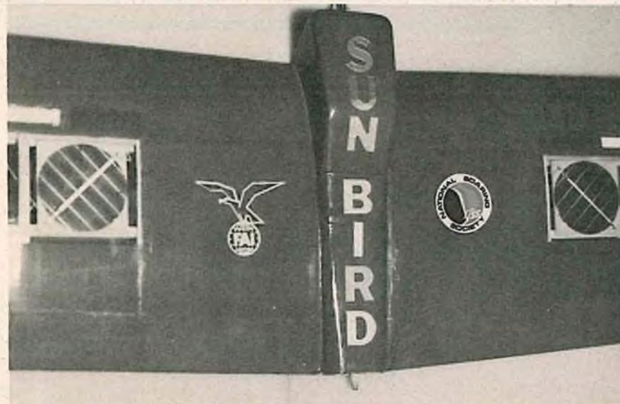
ABOVE: View of radio compartment, showing installation. The little round item next to the radio switch in front is a capacitor added to the receiver connector. The long wires to and from the ammeter introduced too much noise, so an additional filter was added. Note spoiler servo installation in wing. BELOW: Top view of the wing center section with hatch cover enclosing spoiler servo compartment.
