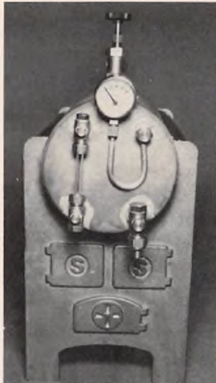
The boiler showing water gauge, check valve and pressure gauge. The tap on top is the steam take-off valve, masked by the safety valve.
