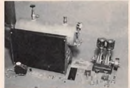
The Double 10 engine and boiler mounted "dry", to see what it looks like. Note the size by comparison with the servo bottom left.
