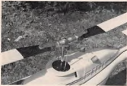
New head on D.C.'s Jet Ranger where the mixing levers have been eliminated for a cleaner more scale appearance.
