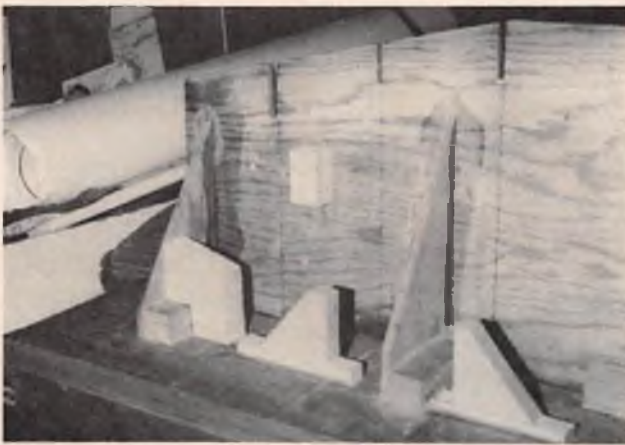
Close up of hull jig showing blocks to secure hull frames.
