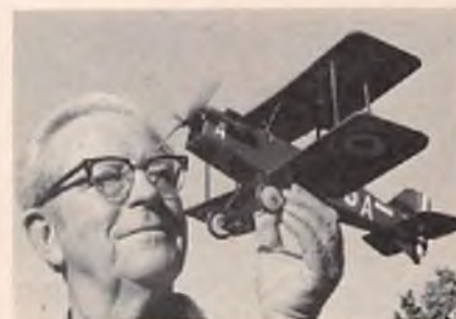
It's the peanutiest! Willard's .020 powered R/C Peanut Scale SE-5 is one of the world's smallest R/C planes.
