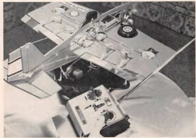
The R/C Flight Simulator at half throttle, full right aileron and full up elevator. A small light on each wing tip blinks on and off to let you know it's ready for action.
