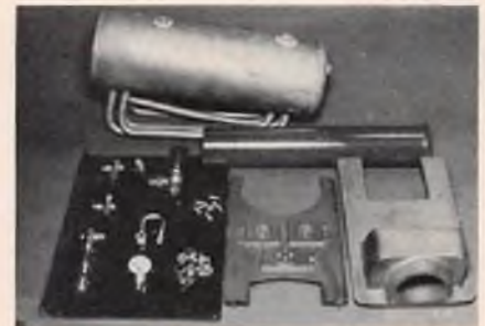
The boiler parts, including the long, cast-iron chimney.
