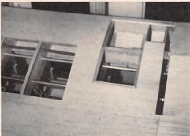
Shows servo compartment and slot for engine pylon.
