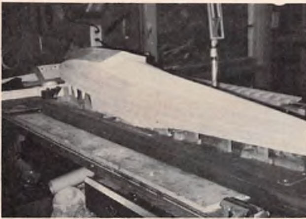
Side and bottom sheeting complete. Set aside over night to dry prior to applying fiberglass cloth and resin.
