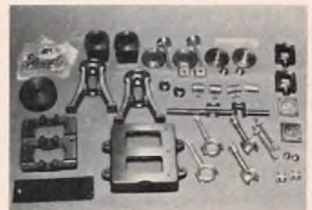
Layout of the parts of the Double 10 engine, less reversing gear. It looks very impressive, but goes together like a construction set.
