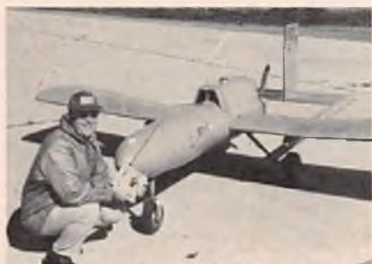
Ken Willard was test pilot for Lockheed's RTV-1 program. Vehicle shown weighed 340 pounds, had 12' wingspan, and was powered by a 24 H.P. snowmobile engine.
