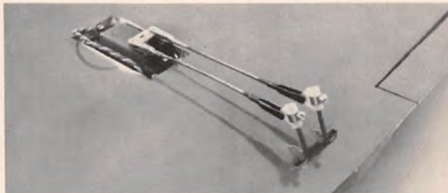
A top view of a low wing with differential horns installed on strip ailerons. The more the horns are bent, the greater the differential.
