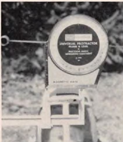
Close-up shot showing how to properly use 4" Angleometer and X-Acto clamp.
