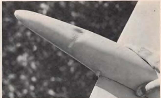
Bill Watson's plastic fuse Cheetah after a very solid centerpunch. The dent could be easily popped back out.
