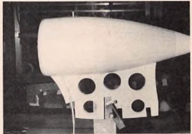
View of nacelle and pylon after strip planking. Not difficult but takes time.
