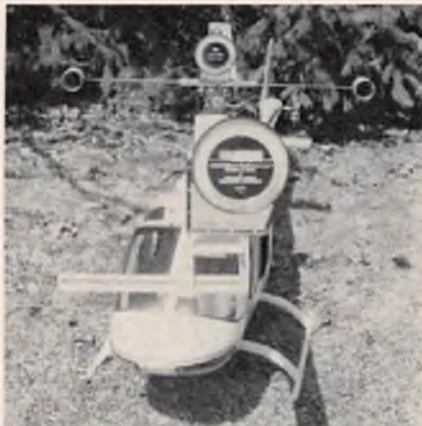
Both 3" and 4" Angleometers as used to check and set pitch.
