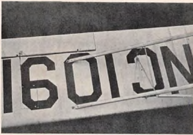
Wing strut attachment to wing – note servo access hatch.
