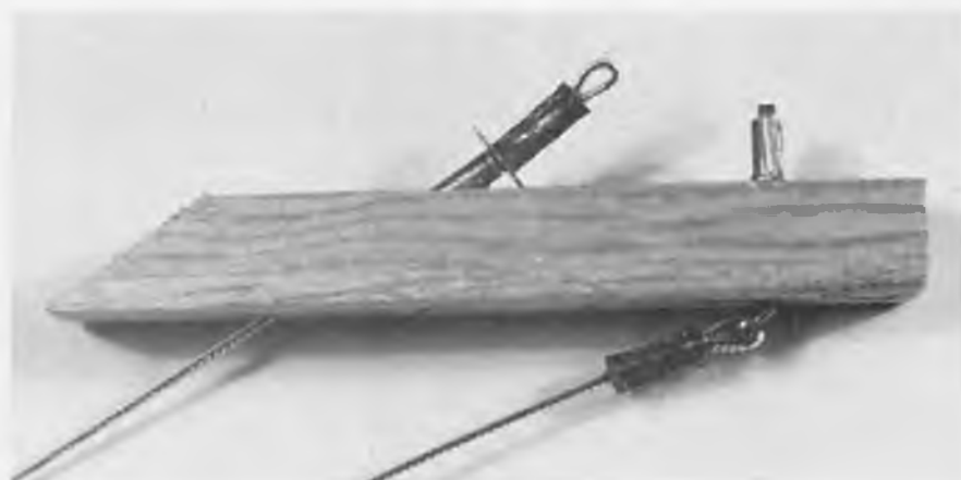
Flying wire anchor on left side uses no cotter key. Wire is brought through brass tube and secured on far side with A-3 sleeve. Use washer between sleeve and tubing.
