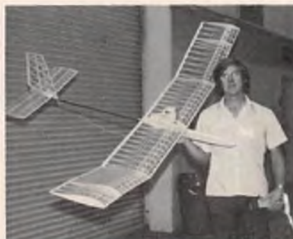
Bill Watson shows off his construction on his indoor electric. He changes power pod and it becomes a CO 2 powered glider.
