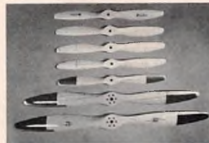
(10) Top to bottom. Out of the box. Shaped, sanded and balanced. Metal leading edges and canvas tips. Laminations drawn in. Canvas painted. Gold leading edges and coat of clear K & B clear epoxy paint. Decal and two more coats clear.
