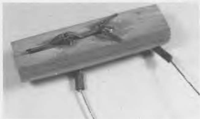
Typical cotter key flying wire anchor through wing spar. Note way the legs are bent over brass tubing. A tight bend is essential for a successful installation.
