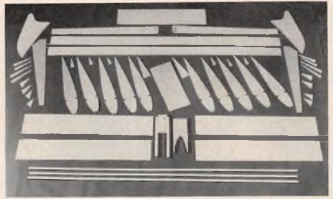
Note that the only area of moderate complexity is cutting out ribs in pre-assembly preparation.
