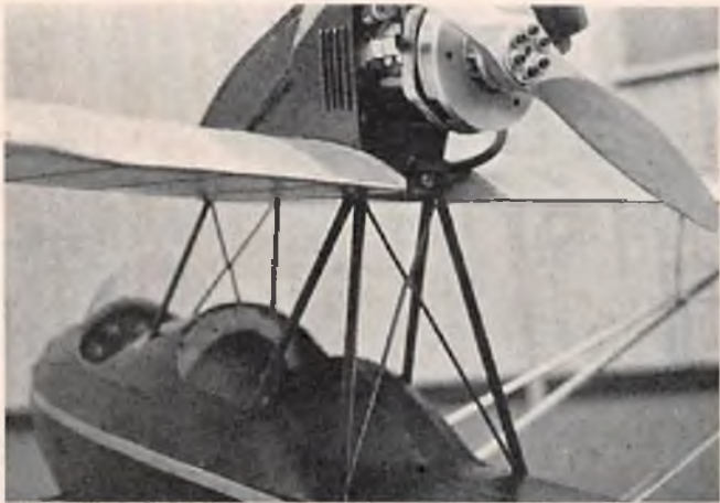
Rear view of cabane struts.
