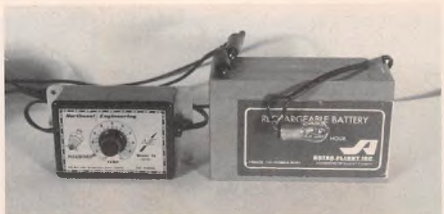
Testing the driver, using the automotive bulb furnished for a load. Saves plug if problem exists.
