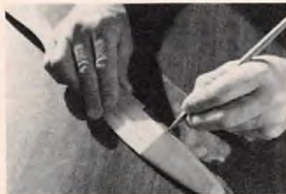
(7) Drawing in divisions in metal leading edges and applying dots to simulate screws.
