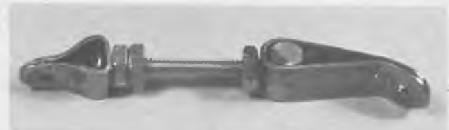
Simple to build turnbuckle will do the job. Easy on the pocketbook too. Would look great on most vintage aircraft.
