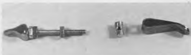
Turnbuckle parts spread out. Flying wire fitting is bent around head of machine screw. Anchor fitting is bent around 3/16" dia. music wire. No problem with special threads in this design.
