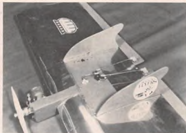
Completed "Silver Fox" with Du-Bro mixer. Works well but has some drawbacks. Fuel tank mounted in leading edge of wing.
