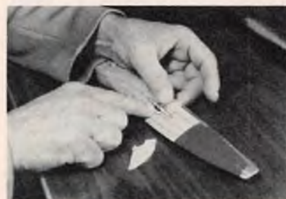
(9) Applying manufacturer's brand name decals.
