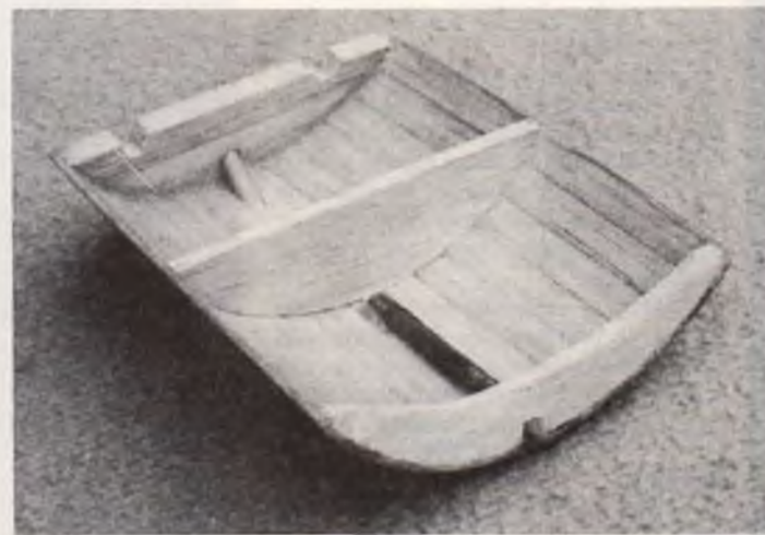
Underside of tank hatch. Hatch was planked with strips.
