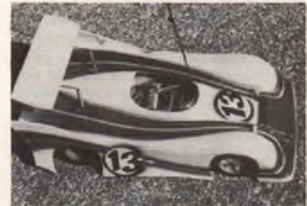
Jianas' RC12E car was built by Mike Lavacot, featuring Reedy Modified horsepower, graphite chassis, Novak servos and receiver.
