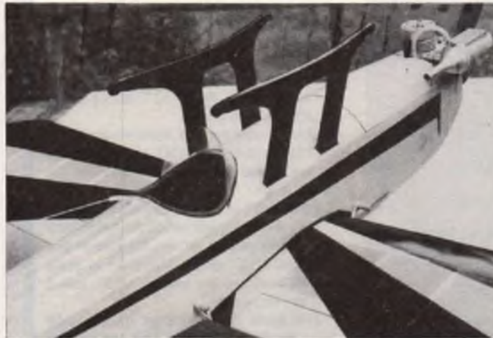
Top wing removed to show cabane struts.
