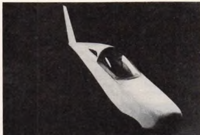
Fuselage sanded to shape.
