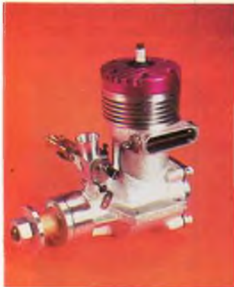
1919 Lee .45; handmade engine designed expressly for R/C.
