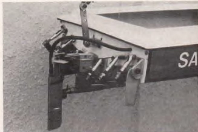
Starboard view of hardware showing anti-spin fin.
