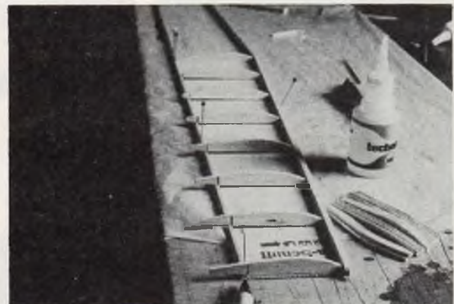
Rib length is marked for tapered ribs.
