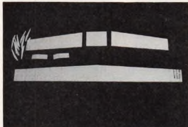
Wing bottom sheeting and ribs.
