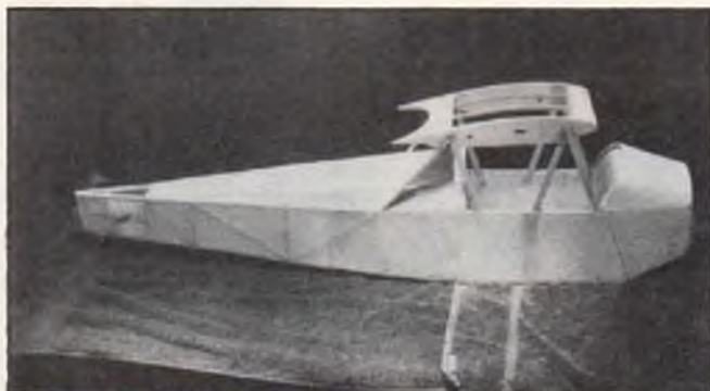
Cover all areas before shrinking to avoid any warps and twists in framework.
