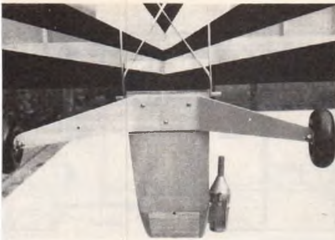
Bottom side showing landing gear installation. L/G bolted to 1/4" ply plate.
