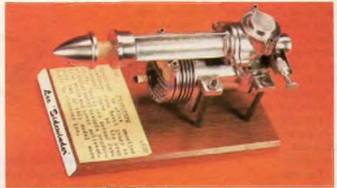
1952 Lee Sidewinder .32; horizontal piston engine.
