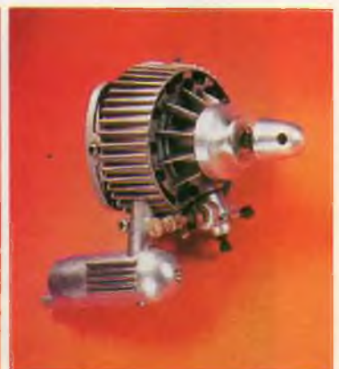
1971 O.S. Wankel; 1st and only Wankel type model engine.
