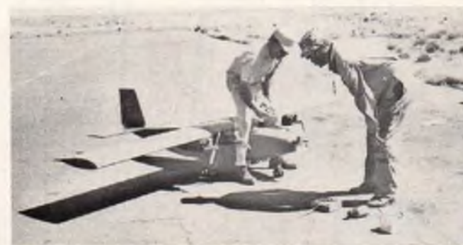
Dan Parsons (right) and unidentified assistant prepare five engined (OS Max .80's) drone for flight back in 1967. Model was part of a research project in New Mexico at that time. Look at that flying field, if you couldn't get on that runway, you shouldn't fly! More in text.
