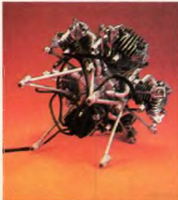
1946 Morton M-5; rear view, 5 cylinder 4 stroke cycle.
