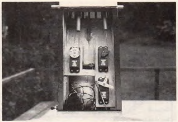
Bottom wing removed showing ample room for servo installation and access to linkage.
