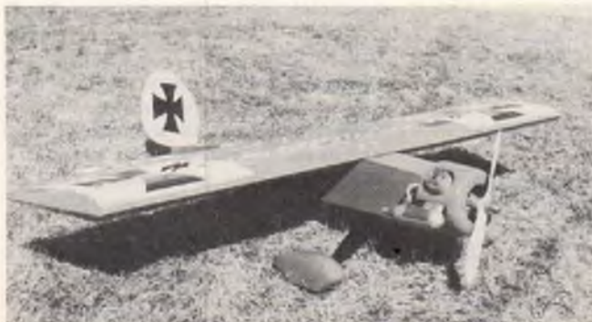
Modified Sweet Stick by Bob Land. K & B .61 cowl, wheel pants, bolted wings. Slick.
