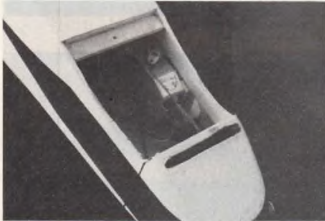
Throttle servo is mounted with foam mounting tape.
