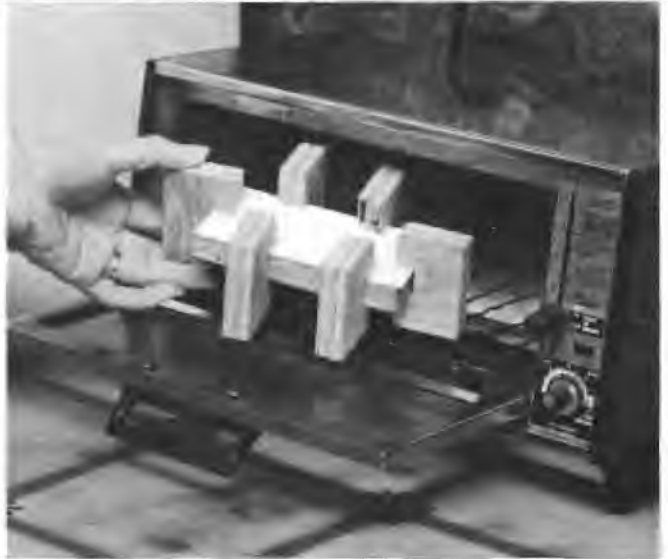
Photo 4. The whole shooting match going into our toaster oven to heat up the plastic. The form should be heated until the plastic just starts to sag.
