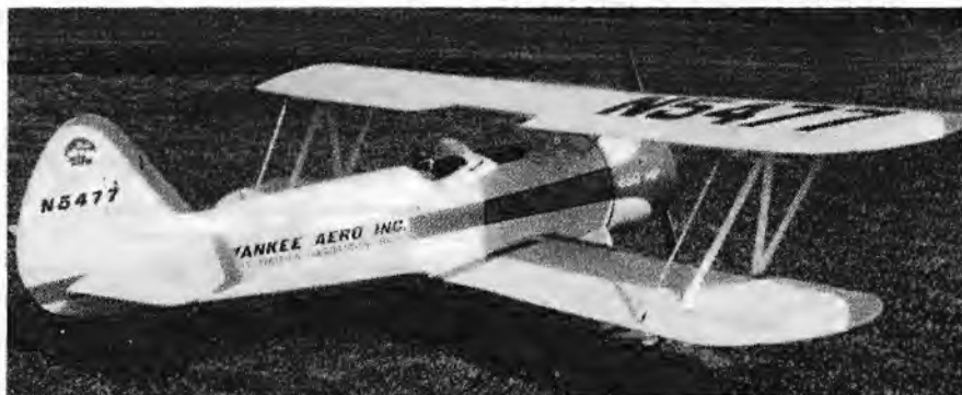
Photo of Bob Wallace's large Stearman powered with a Kawasaki engine. Bob uses the Don Harris smoke system which works very well. Model weighs in dry at 28½ lbs.
