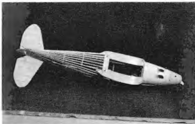
Bottom view of fuselage. Note engine cooling outlets.
