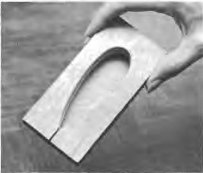
Photo 1. The base block that was cut out of 3/4 ply on a band saw.
