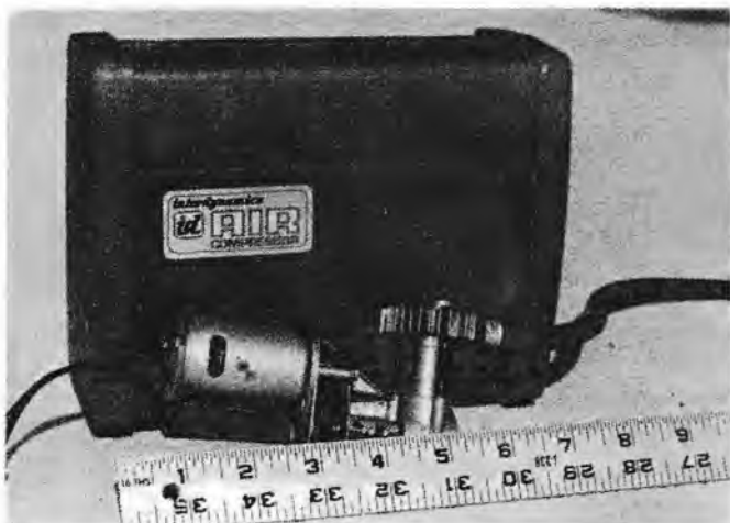
Twelve volt compressors sold to pump up auto tires work even better putting air in your retract system. Throw away the plastic case and put it in your flight box.
