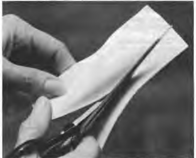
Photo 6. All that is left to do is to trim the plastic with scissors, make 17 more and jet glue them into position on the cowling. One last coat of resin over the entire cowling will smooth out all of the surfaces in preparation for painting.
