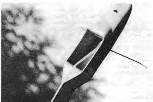
Fuselage top filled in and shaped.
