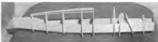
Basic fuselage structure.
