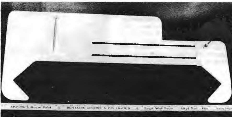
An incidence meter large enough to measure practically anything. Will accept up to 31" chord and up to 6" deep wings and give accurate incidence measurements. More in text.
