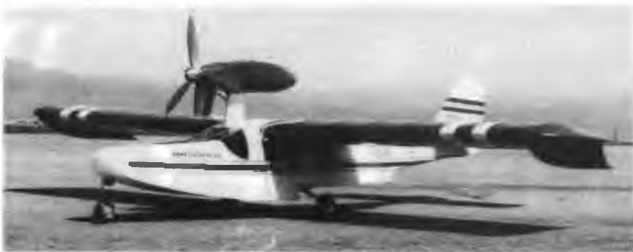
Original Seamaster Sport 40 with short specially bent landing gear.
