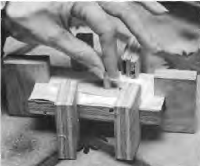
Photo 5. The form being pushed into the base to form the blister.
