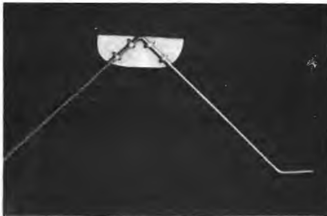
Landing gear wire is sewn and epoxied to Item 8.
