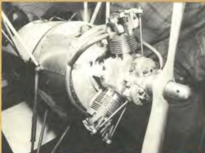
Forest Edwards' first radial engine was this 3 cylinder four stroker shown installed in a 9 lb. Gere Sport.
