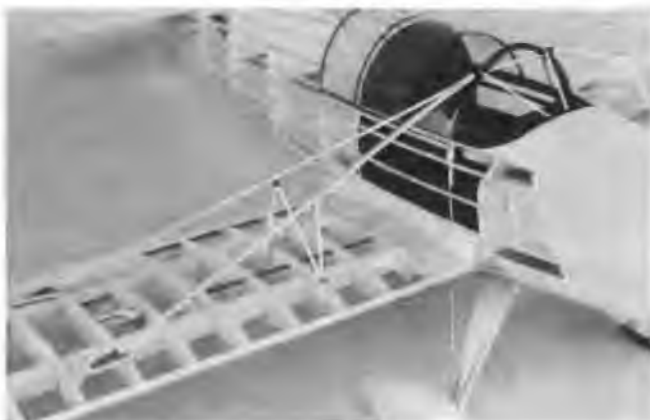
Strut details. Note fillet construction.
