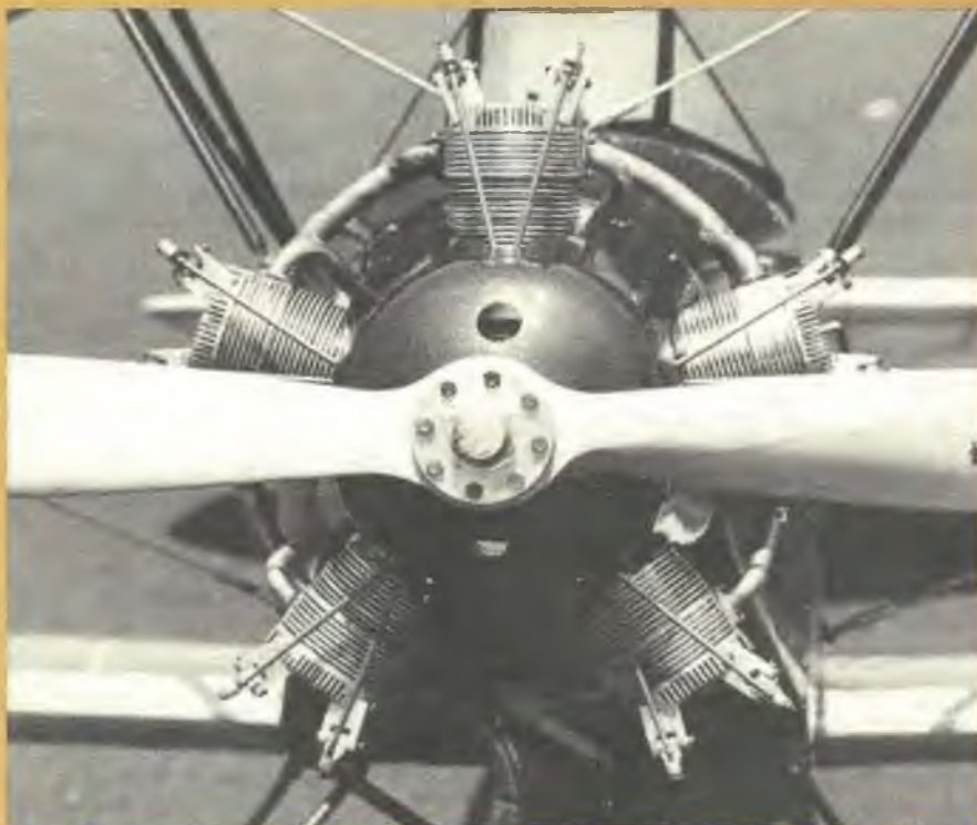
Front view of Forest Edwards' 5 cylinder four stroke engine mounted in a Quarter Scale Concept Fleet. Tichenor photo.
