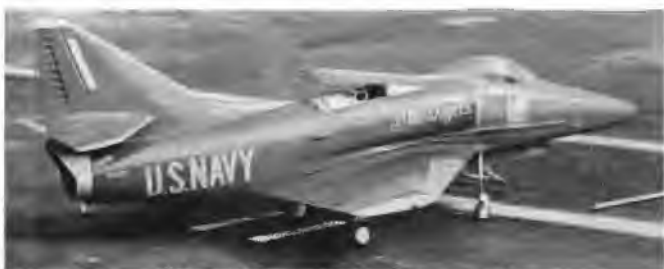
Art Arrow's A-4 Skyhawk at the Tangerine, ready for engine start. Note the hand pump connected to retract valve. Good for small air tanks but flight box compressor is easier.
